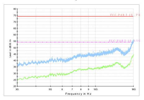
Fig.5. Radiated emission: Channel 0, 3 GHz - 18 GHz
