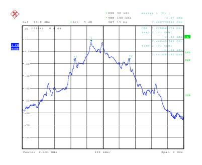
Fig.1. Occupied Bandwidth: Channel39
