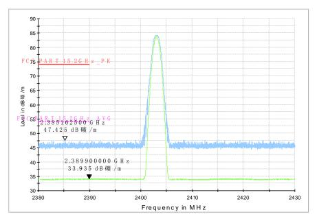
Fig.12. Radiated emission (Power): Low Channel
