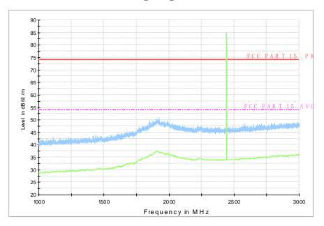
Fig.7. Radiated emission: Channel 39, 1 GHz - 3 GHz
