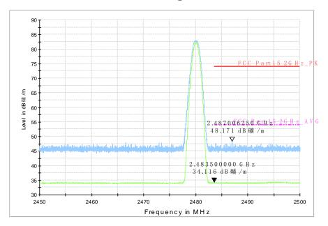
Fig.13. Radiated emission (Power): High Channel
