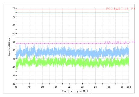
Fig.9. Radiated emission: Channel 39, 18 GHz ~ 26 GHz
