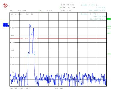
Fig.2. pulse width: Channel 39
