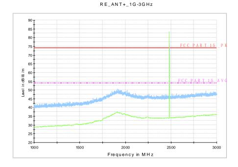
Fig.10. Radiated emission: Channel 78, 1 GHz - 3 GHz
