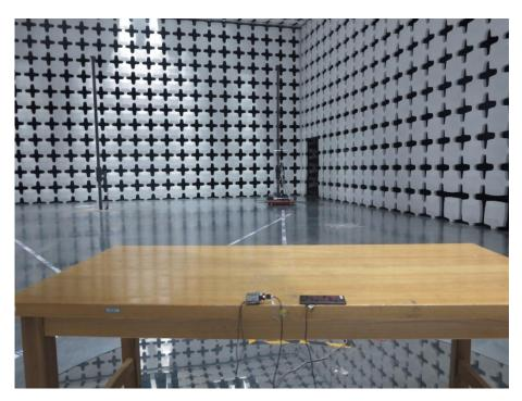
Picture C-6: Radiated emission (PART15B)
