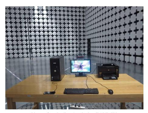
Picture C-7: Radiated emission (PART15B)
