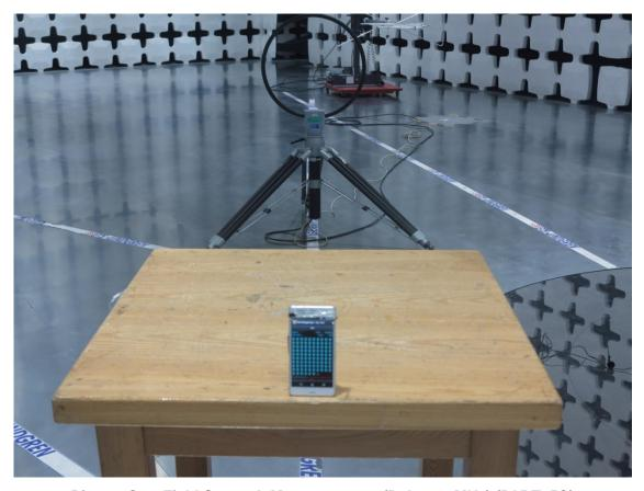
Picture C-1: Field Strength Measurements (Below 30MHz) (PART15C)
