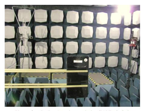
Picture C-4: Radiated spurious emission (PART22/24/27)
