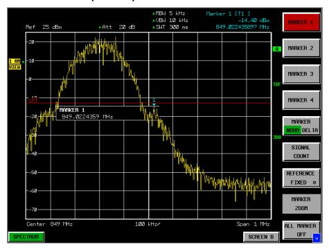
GPRS 850 LOW BAND EDGE BLOCK-A (GSM850)-Channel 128
