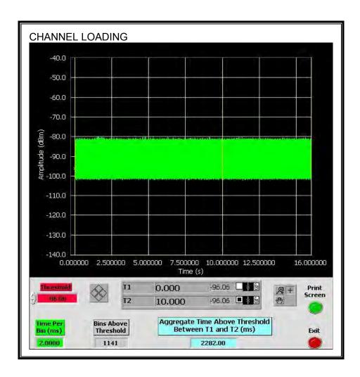
The level of traffic loading on the channel by the EUT is 22.82%
