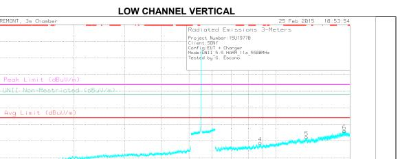
Note: Emission was scanned up to 40GHz; No emissions were detected above the noise floor which was at least 20dB below the specification limit.
