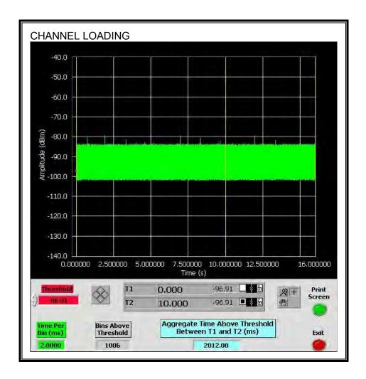
The level of traffic loading on the channel by the EUT is 20.12%
