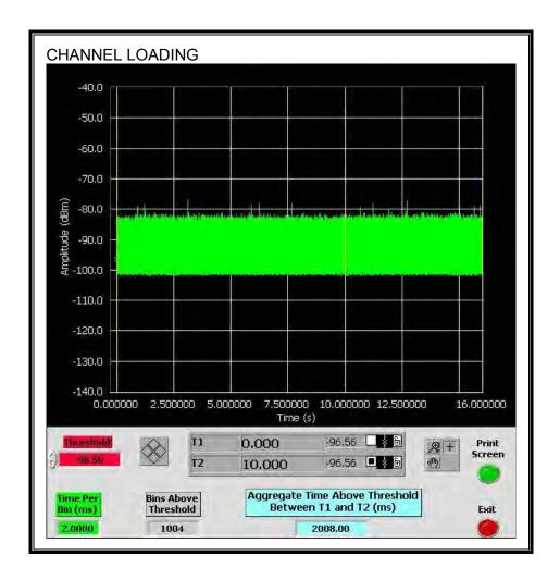
The level of traffic loading on the channel by the EUT is 20.08%
