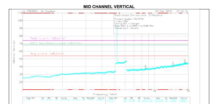
Note: Emission was scanned up to 40GHz; No emissions were detected above the noise floor which was at least 20dB below the specification limit.
