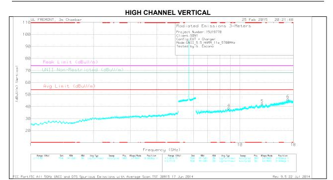
Note: Emission was scanned up to 40GHz; No emissions were detected above the noise floor which was at least 20dB below the specification limit.
