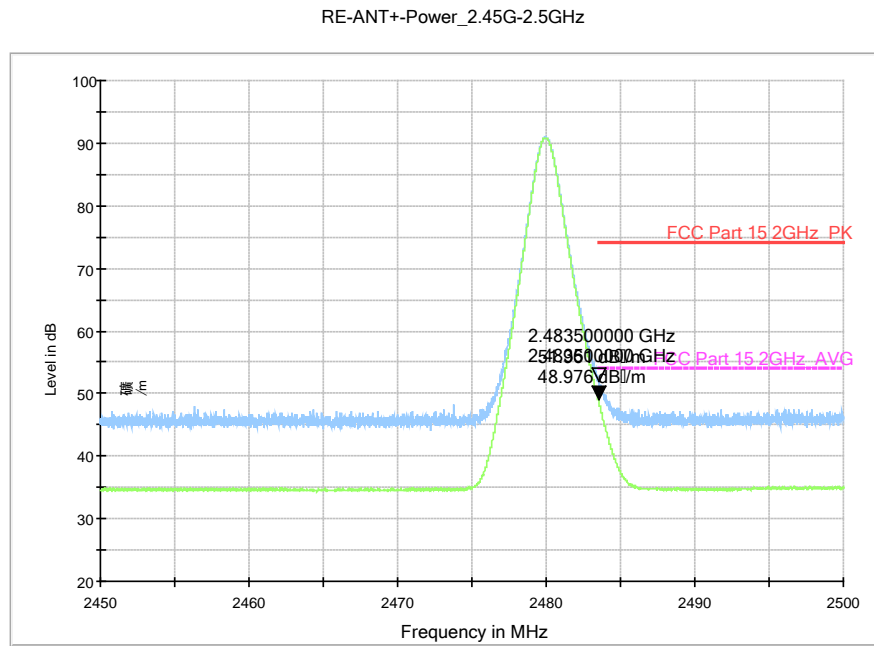
Fig.10 Radiated emission (Power): High Channel
