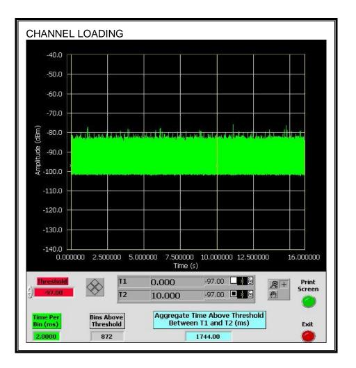
The level of traffic loading on the channel by the EUT is 17.44%
