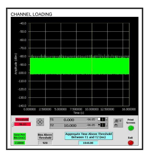
The level of traffic loading on the channel by the EUT is 18.4%
