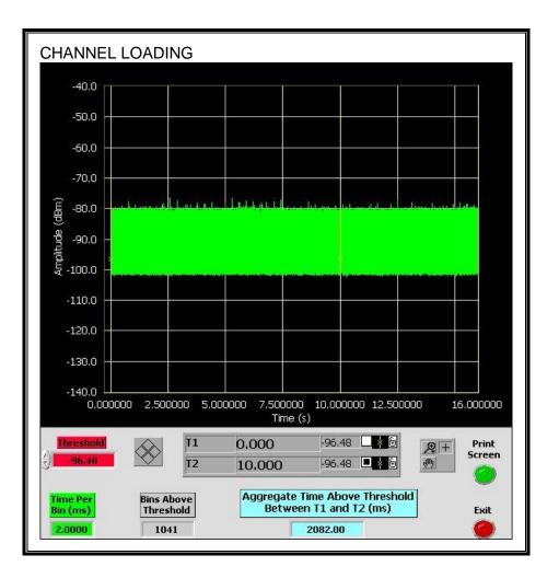
The level of traffic loading on the channel by the EUT is 20.82%
