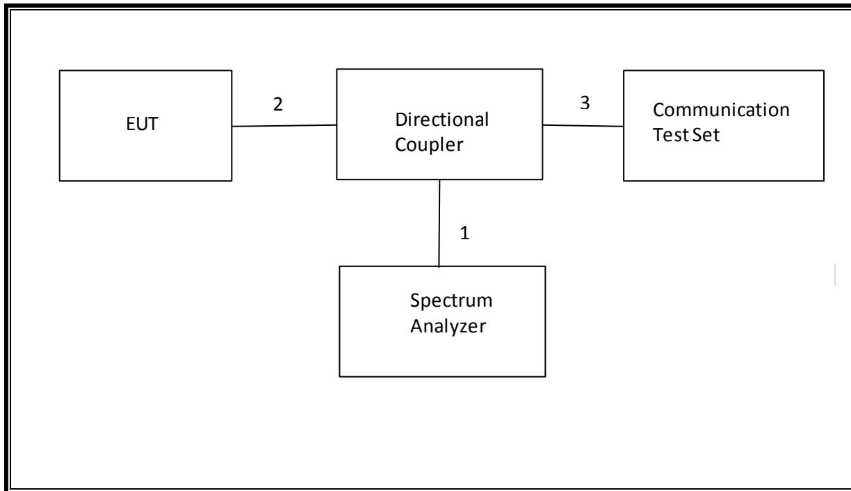
**SETUP DIAGRAM FOR TESTS (RADIATED TEST SETUP)**
