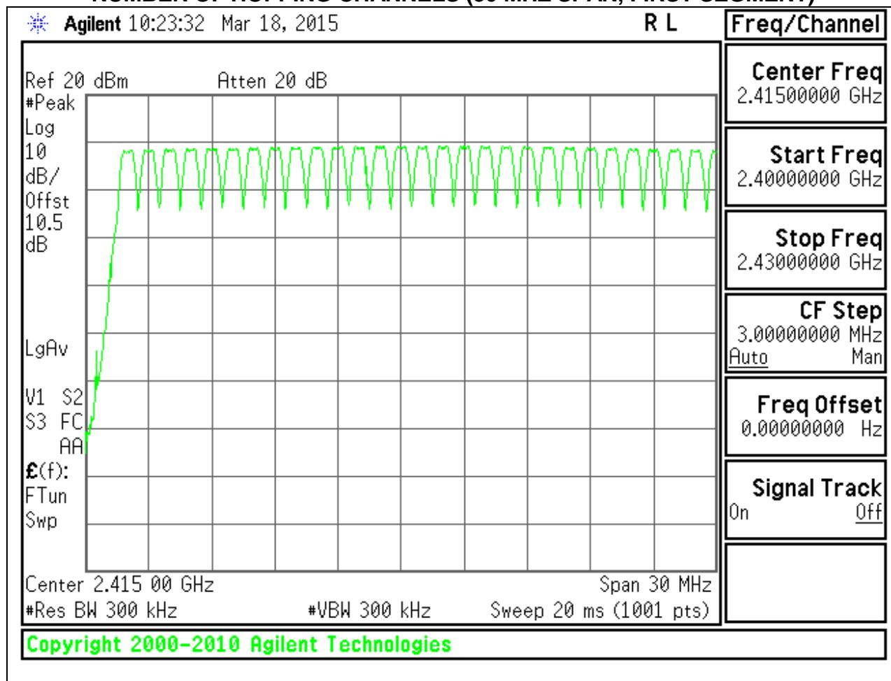
**NUMBER OF HOPPING CHANNELS (30 MHZ SPAN, SECOND SEGMENT)**
