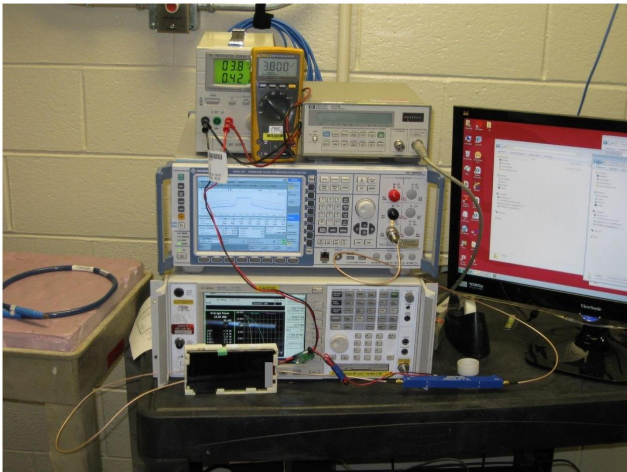
**RADIATED RF MEASUREMENT SETUP FOR PORTABLE CONFIGURATION**
