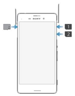
Don't confuse the nano SIM card slot with the memory card slot. Inserting a card in the wrong slot could damage both the card and your device.
