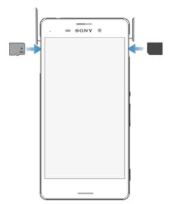
Don't confuse the nano SIM card slot with the memory card slot. Inserting a card in the wrong slot could damage both the card and your device.
