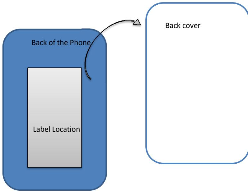
The label is under the back cover and is visible to the users as the users remove the back cover to install the SIM card.
