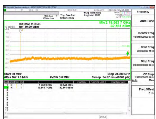
LTE66 20MHz QPSK HIGH Ch RB1-0
