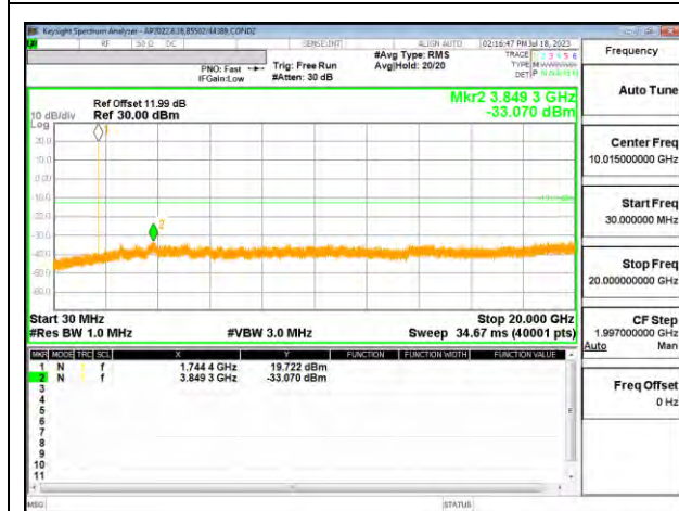
LTE66 3MHz QPSK MID Ch RB1-0
