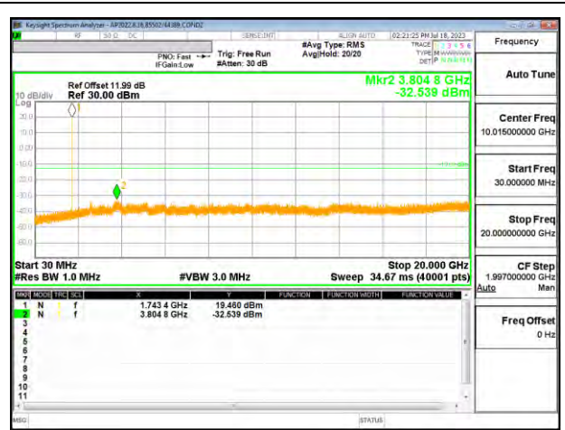
LTE66 5MHz QPSK MID Ch RB1-0
