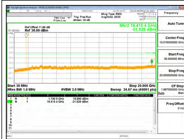
LTE66 10MHz QPSK MID Ch RB1-0
