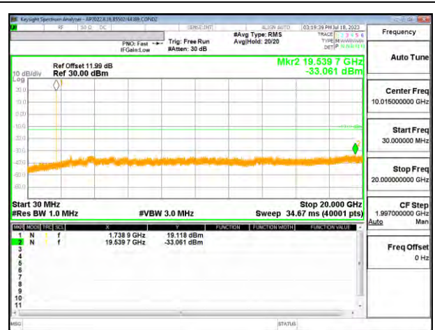
LTE66 15MHz QPSK MID Ch RB1-0
