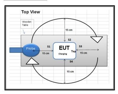
Note: This is a 2D representation of setup. EUT and load are stacked on top of each other.
