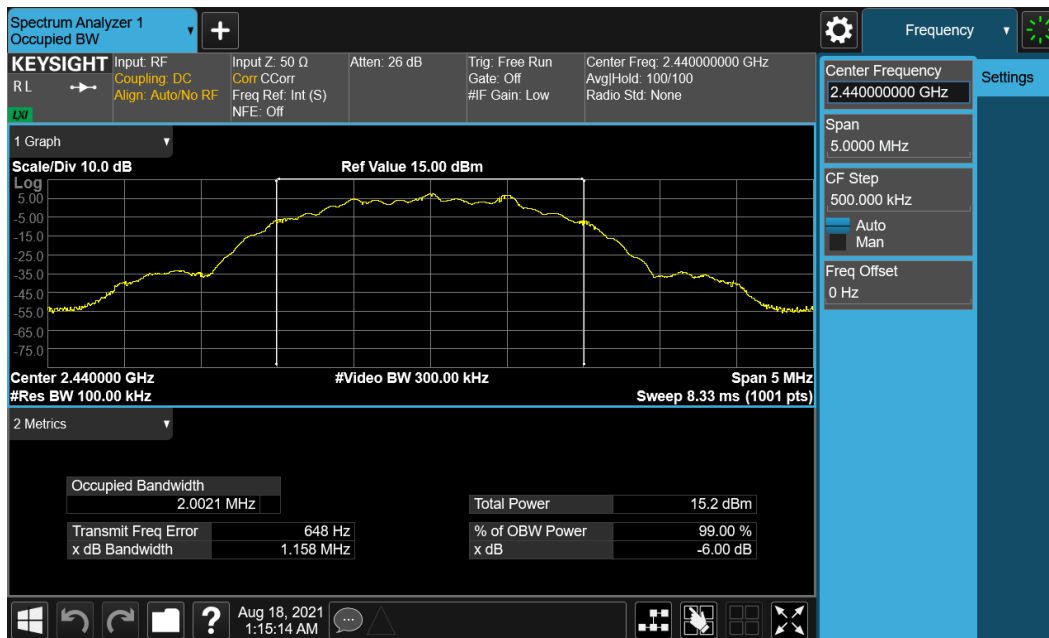
Plot 7-5. 6dB Bandwidth Plot (Bluetooth (LE), 2Mbps – Ch. 19) – Main Antenna
