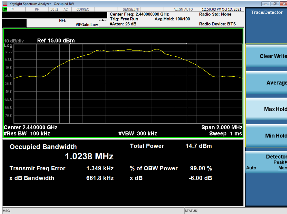
Plot 7-8. 6dB Bandwidth Plot (Bluetooth (LE), 1Mbps – Ch. 19) – Sub Antenna
