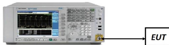
Figure 7-2. Test Instrument & Measurement Setup
