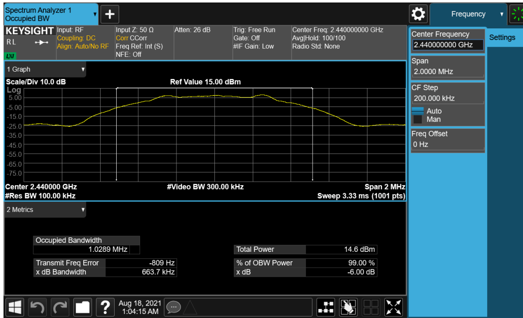
Plot 7-2. 6dB Bandwidth Plot (Bluetooth (LE), 1Mbps – Ch. 19) – Main Antenna
