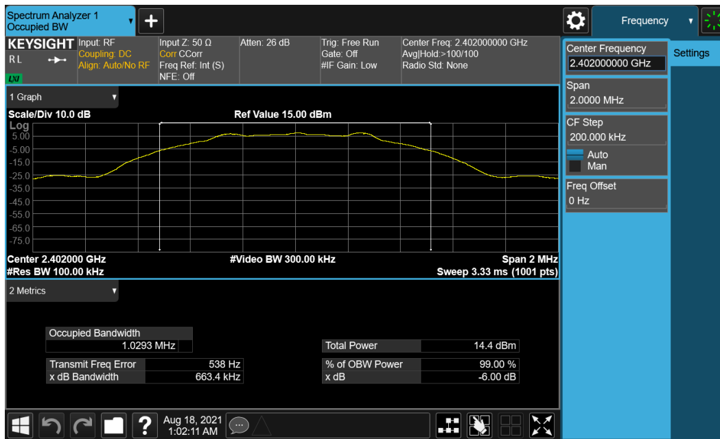
Plot 7-1. 6dB Bandwidth Plot (Bluetooth (LE), 1Mbps – Ch. 0) – Main Antenna
