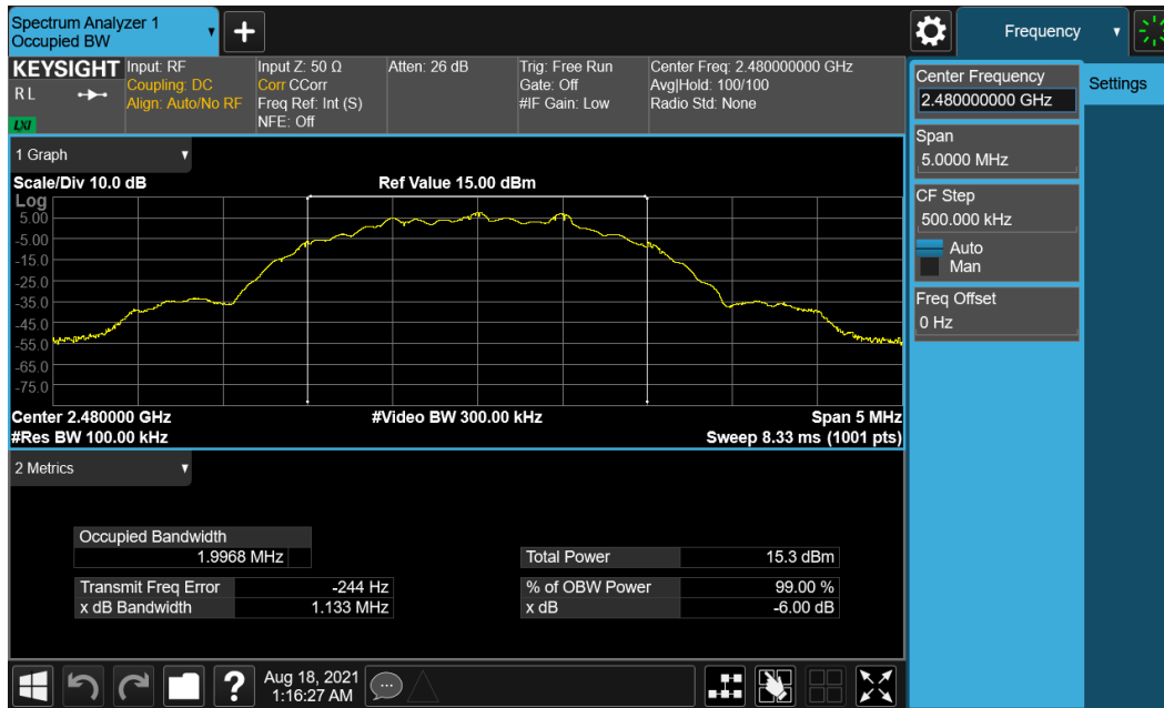
Plot 7-6. 6dB Bandwidth Plot (Blue tooth (LE), 2Mbps - Ch. 39) - Main Antenna
