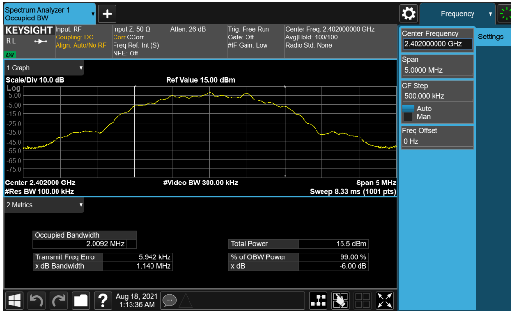
Plot 7-4. 6dB Bandwidth Plot (Bluetooth (LE), 2Mbps – Ch. 0) – Main Antenna
