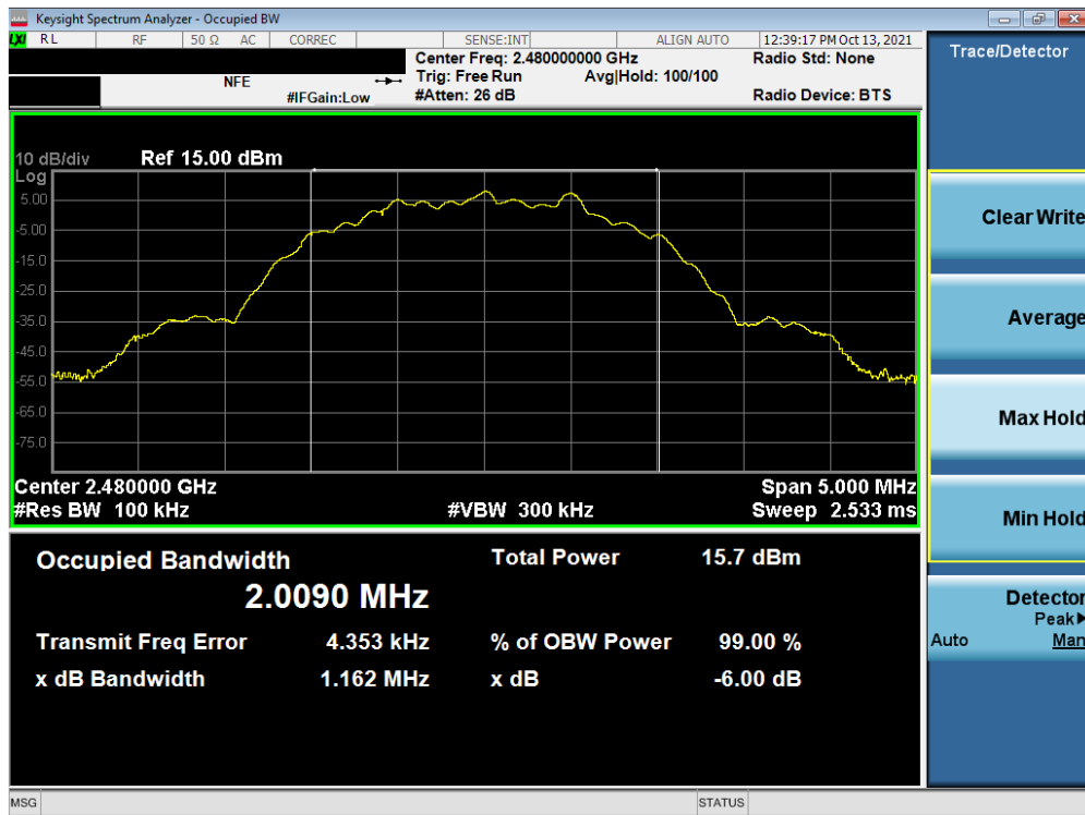
Plot 7-12. 6dB Bandwidth Plot (Bluetooth (LE), 2Mbps – Ch. 39) – Sub Antenna
