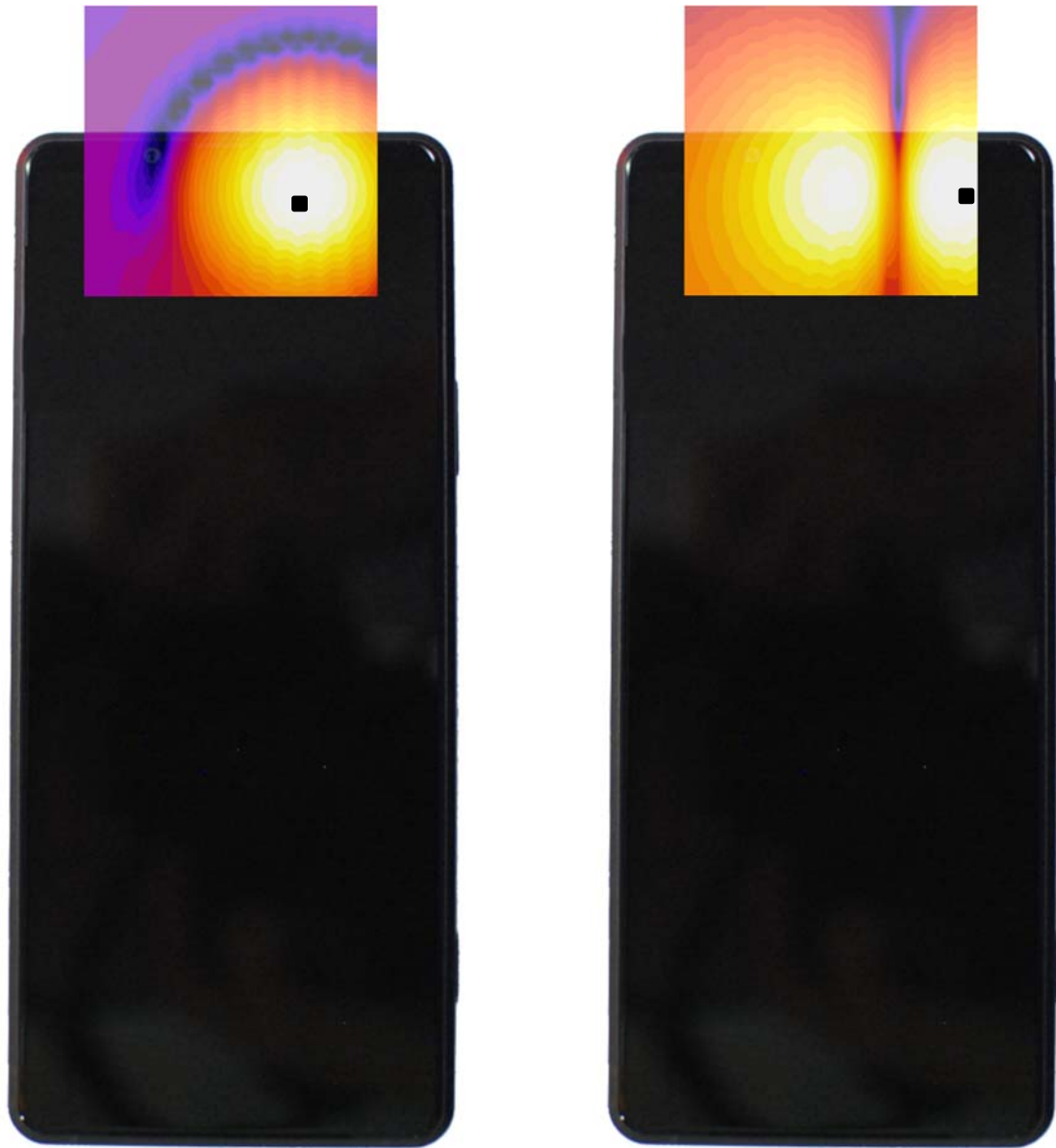
Figure 15-3 T-Coil Scan Overlay Magnetic Field Distributions
