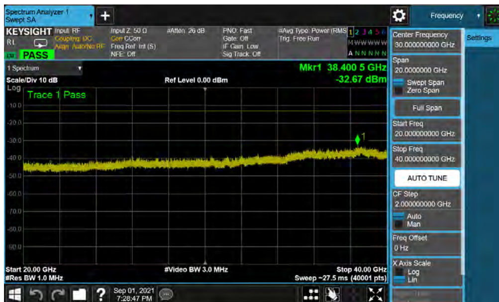
Plot 7-33. Conducted Spurious Plot (NR Band n77 - 100MHz QPSK - RB Size 1, RB Offset 0 - Mid Channel )
