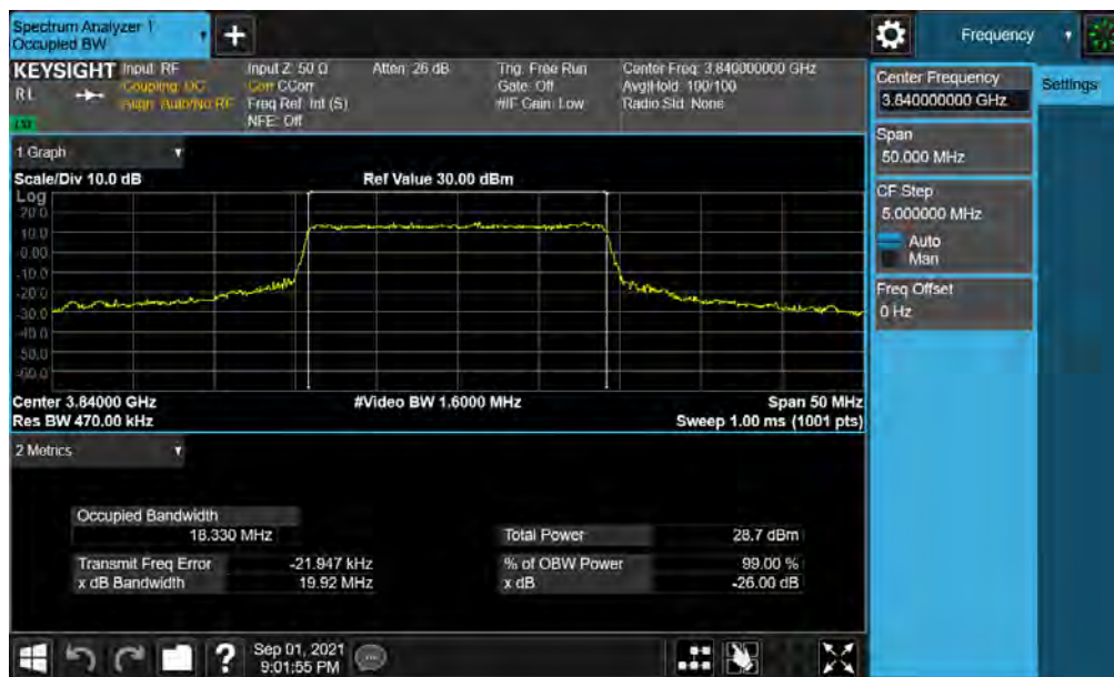
Plot 7-26. Occupied Bandwidth Plot (NR Band n77 - 20MHz QPSK - Full RB )
