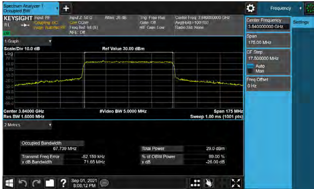
Plot 7-11. Occupied Bandwidth Plot (NR Band n77 - 70MHz QPSK - Full RB )
