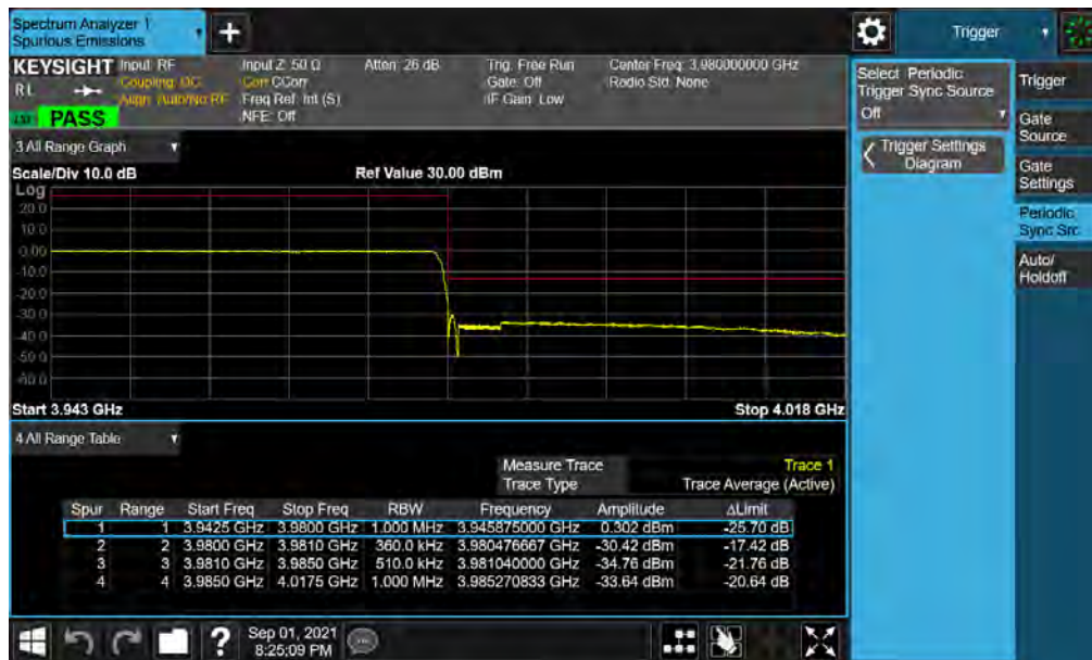
Plot 7-46. Upper ACP Plot (NR Band n77 - 60MHz CP-OFDM-QPSK – Full RB )
