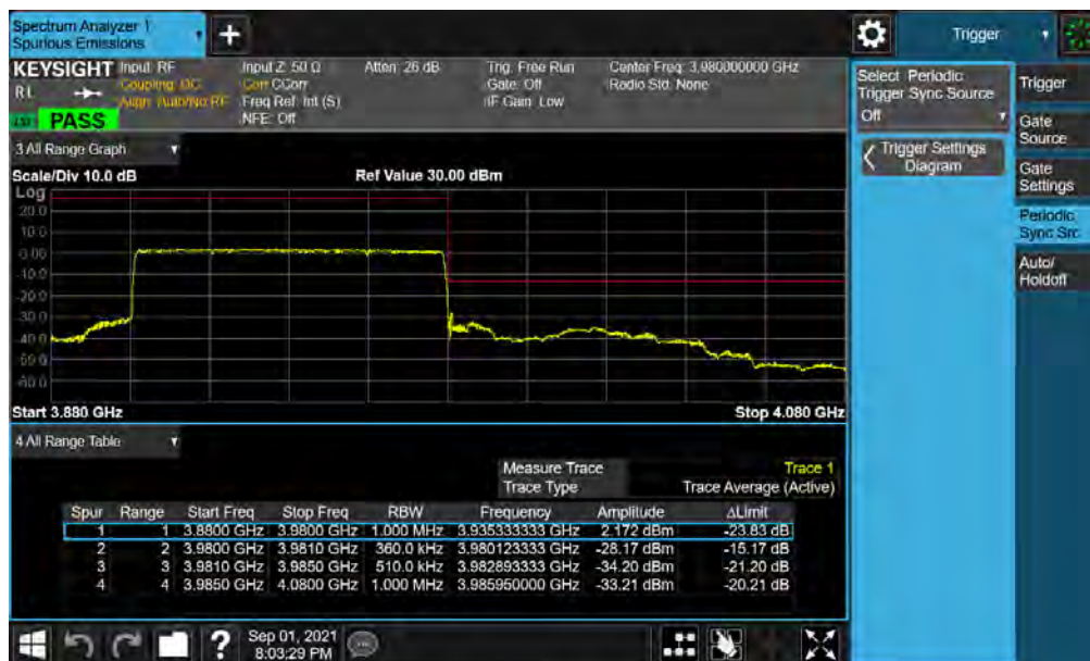
Plot 7-42. Upper ACP Plot (NR Band n77 - 80MHz CP-OFDM-QPSK - Full RB)
