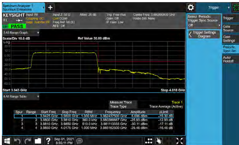
Plot 7-52. Upper ACP Plot (NR Band n77 - 30MHz CP-OFDM-QPSK - Full RB)
