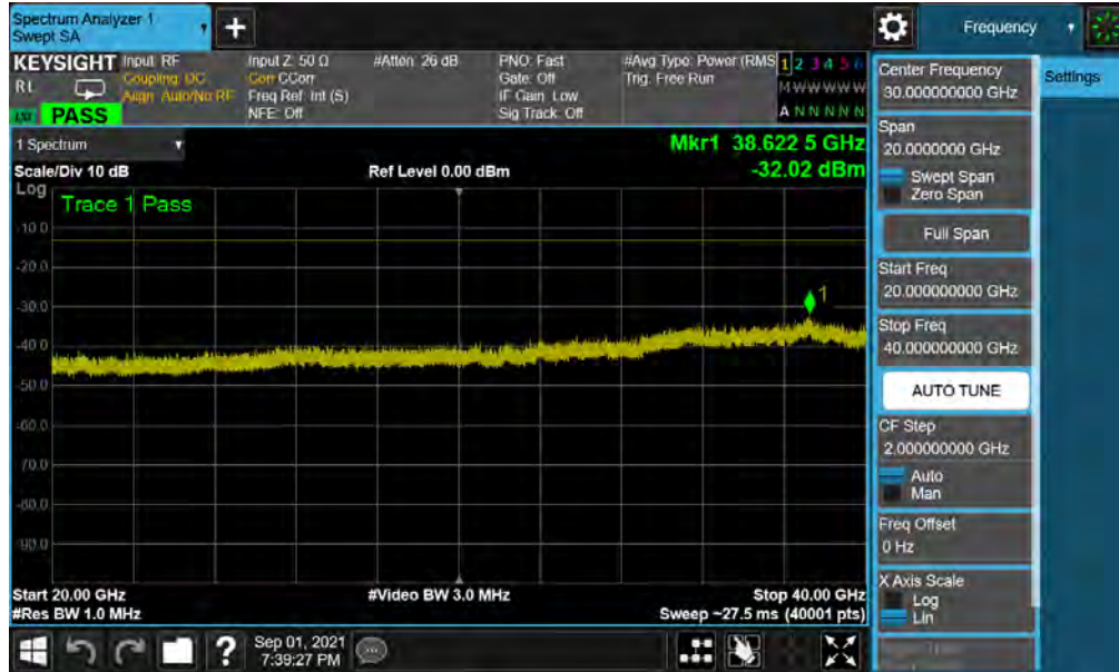
Plot 7-36. Conducted Spurious Plot (NR Band n77 - 100MHz QPSK - RB Size 1, RB Offset 0 - High Channel)
