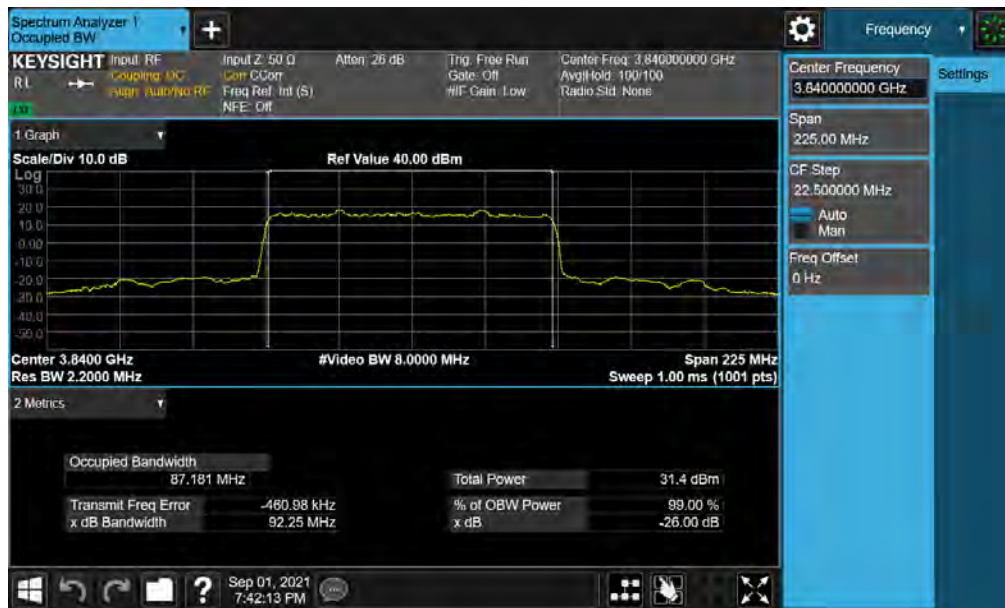
Plot 7-4. Occupied Bandwidth Plot (NR Band n77 - 90MHz \pi/2 BPSK - Full RB )
