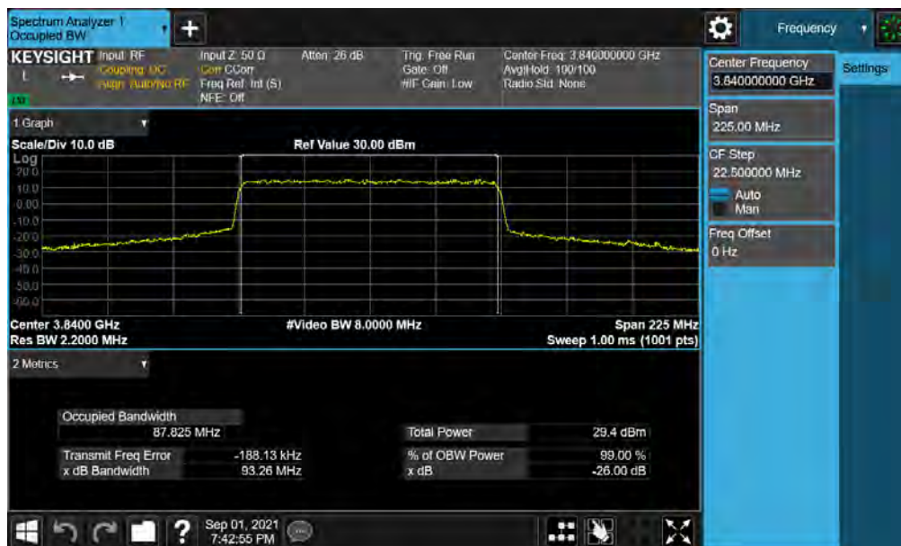
Plot 7-6. Occupied Bandwidth Plot (NR Band n77 - 90MHz 16-QAM - Full RB )
