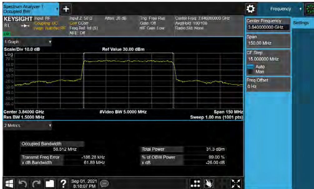
Plot 7-13. Occupied Bandwidth Plot (NR Band n77 - 60MHz \pi/2 BPSK - Full RB )
