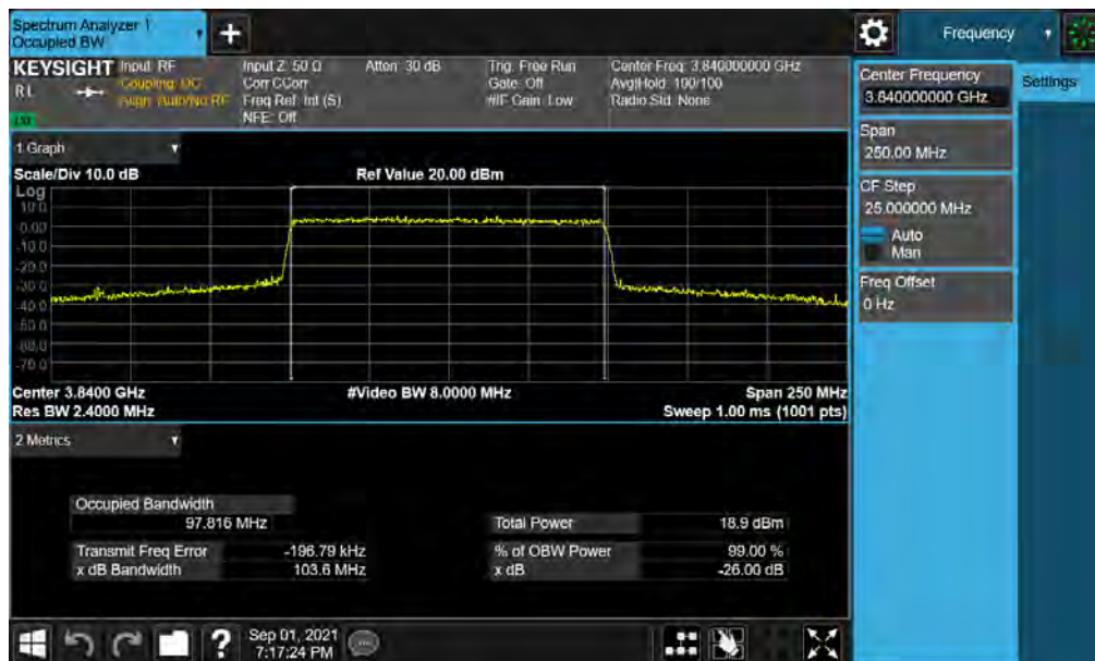
Plot 7-2. Occupied Bandwidth Plot (NR Band n77 - 100MHz QPSK - Full RB )
