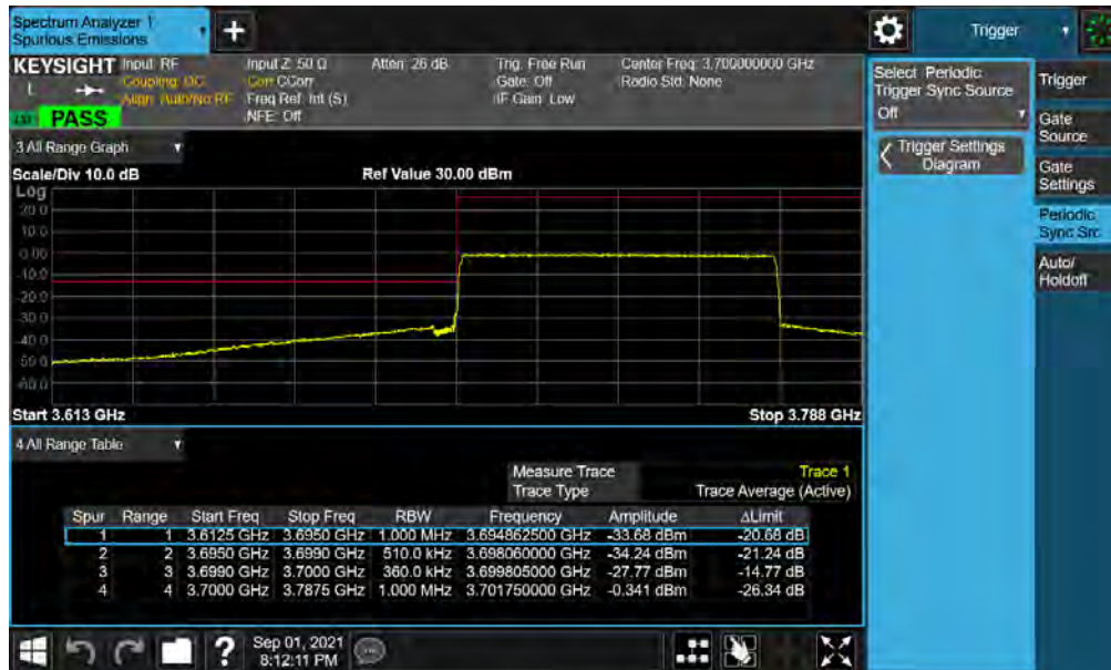
Plot 7-43. Lower ACP Plot (NR Band n77 - 70MHz CP-OFDM-QPSK - Full RB)
