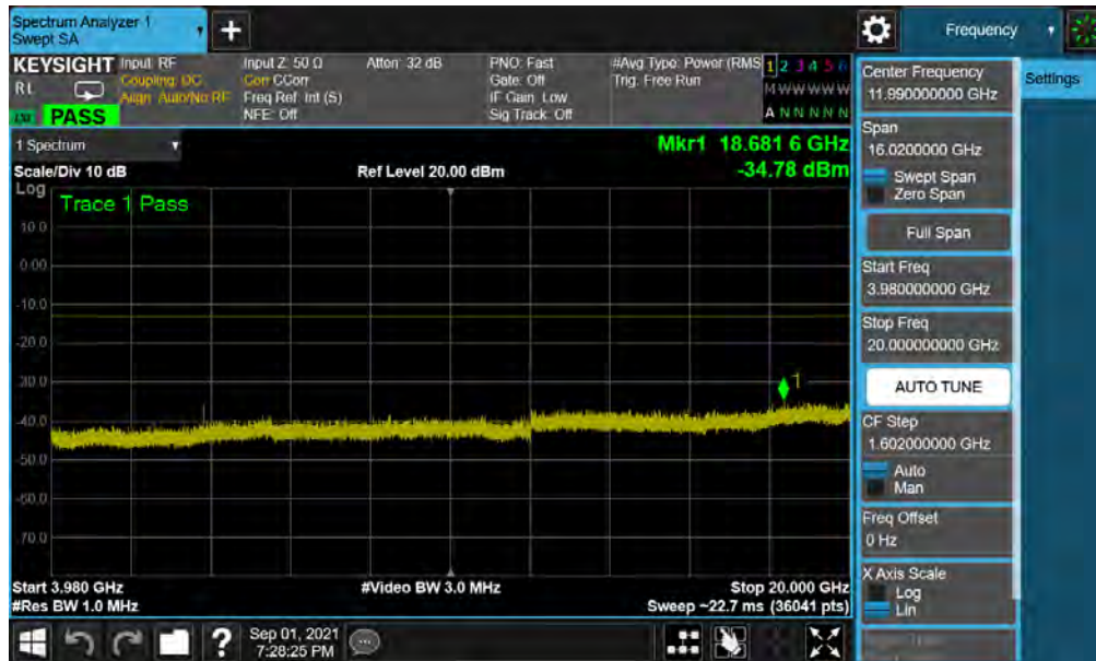
Plot 7-32. Conducted Spurious Plot (NR Band n77 - 100MHz QPSK - RB Size 1, RB Offset 0 - Mid Channel )
