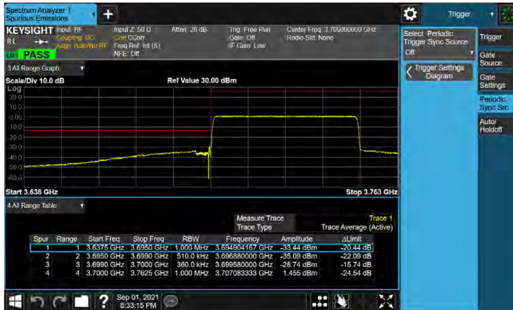
Plot 7-47. Lower ACP Plot (NR Band n77 - 50MHz CP-OFDM-QPSK - Full RB)
