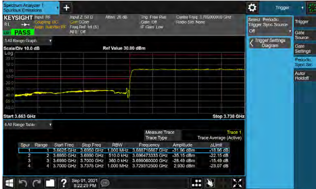
Plot 7-45. Lower ACP Plot (NR Band n77 - 60MHz CP-OFDM-QPSK – Full RB )
