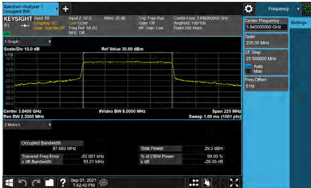
Plot 7-5. Occupied Bandwidth Plot (NR Band n77 - 90MHz QPSK - Full RB )
