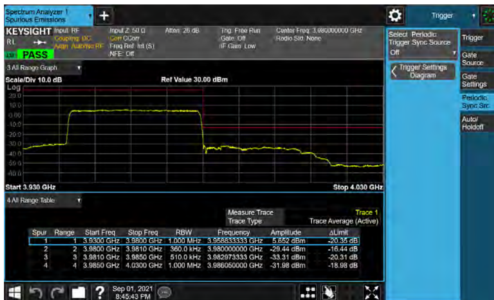
Plot 7-50. Upper ACP Plot (NR Band n77 - 40MHz CP-OFDM-QPSK - Full RB)
