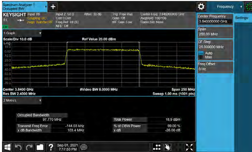
Plot 7-3. Occupied Bandwidth Plot (NR Band n77 - 100MHz 16-QAM - Full RB )
