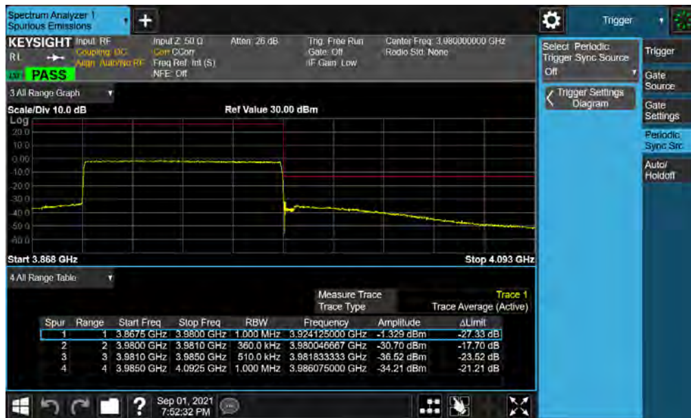
Plot 7-40. Upper ACP Plot (NR Band n77 - 90MHz CP-OFDM-QPSK - Full RB )
