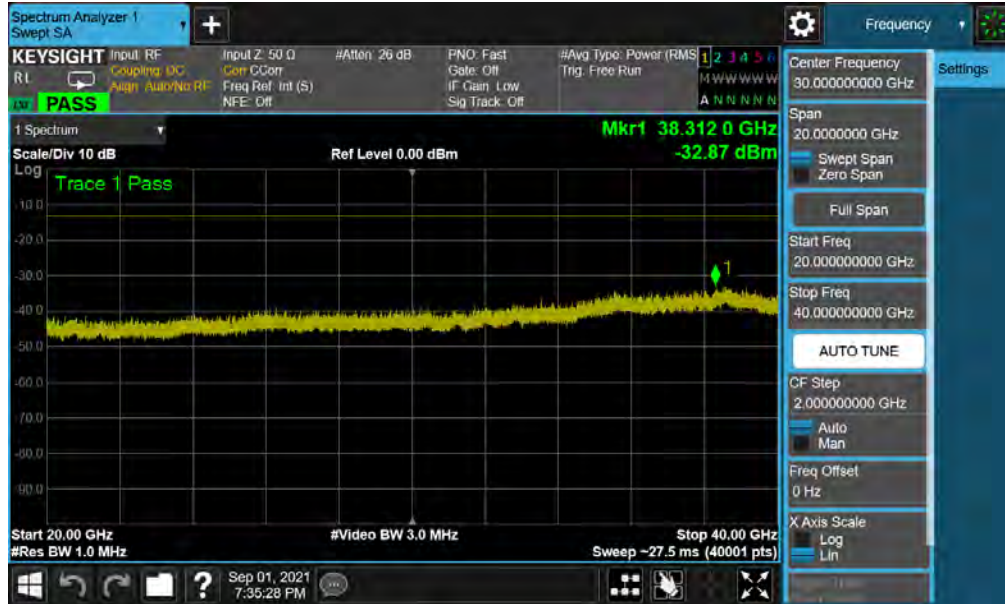
Plot 7-30. Conducted Spurious Plot (NR Band n77 - 100MHz QPSK - RB Size 1, RB Offset 0 - Low Channel )
