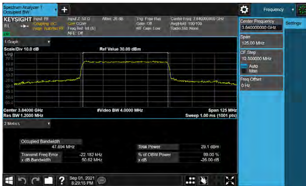
Plot 7-18. Occupied Bandwidth Plot (NR Band n77 - 50MHz 16-QAM - Full RB )
