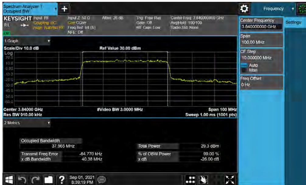
Plot 7-21. Occupied Bandwidth Plot (NR Band n77 - 40MHz 16-QAM - Full RB )
