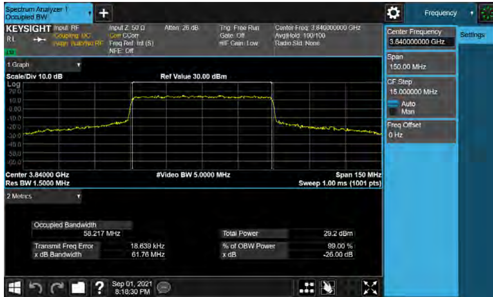
Plot 7-15. Occupied Bandwidth Plot (NR Band n77 - 60MHz 16-QAM - Full RB )
