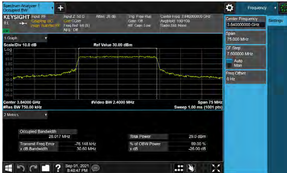
Plot 7-23. Occupied Bandwidth Plot (NR Band n77 - 30MHz QPSK - Full RB )
