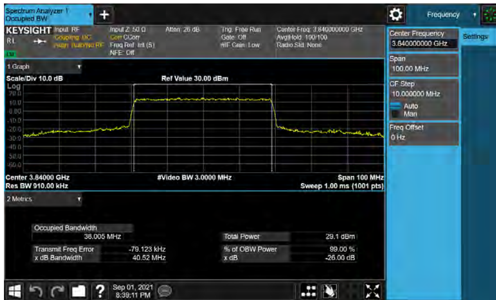
Plot 7-20. Occupied Bandwidth Plot (NR Band n77 - 40MHz QPSK - Full RB )
