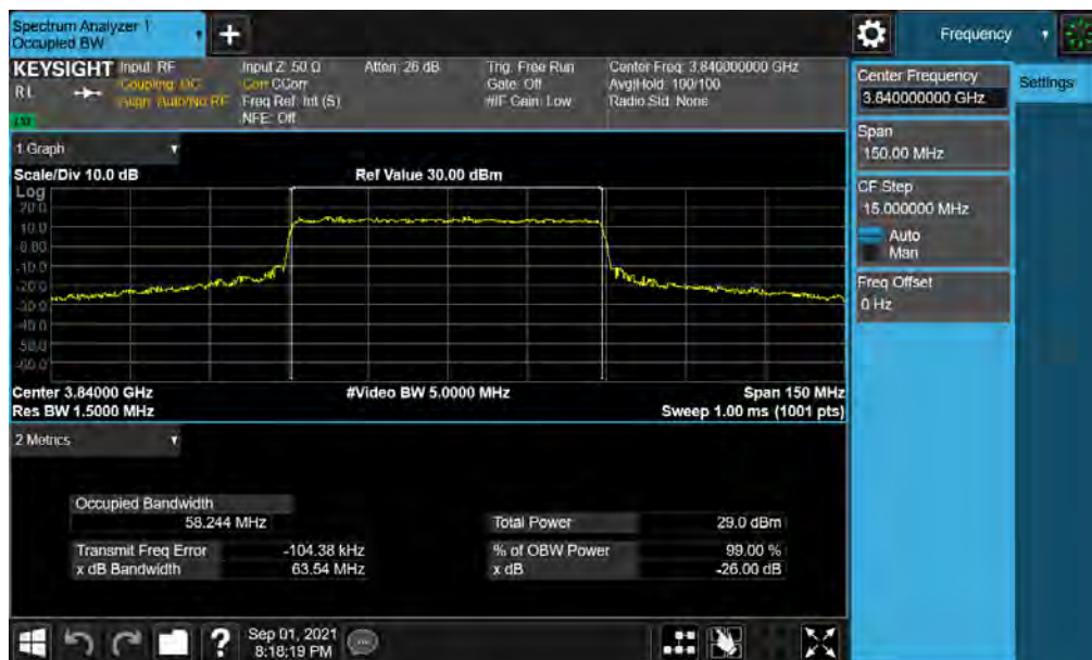
Plot 7-14. Occupied Bandwidth Plot (NR Band n77 - 60MHz QPSK - Full RB )
