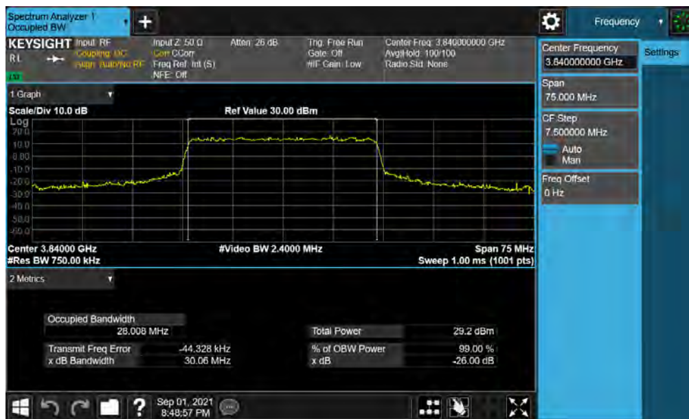
Plot 7-24. Occupied Bandwidth Plot (NR Band n77 - 30MHz 16-QAM - Full RB )
