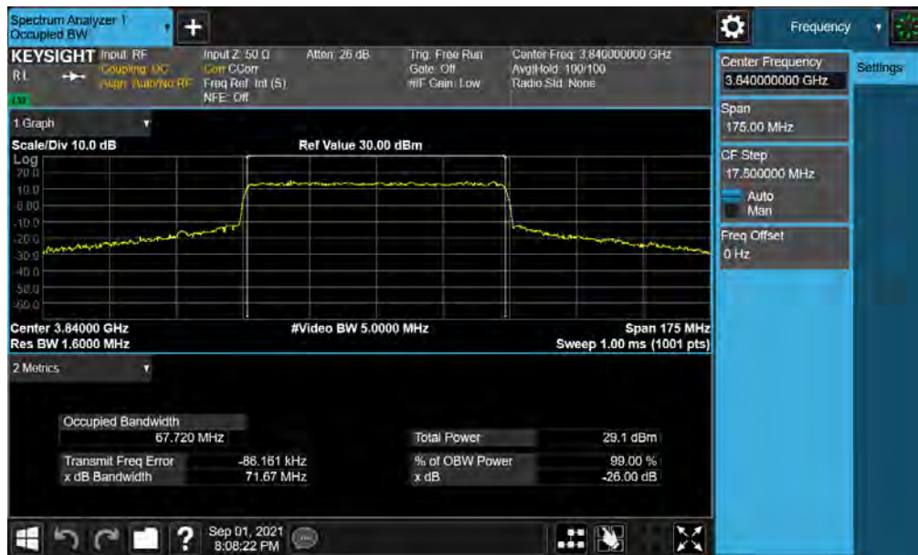
Plot 7-12. Occupied Bandwidth Plot (NR Band n77 - 70MHz 16-QAM - Full RB )
