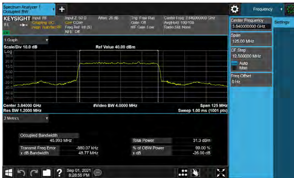
Plot 7-16. Occupied Bandwidth Plot (NR Band n77 - 50MHz \pi/2 BPSK - Full RB )
