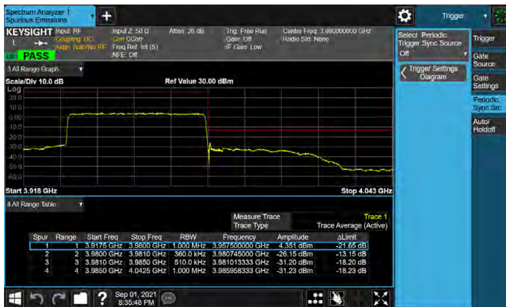
Plot 7-48. Upper ACP Plot (NR Band n77 - 50MHz CP-OFDM-QPSK - Full RB)
