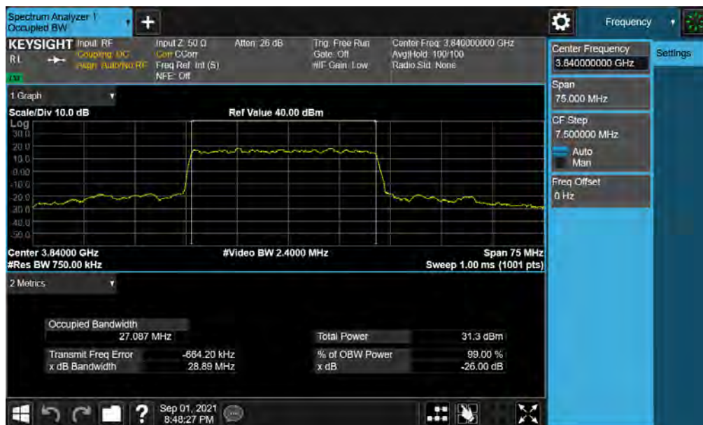
Plot 7-22. Occupied Bandwidth Plot (NR Band n77 - 30MHz \pi/2 BPSK - Full RB )
