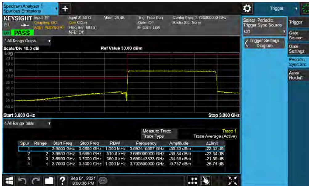
Plot 7-41. Lower ACP Plot (NR Band n77 - 80MHz CP-OFDM-QPSK - Full RB)
