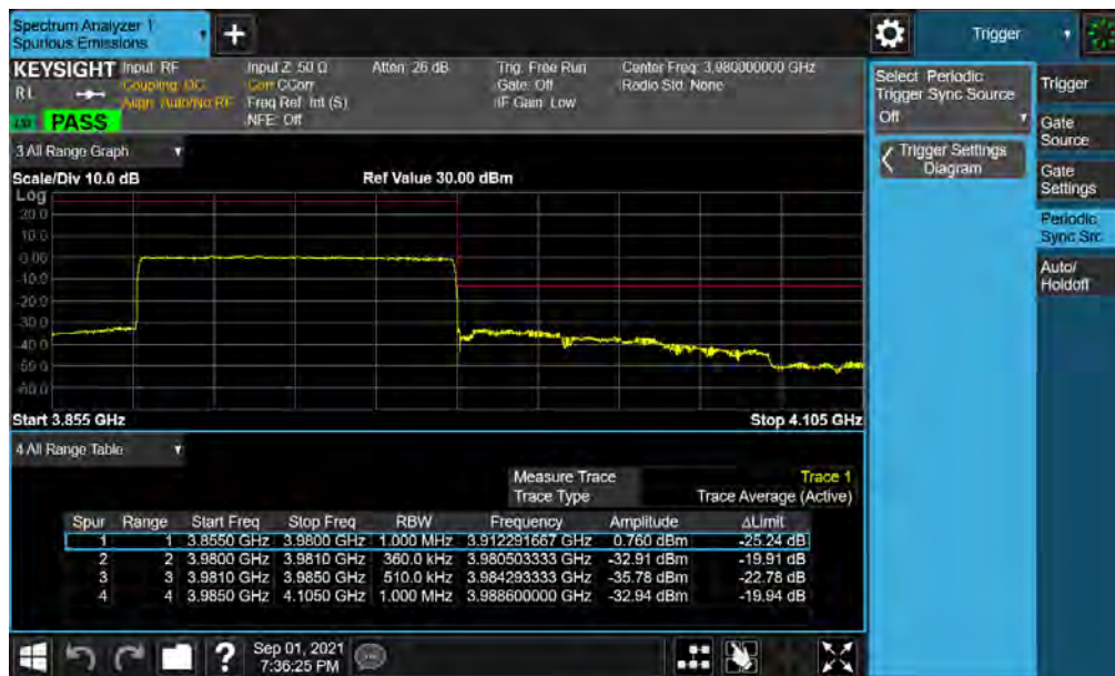
Plot 7-38. Upper ACP Plot (NR Band n77 - 100MHz CP-OFDM-QPSK – Full RB )
