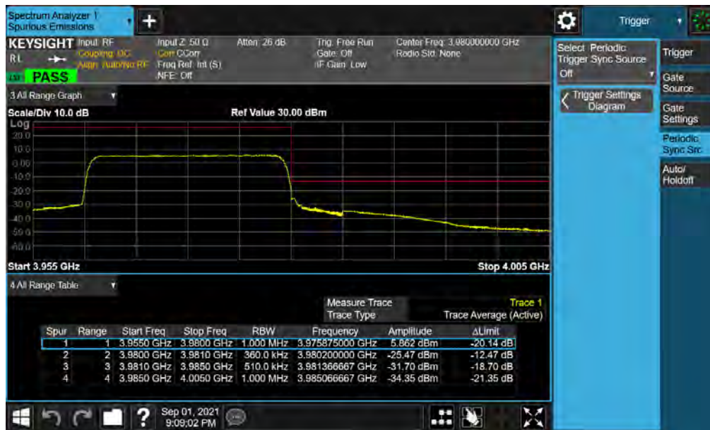
Plot 7-54. Upper ACP Plot (NR Band n77 - 20MHz CP-OFDM-QPSK – Full RB )
