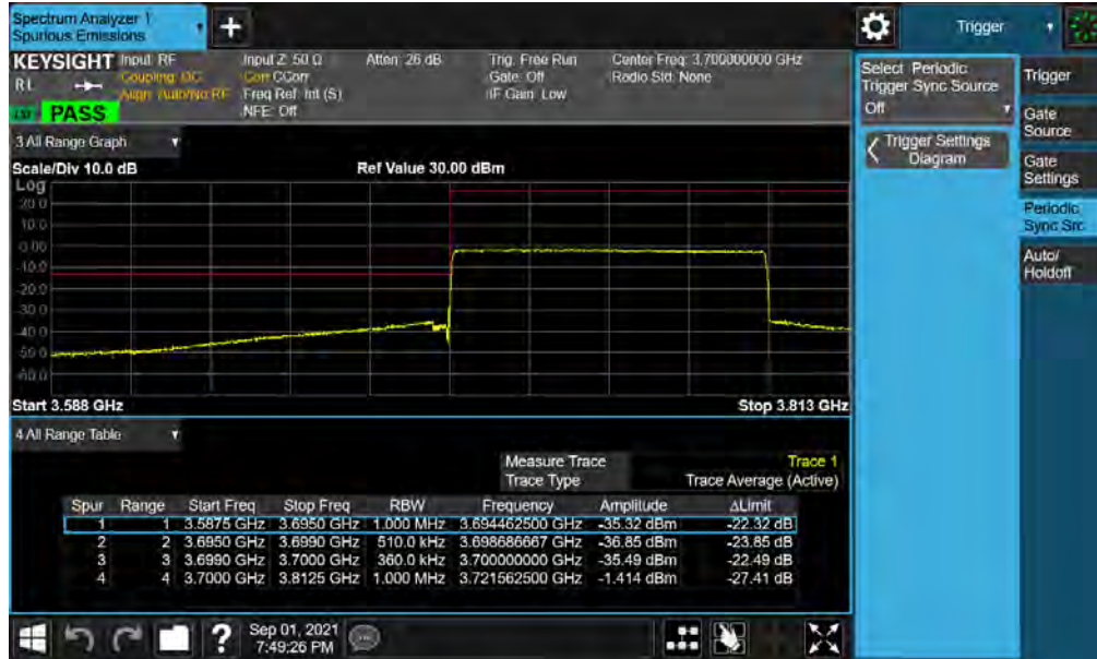
Plot 7-39. Lower ACP Plot (NR Band n77 - 90MHz CP-OFDM-QPSK - Full RB )
