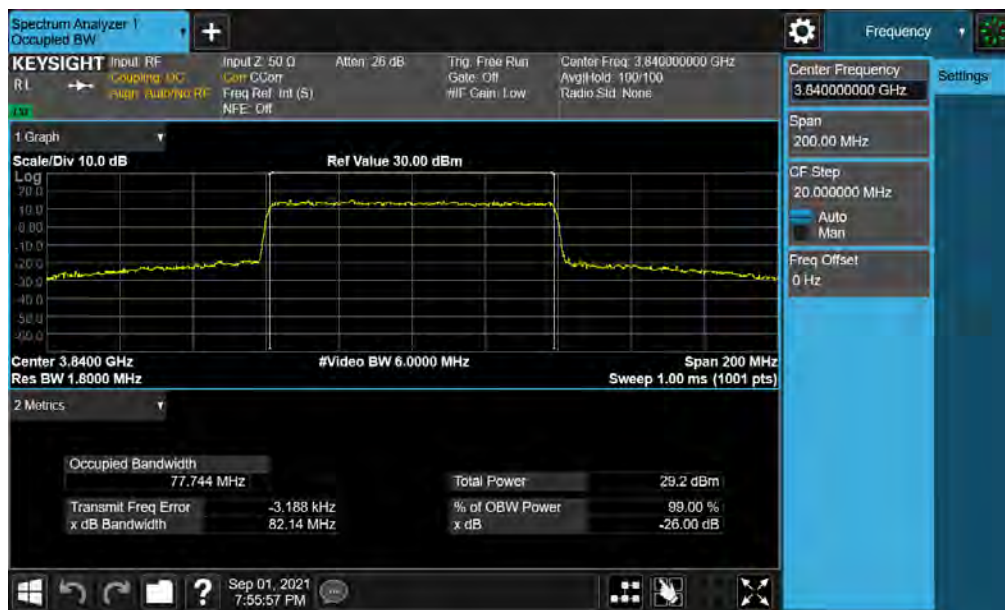
Plot 7-8. Occupied Bandwidth Plot (NR Band n77 - 80MHz QPSK - Full RB )
