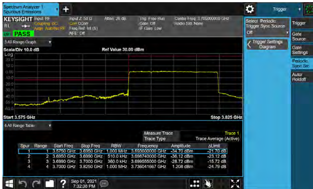
Plot 7-37. Lower ACP Plot (NR Band n77 - 100MHz CP-OFDM-QPSK – Full RB )
