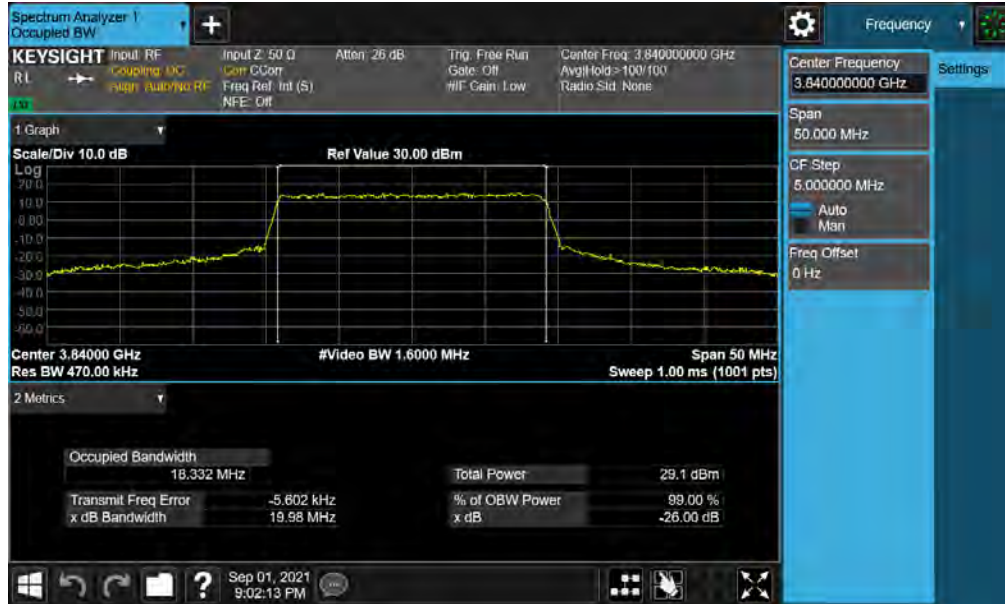
Plot 7-27. Occupied Bandwidth Plot (NR Band n77 - 20MHz 16-QAM - Full RB )
