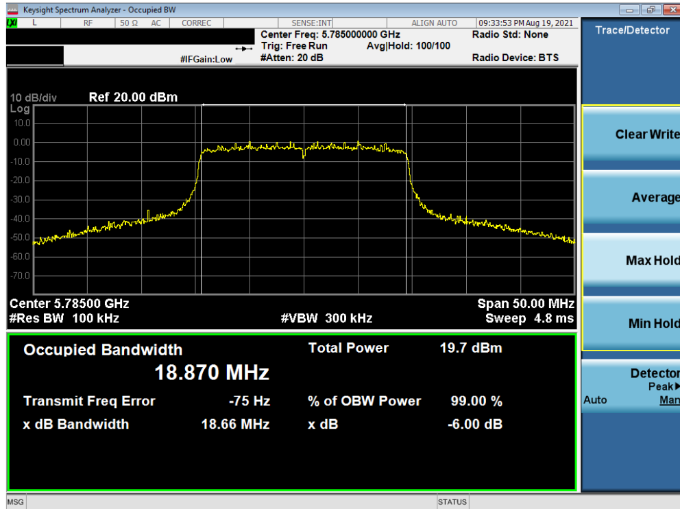
Plot 7-133. 6dB Bandwidth Plot SISO ANT2 (20MHz BW 802.11ax (UNII Band 3) – Ch. 157)
