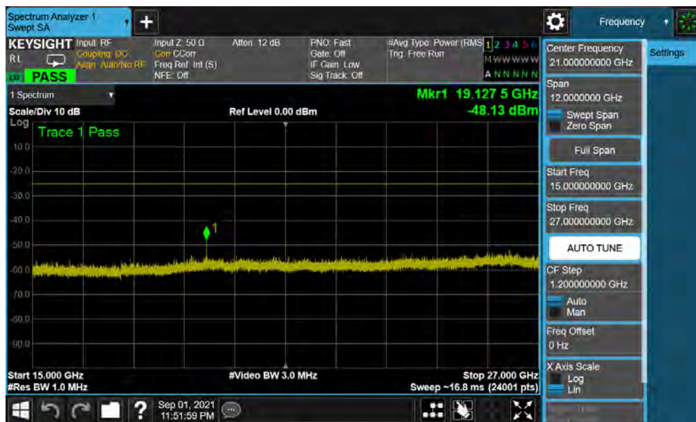
Plot 7-47. Conducted Spurious Plot (NR Band n41 - 100MHz QPSK - RB Size 1, RB Offset 0 - Mid Channel Ant1)
