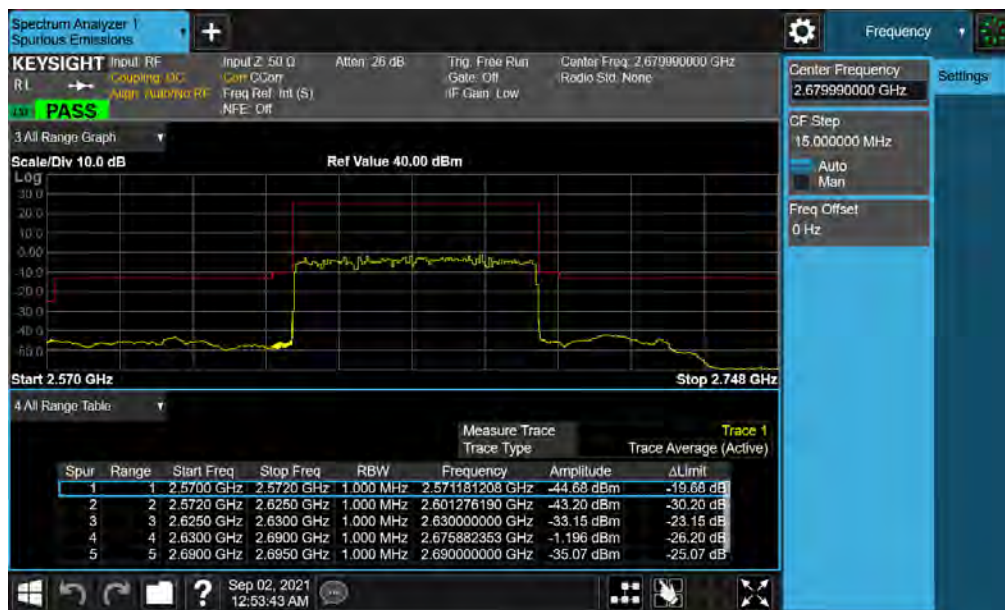
Plot 7-66. Upper ACP Plot (NR Band n41 - 60MHz CP-OFDM-QPSK – Full RB)
