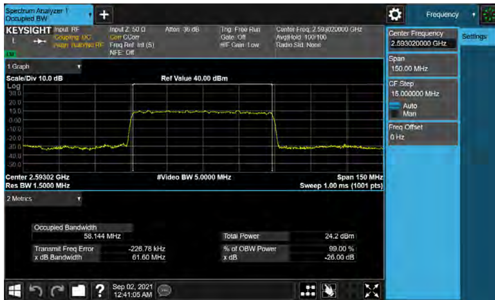
Plot 7-18. Occupied Bandwidth Plot (NR Band n41 - 60MHz \pi/2 BPSK - Full RB)
