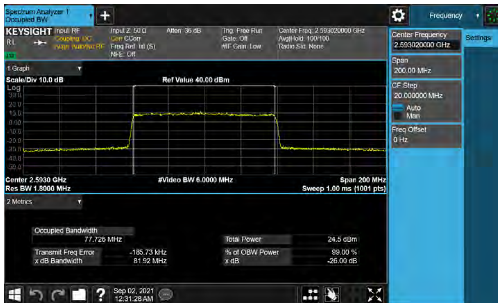
Plot 7-16. Occupied Bandwidth Plot (NR Band n41 - 80MHz QPSK - Full RB)
