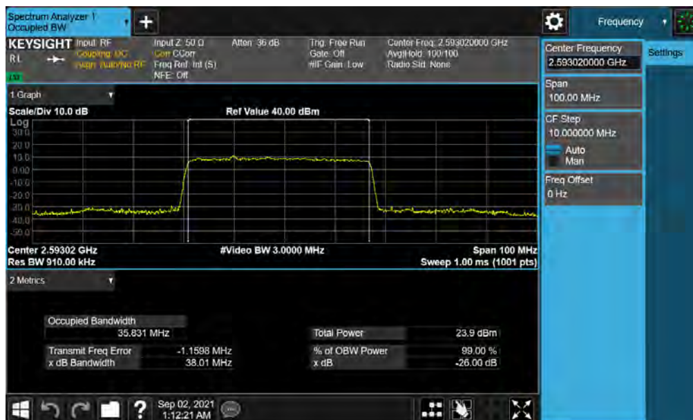
Plot 7-24. Occupied Bandwidth Plot (NR Band n41 - 40MHz \pi/2 BPSK - Full RB)
