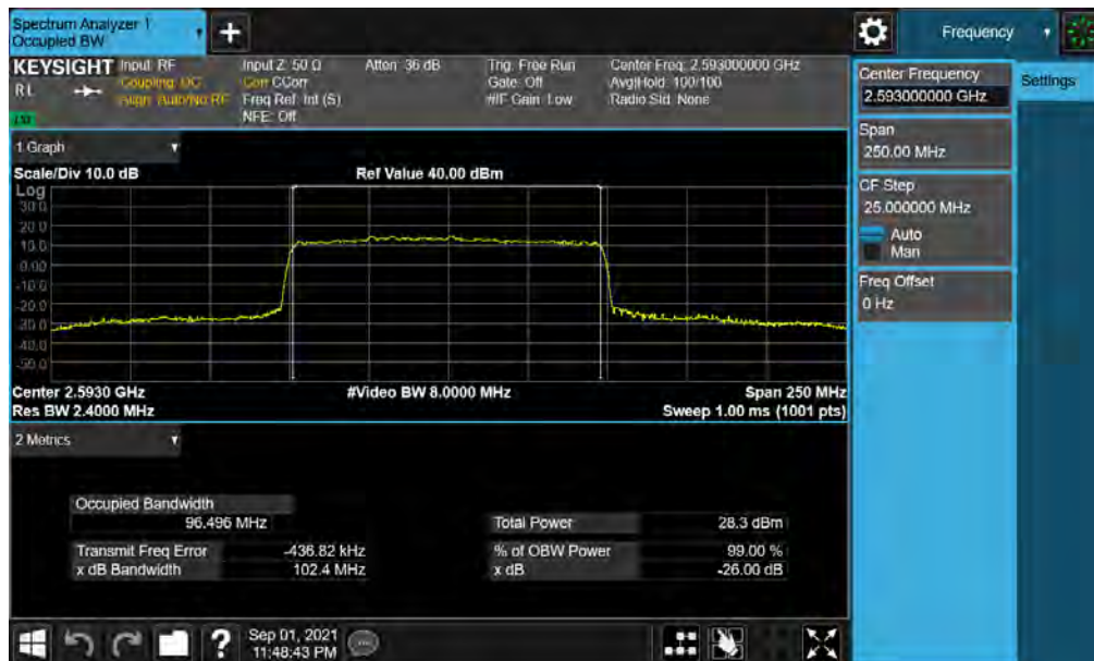
Plot 7-9. Occupied Bandwidth Plot (NR Band n41 - 100MHz \pi/2 BPSK - Full RB)
