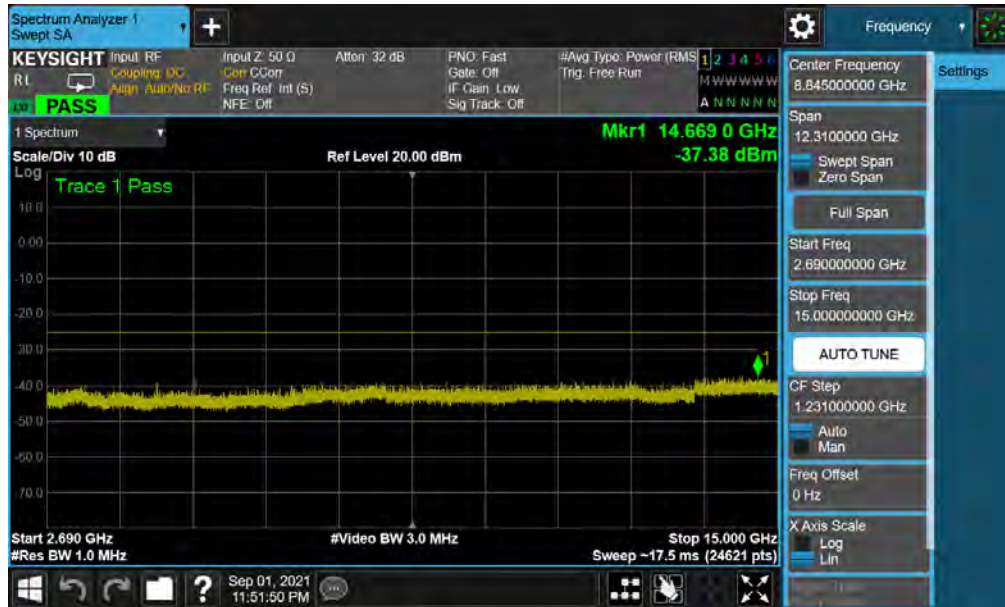
Plot 7-46. Conducted Spurious Plot (NR Band n41 - 100MHz QPSK - RB Size 1, RB Offset 0 - Mid Channel Ant1)
