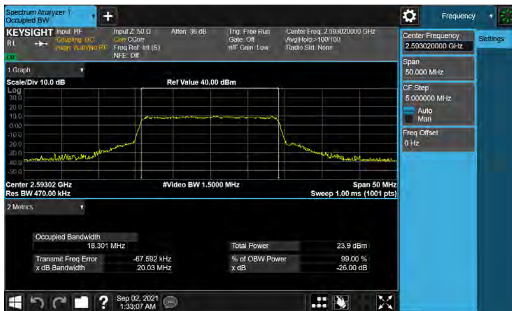
Plot 7-32. Occupied Bandwidth Plot (NR Band n41 - 20MHz 16-QAM - Full RB)
