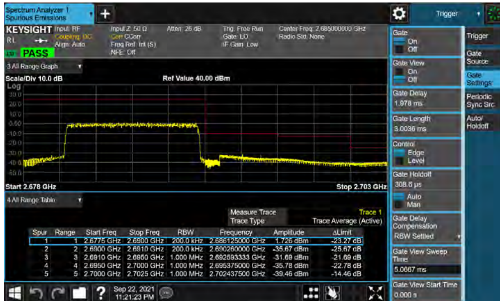
Plot 7-56. Upper ACP Plot (LTE Band 41(PC3) - 10MHz QPSK - Full RB)
