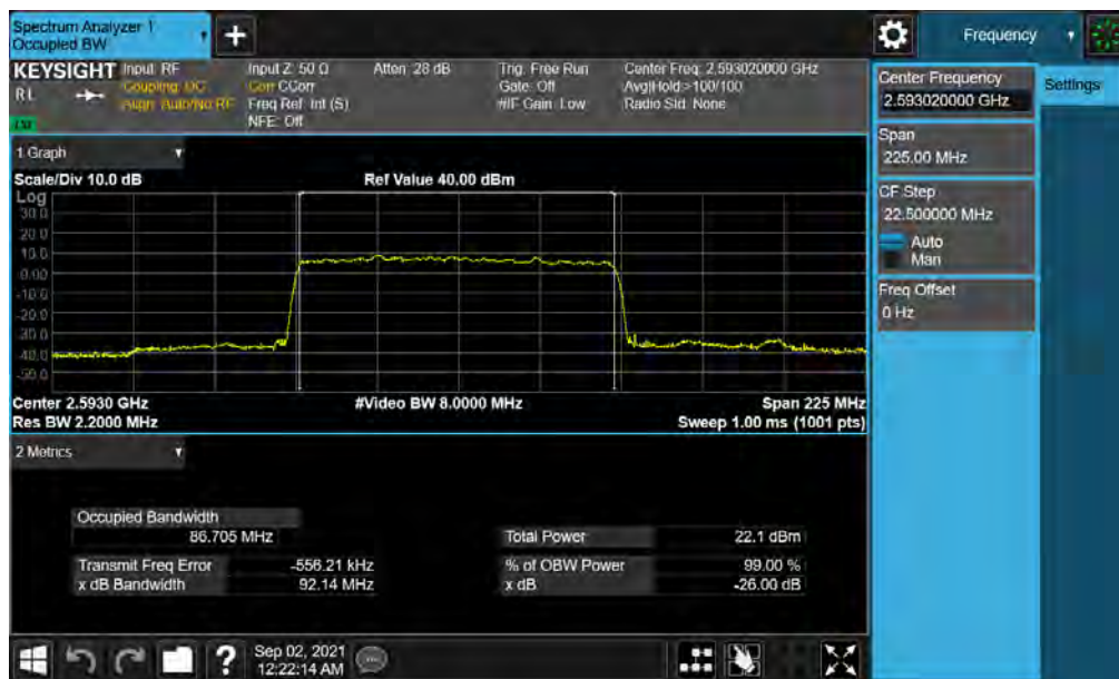
Plot 7-12. Occupied Bandwidth Plot (NR Band n41 - 90MHz \pi/2 BPSK - Full RB)
