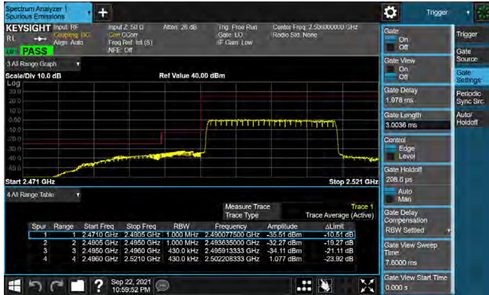
Plot 7-51. Lower ACP Plot (LTE Band 41(PC3) - 20MHz QPSK – Full RB)
