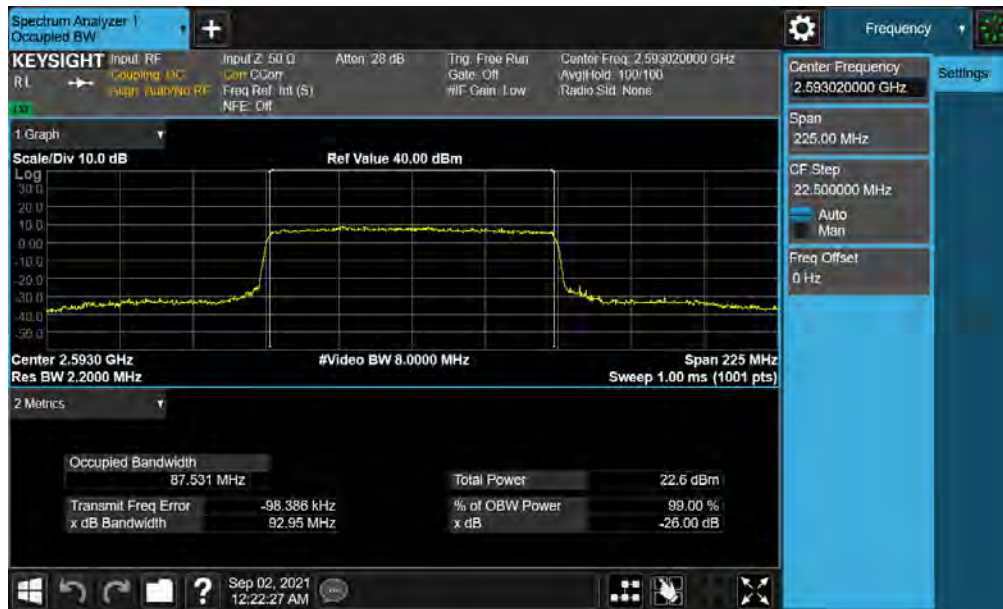
Plot 7-13. Occupied Bandwidth Plot (NR Band n41 - 90MHz QPSK - Full RB)
