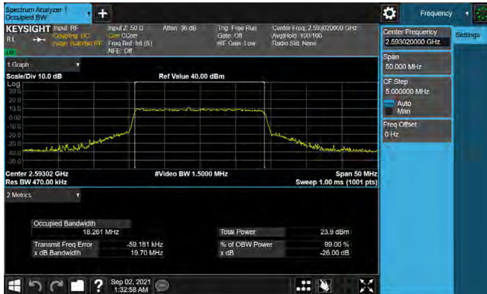
Plot 7-31. Occupied Bandwidth Plot (NR Band n41 - 20MHz QPSK - Full RB)
