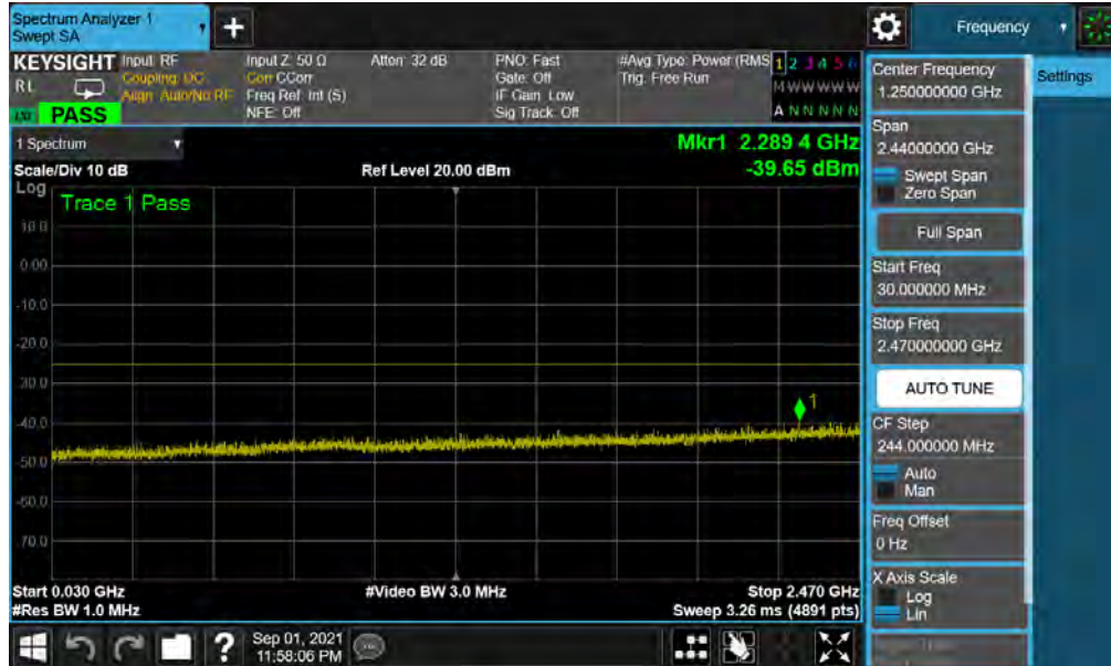
Plot 7-42. Conducted Spurious Plot (NR Band n41 - 100MHz QPSK - RB Size 1, RB Offset 0 - Low Channel Ant1)
