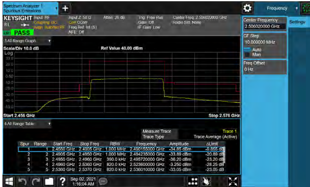
Plot 7-69. Lower ACP Plot (NR Band n41 - 40MHz CP-OFDM-QPSK - Full RB)
