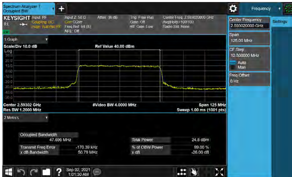
Plot 7-22. Occupied Bandwidth Plot (NR Band n41 - 50MHz QPSK - Full RB)
