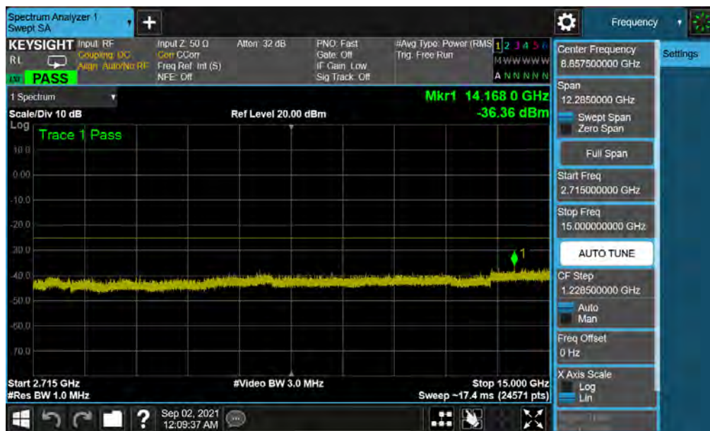
Plot 7-49. Conducted Spurious Plot (NR Band n41 - 100MHz QPSK - RB Size 1, RB Offset 0 - High Channel Ant1)
