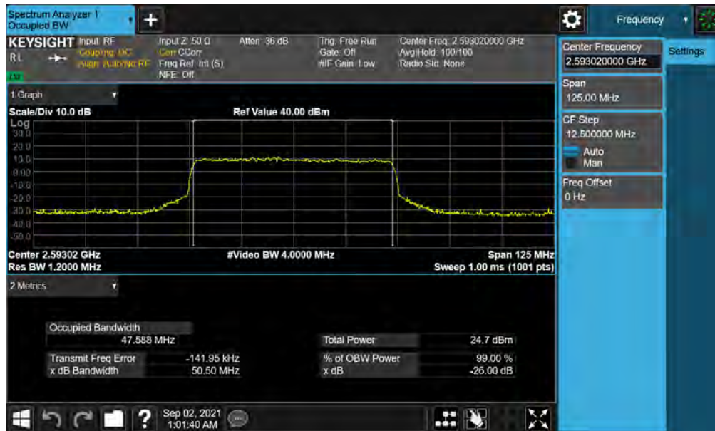
Plot 7-23. Occupied Bandwidth Plot (NR Band n41 - 50MHz 16-QAM - Full RB)
