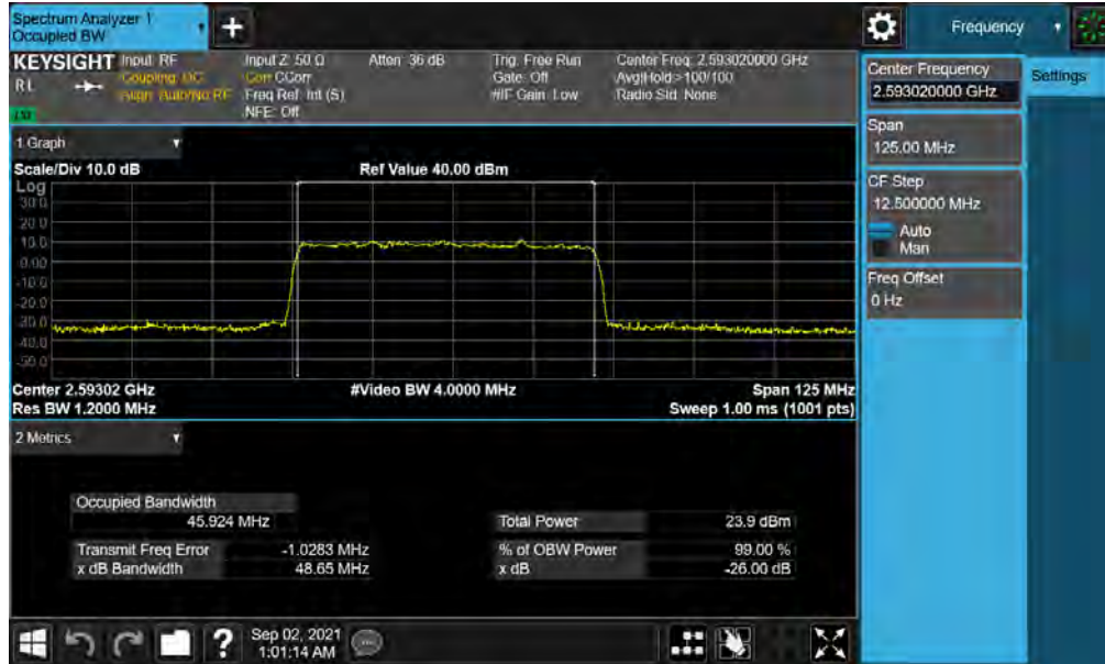
Plot 7-21. Occupied Bandwidth Plot (NR Band n41 - 50MHz \pi/2 BPSK - Full RB)
