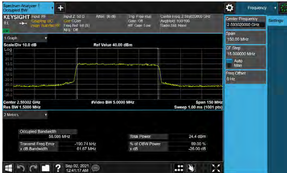
Plot 7-19. Occupied Bandwidth Plot (NR Band n41 - 60MHz QPSK - Full RB)
