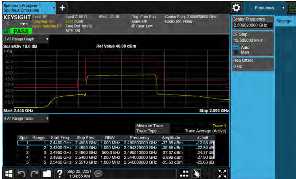
Plot 7-67. Lower ACP Plot (NR Band n41 - 50MHz CP-OFDM-QPSK – Full RB)
