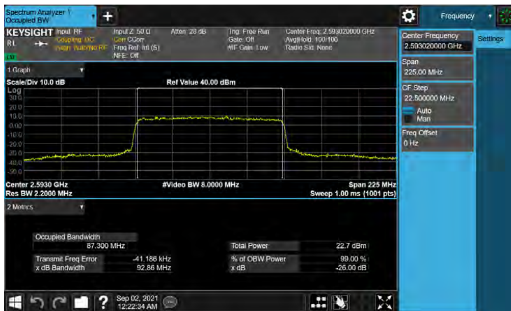
Plot 7-14. Occupied Bandwidth Plot (NR Band n41 - 90MHz 16-QAM - Full RB)
