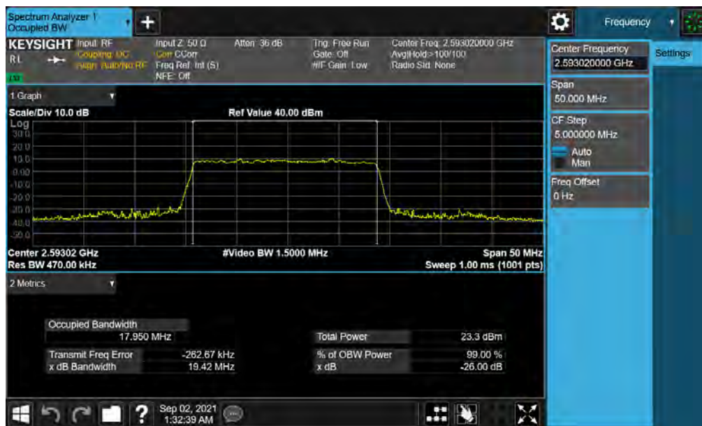
Plot 7-30. Occupied Bandwidth Plot (NR Band n41 - 20MHz \pi/2 BPSK - Full RB)
