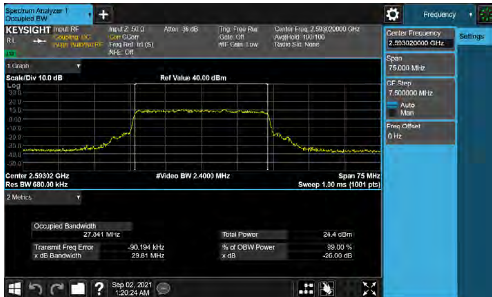
Plot 7-28. Occupied Bandwidth Plot (NR Band n41 - 30MHz QPSK - Full RB)
