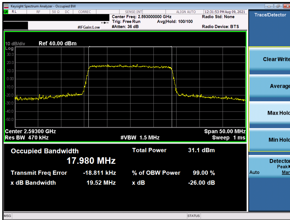
Plot 7-1. Occupied Bandwidth Plot (LTE Band 41(PC3) - 20MHz QPSK - Full RB)
