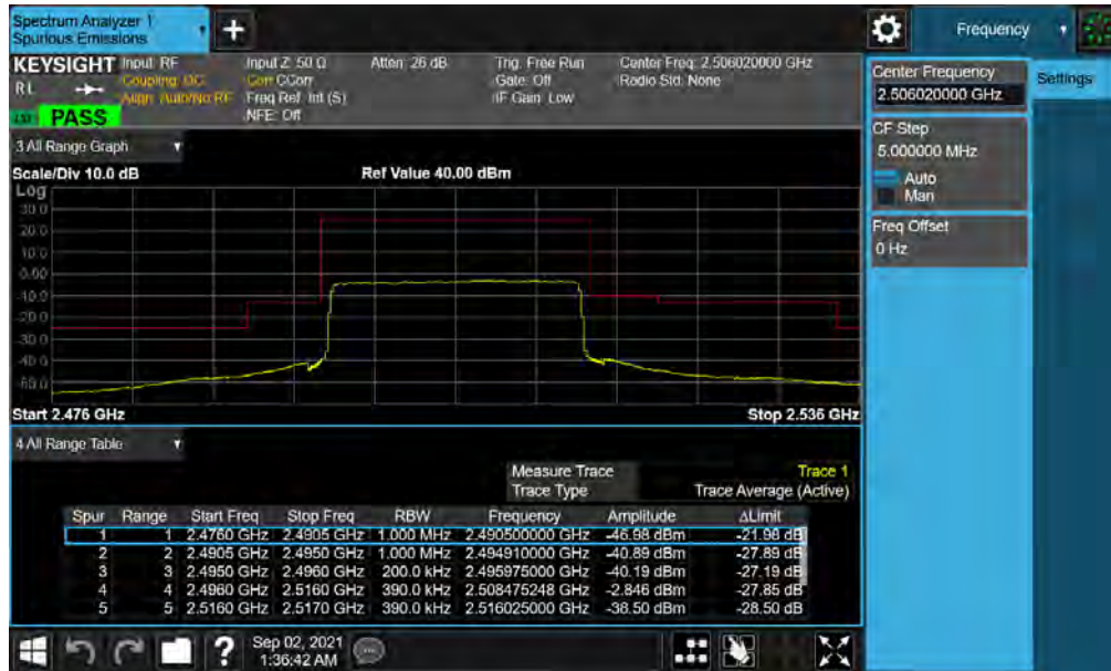
Plot 7-73. Lower ACP Plot (NR Band n41 - 20MHz CP-OFDM-QPSK – Full RB)
