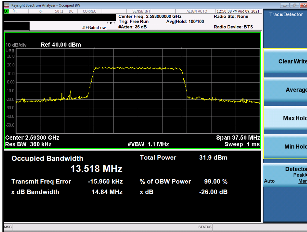
Plot 7-3. Occupied Bandwidth Plot (LTE Band 41(PC3) - 15MHz QPSK - Full RB)
