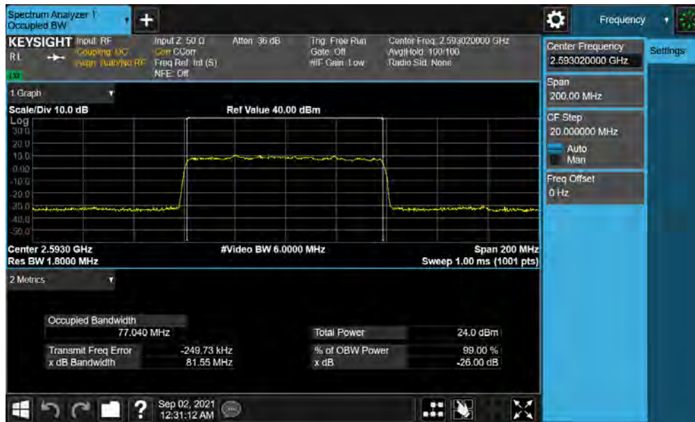
Plot 7-15. Occupied Bandwidth Plot (NR Band n41 - 80MHz \pi/2 BPSK - Full RB)
