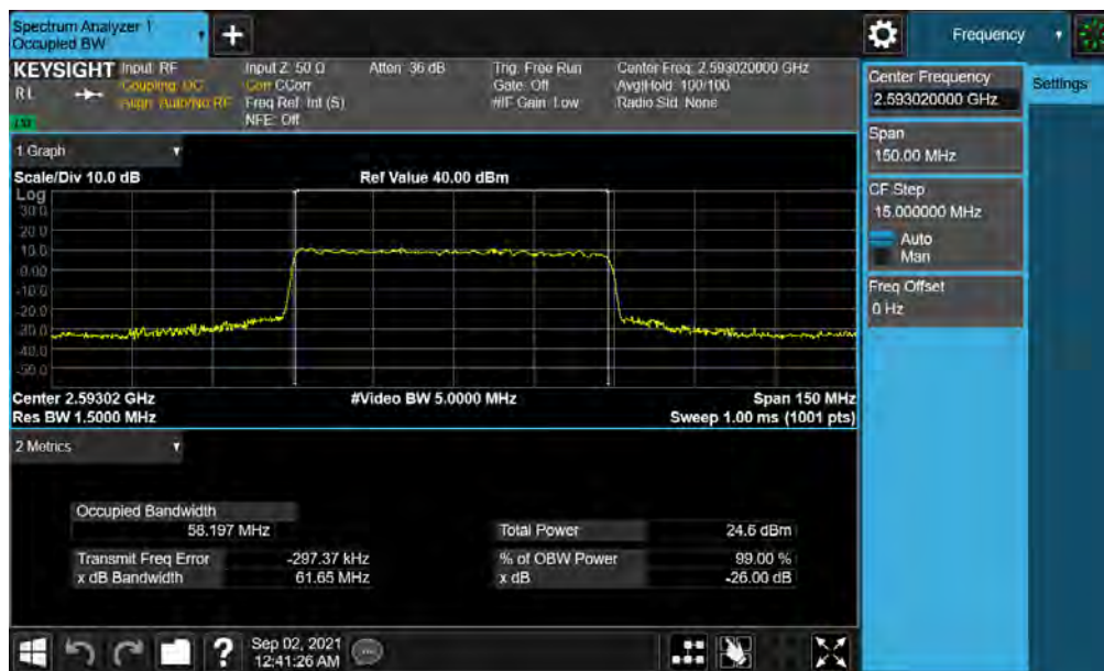
Plot 7-20. Occupied Bandwidth Plot (NR Band n41 - 60MHz 16-QAM - Full RB)
