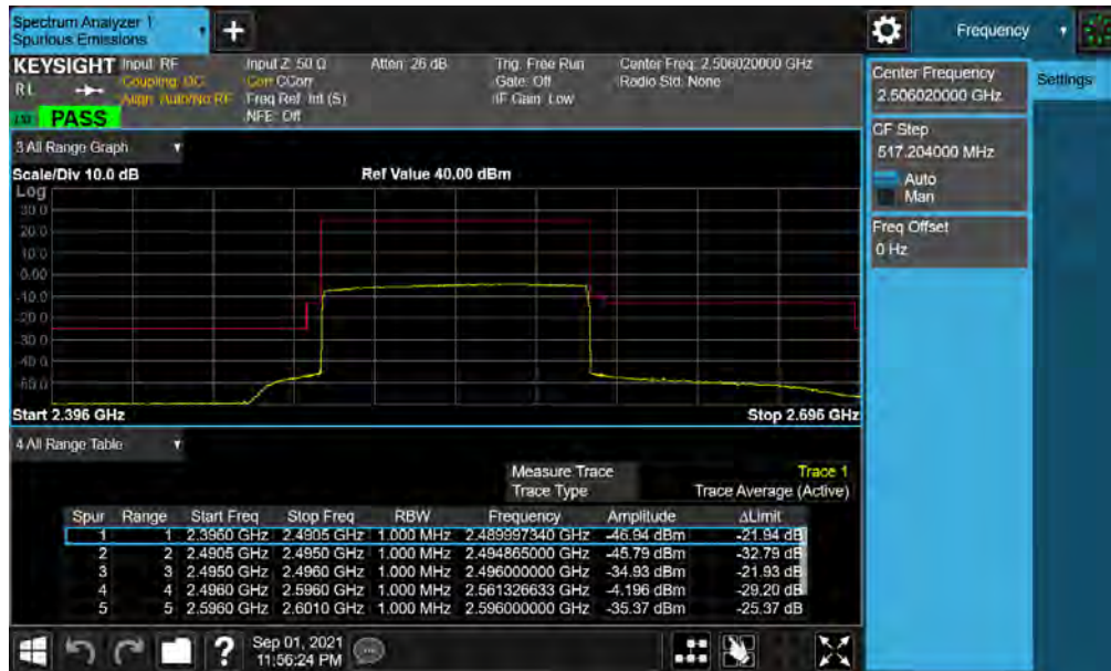
Plot 7-59. Lower ACP Plot (NR Band n41 - 100MHz CP-OFDM-QPSK – Full RB)
