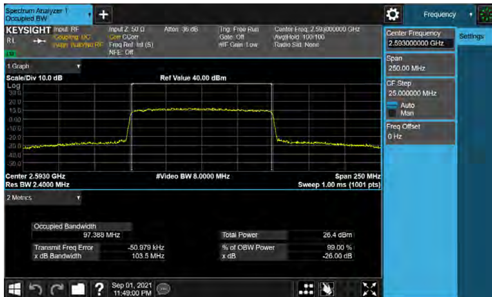
Plot 7-10. Occupied Bandwidth Plot (NR Band n41 - 100MHz QPSK - Full RB)
