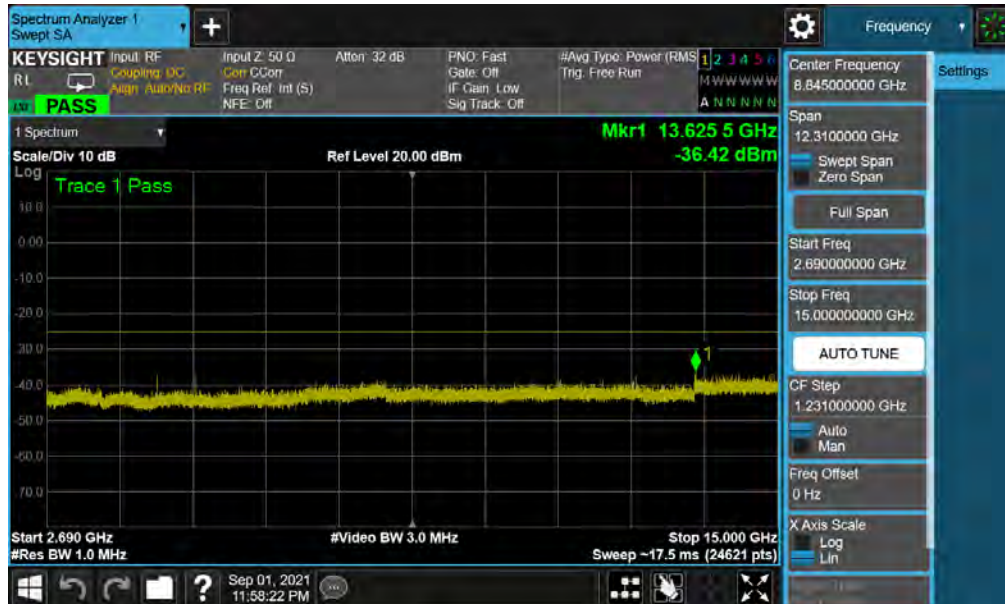
Plot 7-43. Conducted Spurious Plot (NR Band n41 - 100MHz QPSK - RB Size 1, RB Offset 0 - Low Channel Ant1)
