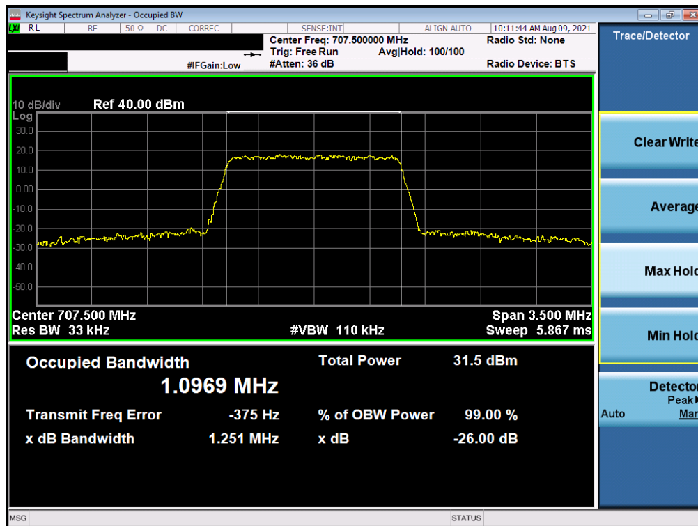
Plot 7-15. Occupied Bandwidth Plot (LTE Band 12 – 1.4MHz QPSK - Full RB – Main Ant)
