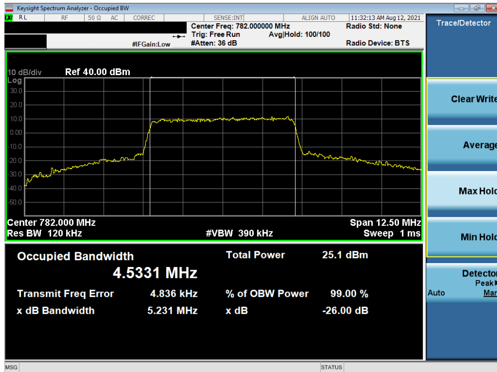
Plot 7-60. Occupied Bandwidth Plot (LTE Band 13 - 5MHz QPSK - Full RB – Sub Ant)
