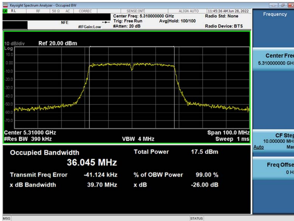
Plot 7-28. 26dB Bandwidth Plot MIMO ANT1 (802.11n – 40MHz BW (UNII Band 2A) – Ch. 62)
