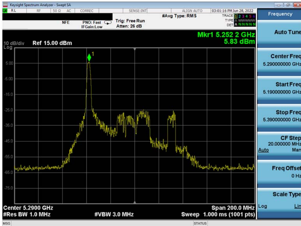
Plot 7-134. Power Spectral Density Plot MIMO ANT1 (80MHz BW 802.11ax – 26 Tones (UNII Band 2A) – Ch. 58)
