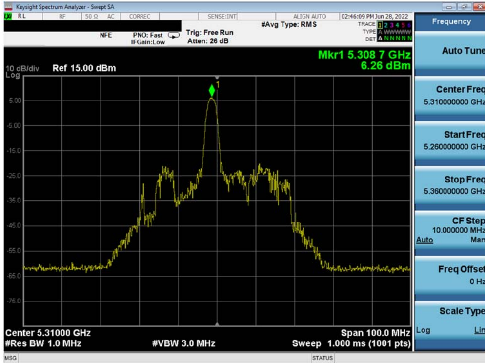
Plot 7-133. Power Spectral Density Plot MIMO ANT1 (40MHz BW 802.11ax – 26 Tones (UNII Band 2A) – Ch. 62)
