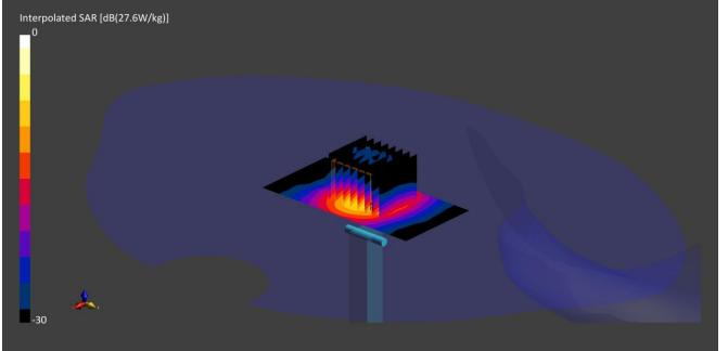
Communication System: CW UID: 0; Frequency: 5750.0 MHz; Duty Cycle: 1;
