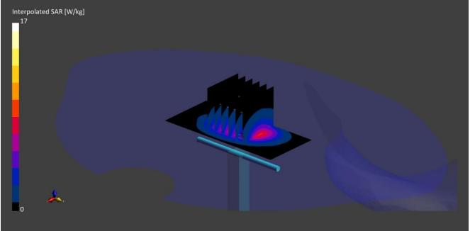
Communication System: CW UID: 0; Frequency: 1900.0 MHz; Duty Cycle: 1;
