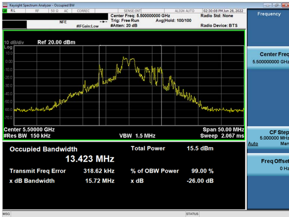
Plot 7-15. 26dB Bandwidth Plot MIMO ANT1 (20MHz BW 802.11ax – 26 Tones (UNII Band 2C) – Ch. 100)
