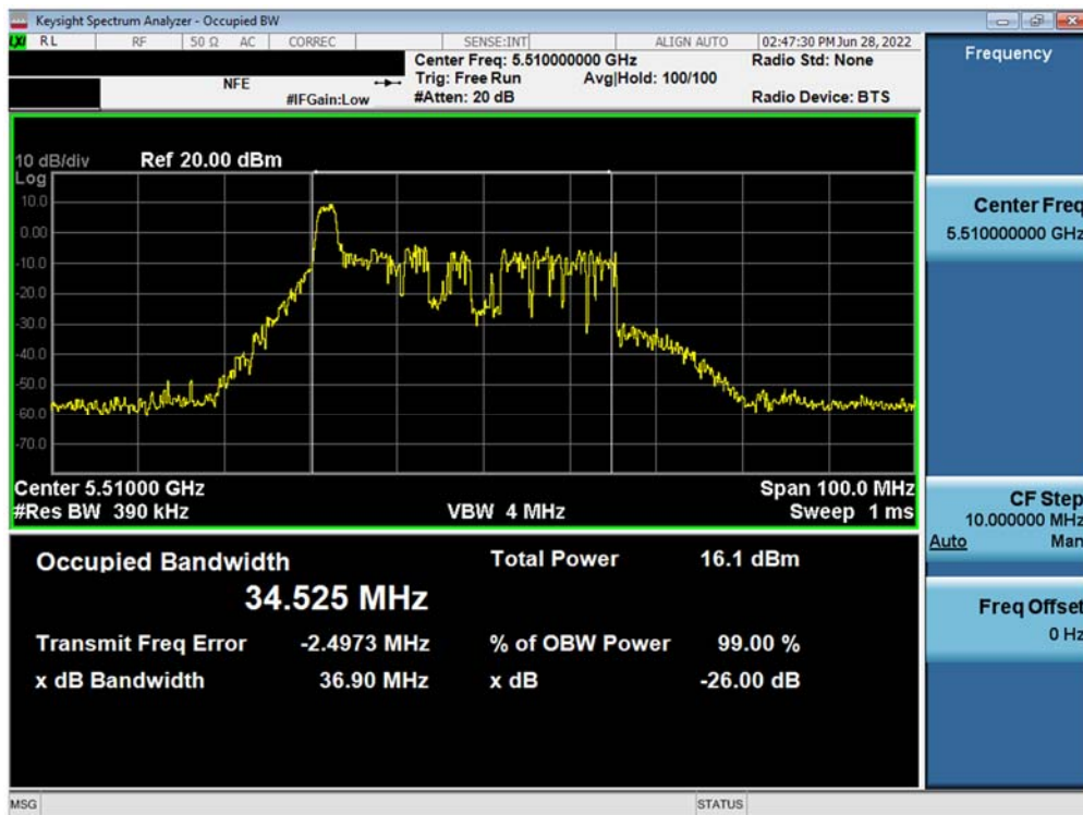
Plot 7-18. 26dB Bandwidth Plot MIMO ANT1 (40MHz BW 802.11ax – 26 Tones (UNII Band 2C) – Ch. 102)
