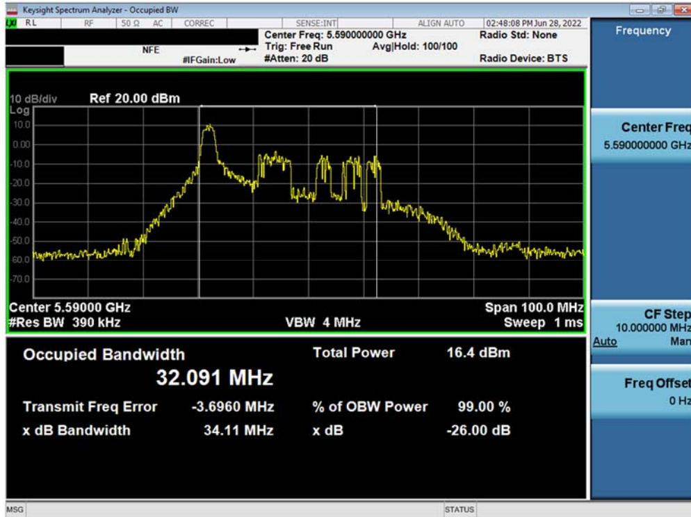
Plot 7-19. 26dB Bandwidth Plot MIMO ANT1 (40MHz BW 802.11ax – 26 Tones (UNII Band 2C) – Ch. 118)
