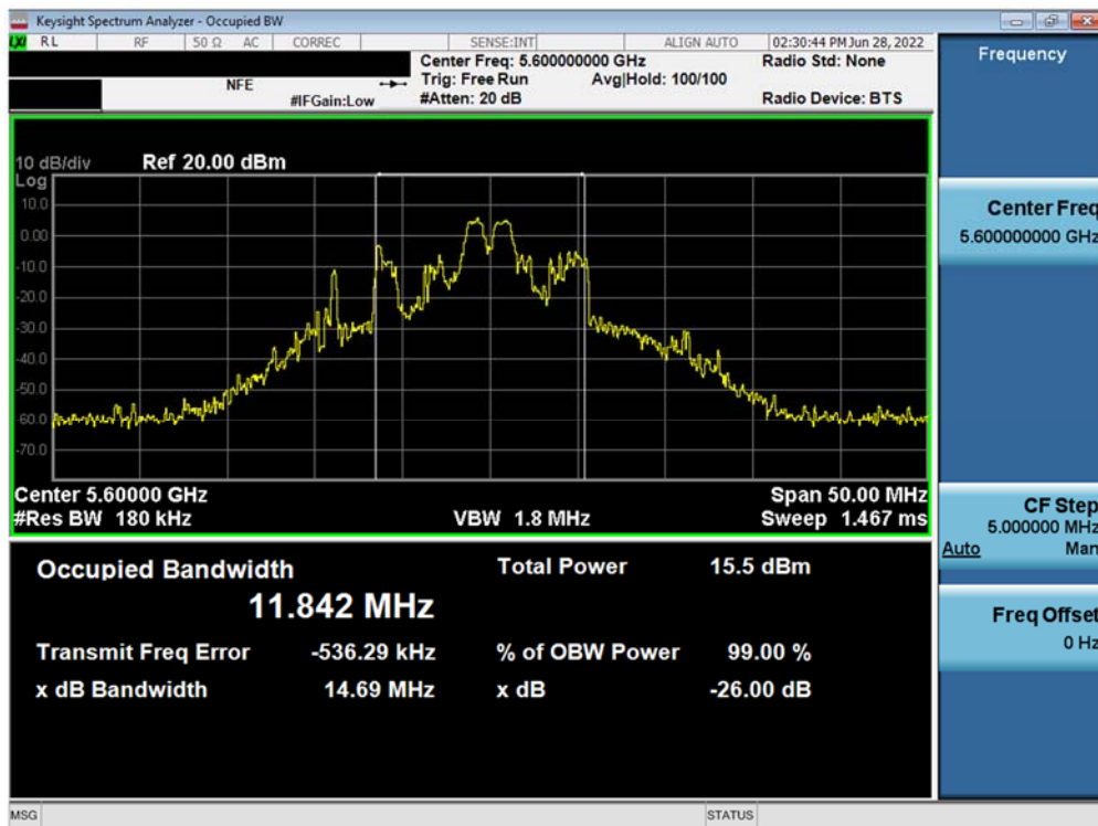
Plot 7-16. 26dB Bandwidth Plot MIMO ANT1 (20MHz BW 802.11ax – 26 Tones (UNII Band 2C) – Ch. 120)
