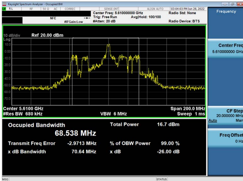
Plot 7-22. 26dB Bandwidth Plot MIMO ANT1 (80MHz BW 802.11ax – 26 Tones (UNII Band 2C) – Ch. 122)
