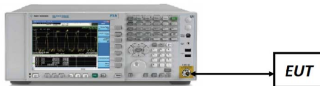
Figure 7-3. Test Instrument & Measurement Setup
