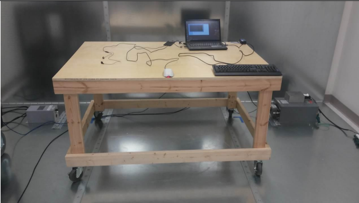
Figure 2 Test Setup for Conducted Emissions -Sync
