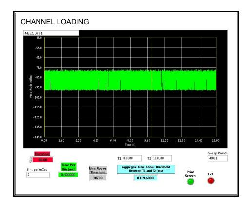
The level of traffic loading on the channel by the EUT is 83.196%.
