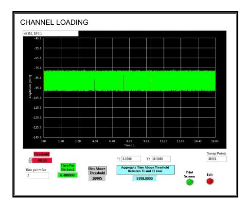
The level of traffic loading on the channel by the EUT is 83.98%.
