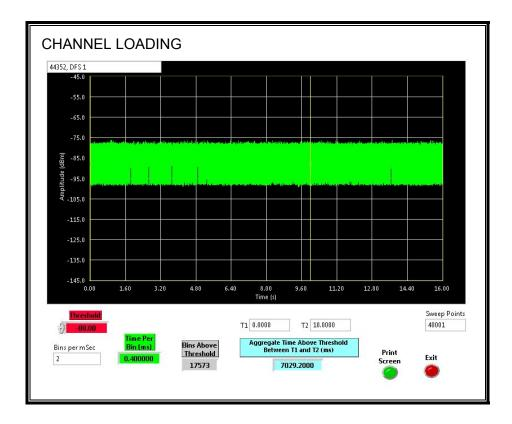
The level of traffic loading on the channel by the EUT is 70.292%.
