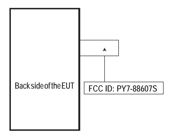
The FCC ID is not on the exterior of the device but labelling meets the conditions allowed in KDB 784748 for the label to be placed in a user accessible area:
