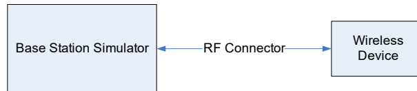
Figure 9-4 Power Measurement Setup – NR FDD
