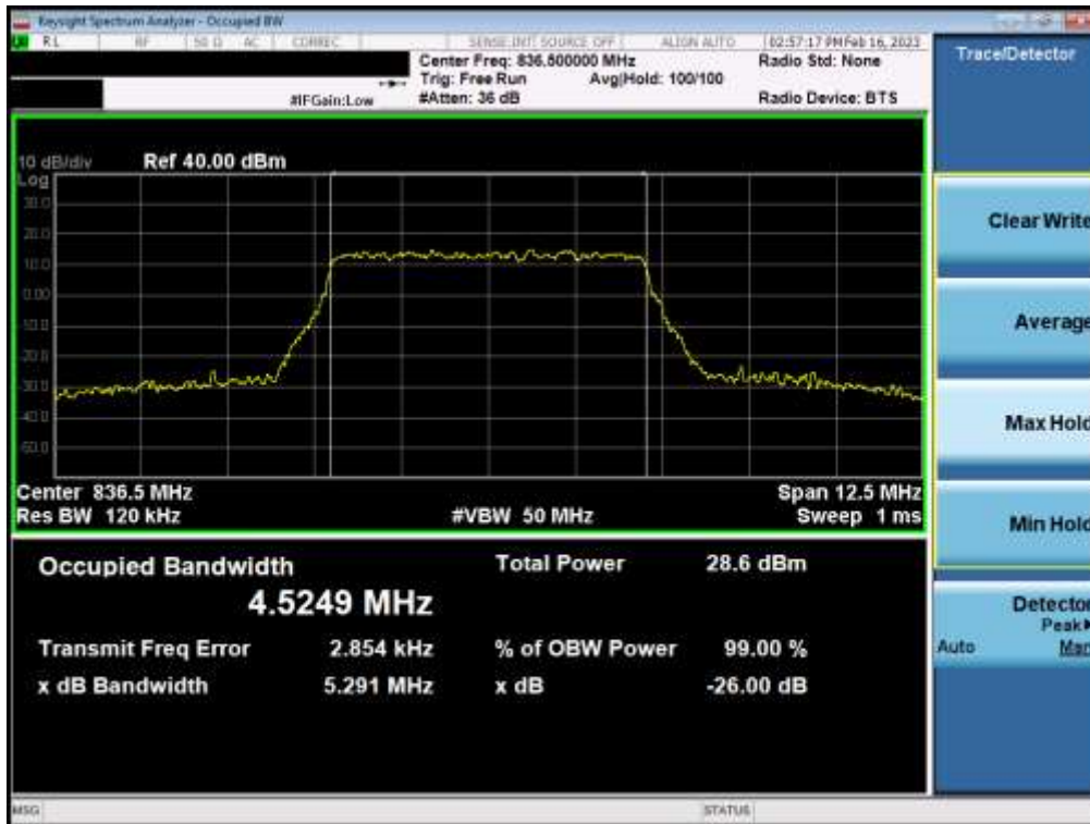
Plot 7-40. Occupied Bandwidth Plot (NR Band n5 - 5MHz 16-QAM - Full RB - Sub)
