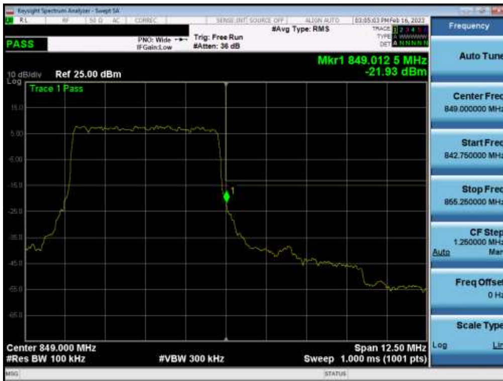
Plot 7-129. Upper Band Edge Plot (NR Band n5 – 5.0MHz - Full RB - Sub)
