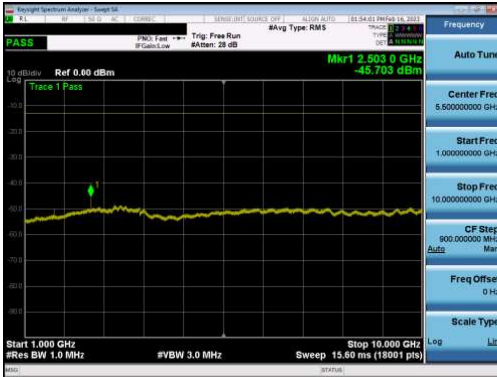
Plot 7-73. Conducted Spurious Plot (NR Band n5 - 20.0MHz - 1 RB - Low Channel - Sub)
