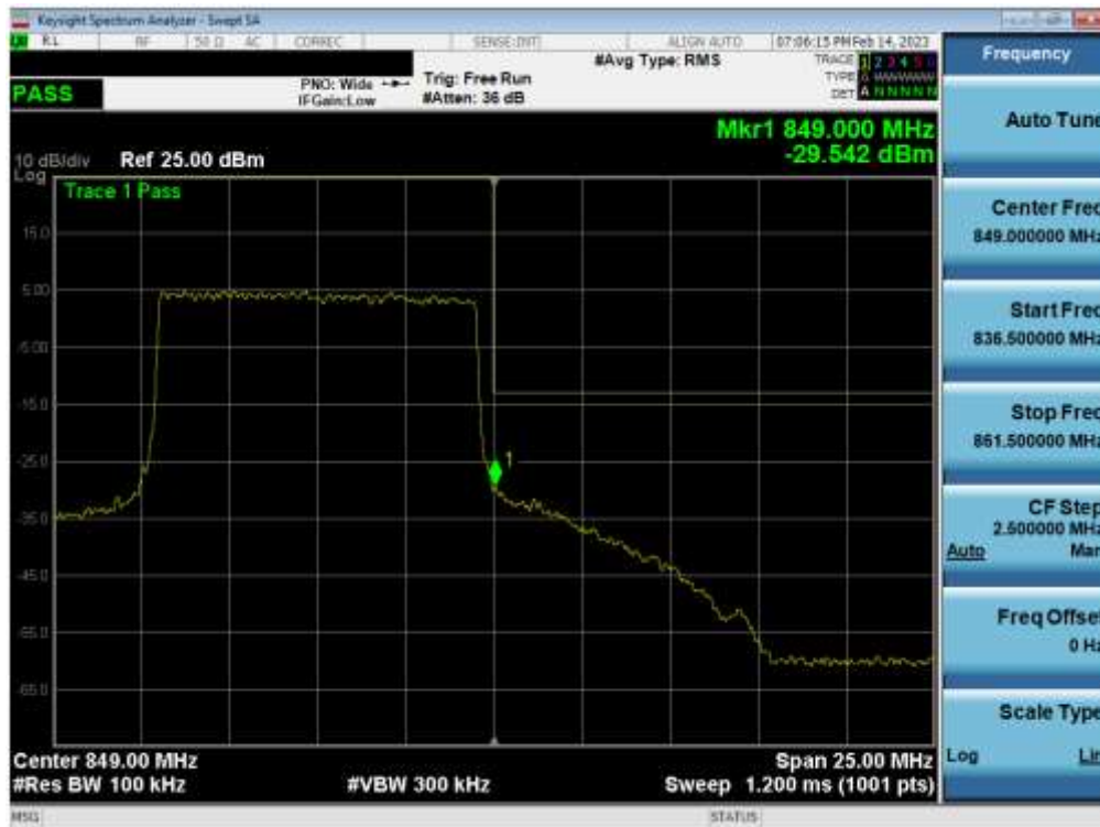
Plot 7-99. Upper Band Edge Plot (LTE Band 5 - 10MHz QPSK – Full RB - Main1)
