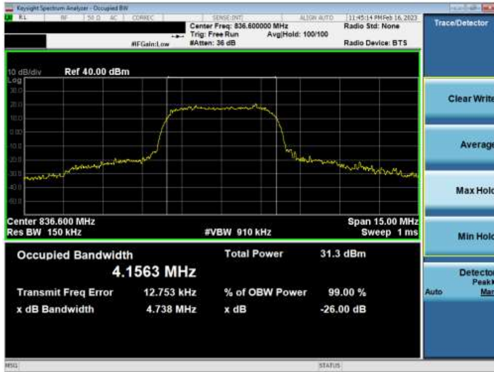
Plot 7-43. Occupied Bandwidth Plot (WCDMA, Ch. 4183 – Main1)
