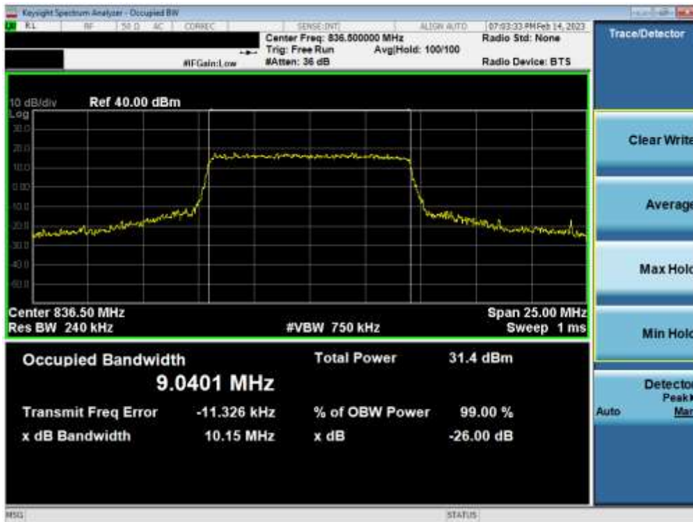
Plot 7-2. Occupied Bandwidth Plot (LTE Band 5 - 10MHz 16-QAM - Full RB - Main1)
