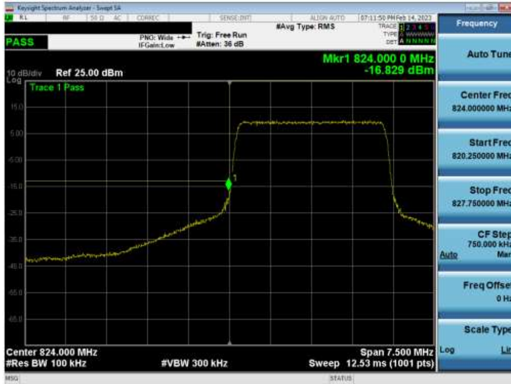
Plot 7-102. Lower Band Edge Plot (LTE Band 5 - 3MHz QPSK – Full RB - Main1)
