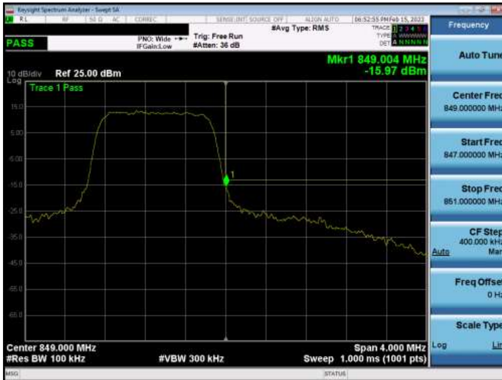
Plot 7-113. Upper Band Edge Plot (LTE Band 5 – 1.4MHz QPSK – Full RB - Sub)
