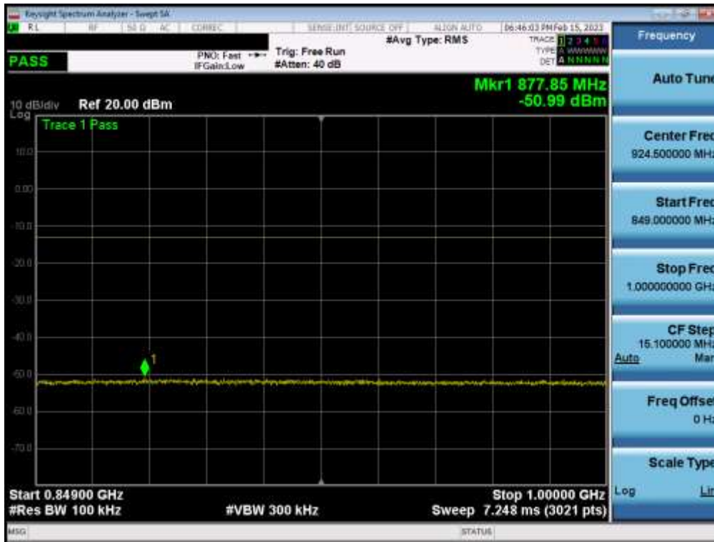
Plot 7-57. Conducted Spurious Plot (LTE Band 5 - 10MHz QPSK - 1 RB - Mid Channel - Sub)
