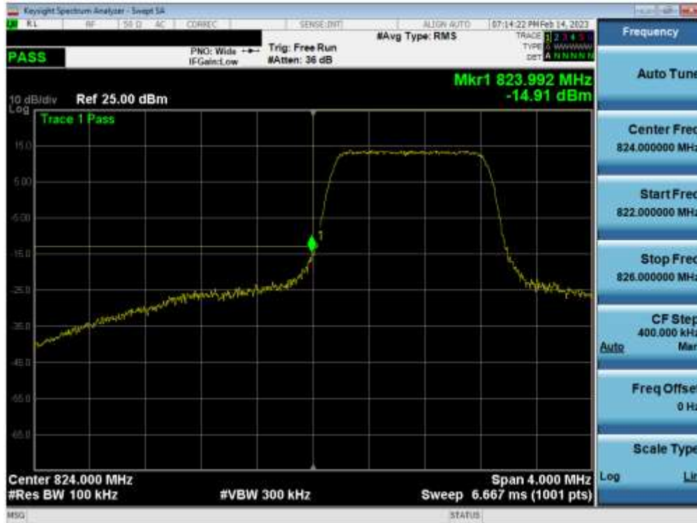
Plot 7-104. Lower Band Edge Plot (LTE Band 5 – 1.4MHz QPSK – Full RB - Main1)
