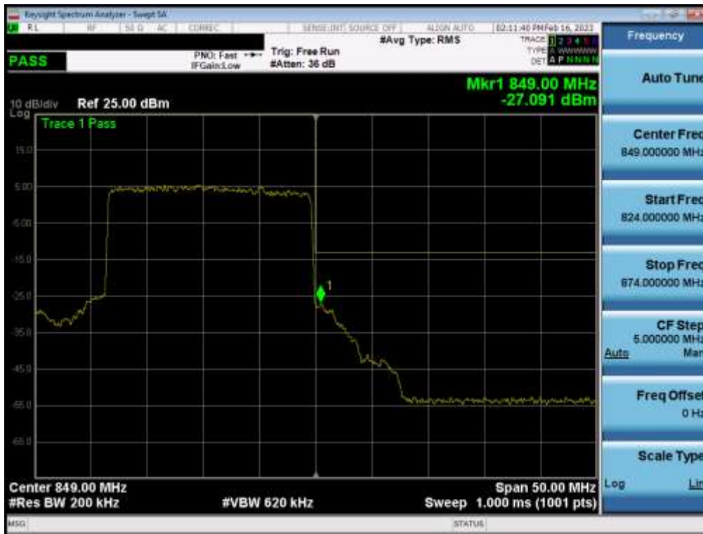
Plot 7-123. Upper Band Edge Plot (NR Band n5 – 20.0MHz - Full RB - Sub)
