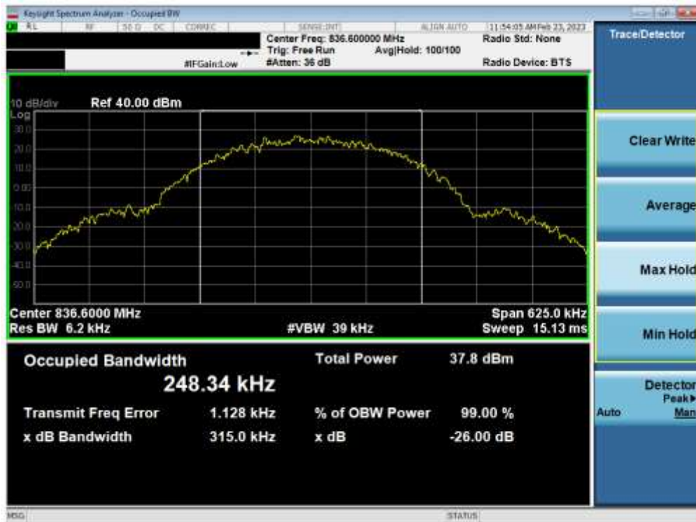
Plot 7-42. Occupied Bandwidth Plot (EDGE, Ch. 190 – Main1)
