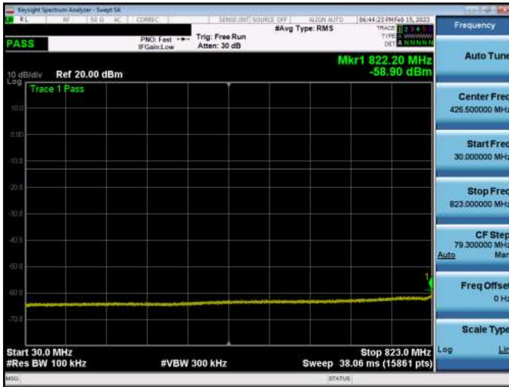
Plot 7-53. Conducted Spurious Plot (LTE Band 5 - 10MHz QPSK - 1 RB - Low Channel - Sub)
