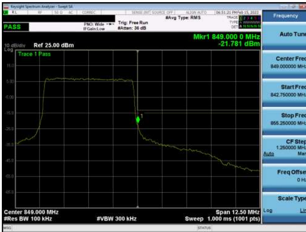
Plot 7-109. Upper Band Edge Plot (LTE Band 5 - 5MHz QPSK – Full RB - Sub)
