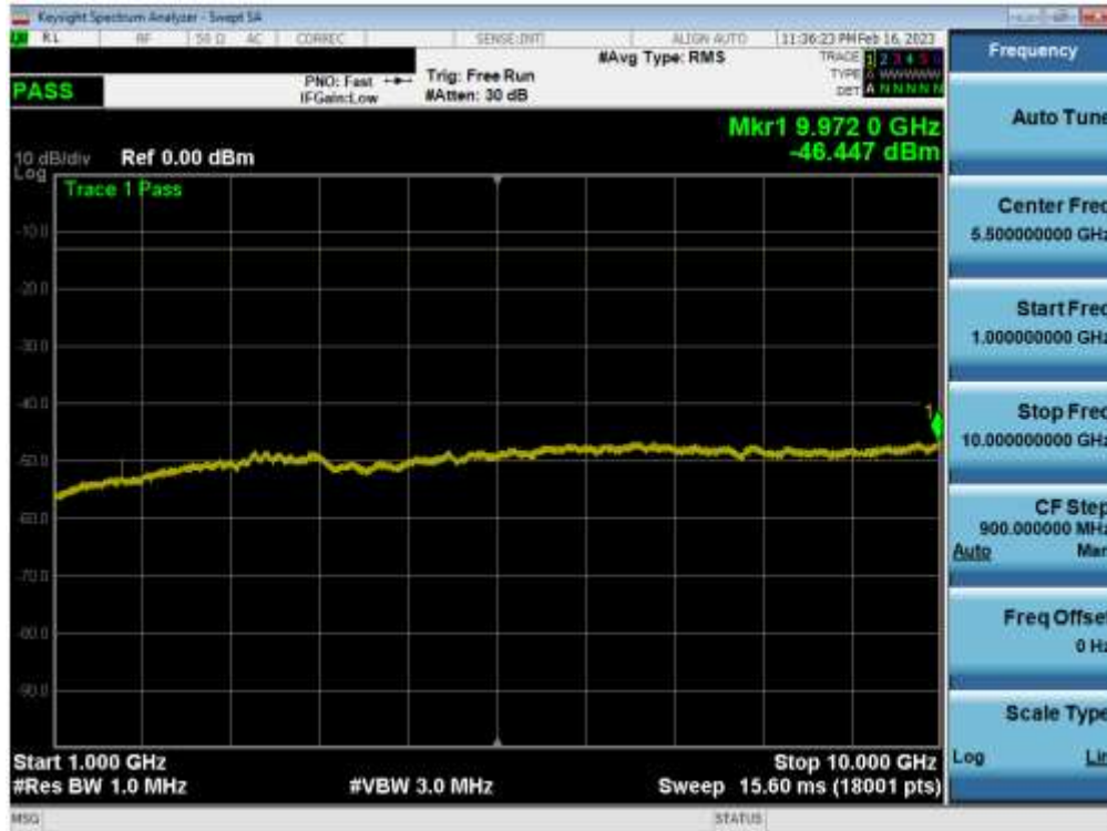
Plot 7-97. Conducted Spurious Plot (WCDMA Ch. 4233 – Main1)
