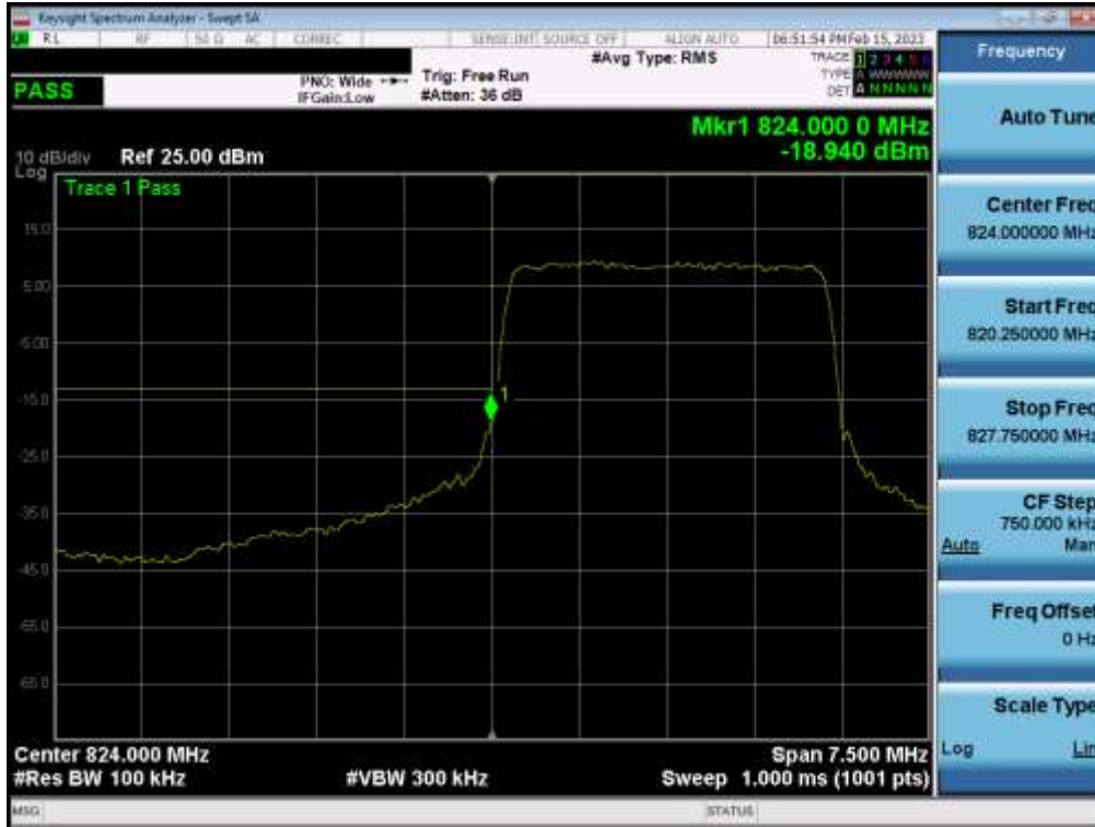
Plot 7-110. Lower Band Edge Plot (LTE Band 5 - 3MHz QPSK – Full RB - Sub)
