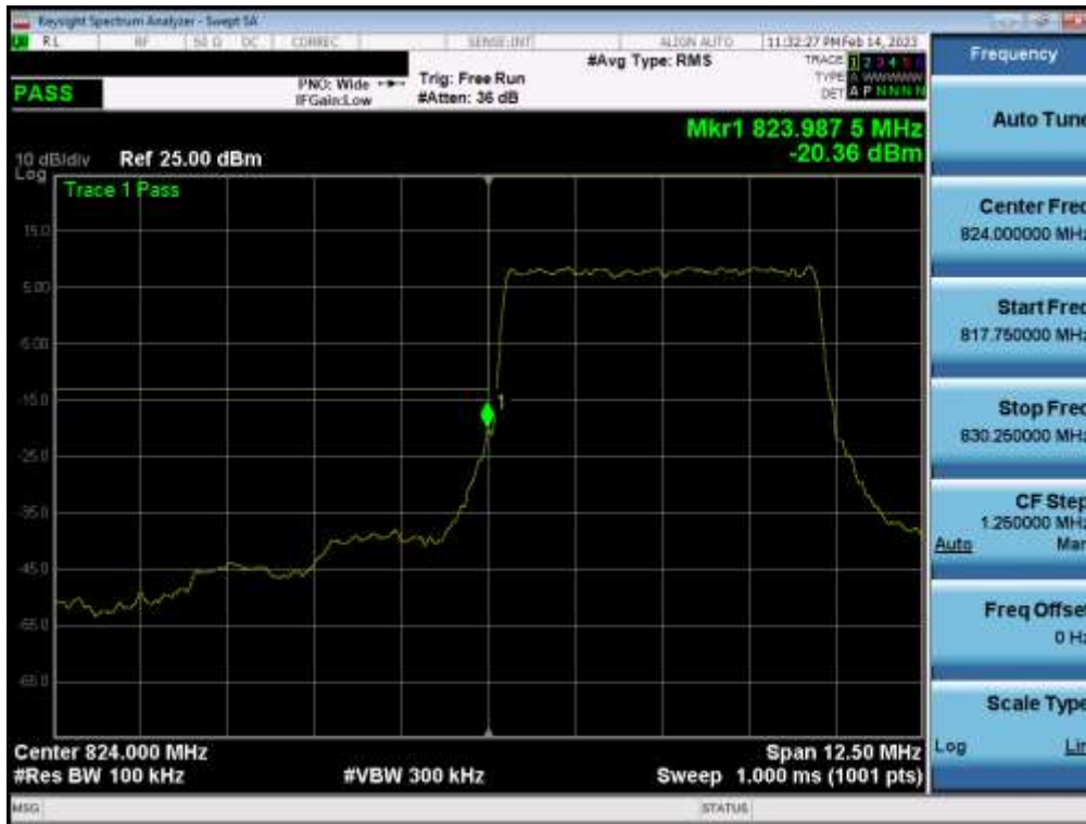
Plot 7-120. Lower Band Edge Plot (NR Band n5 – 5.0MHz - Full RB - Main1)
