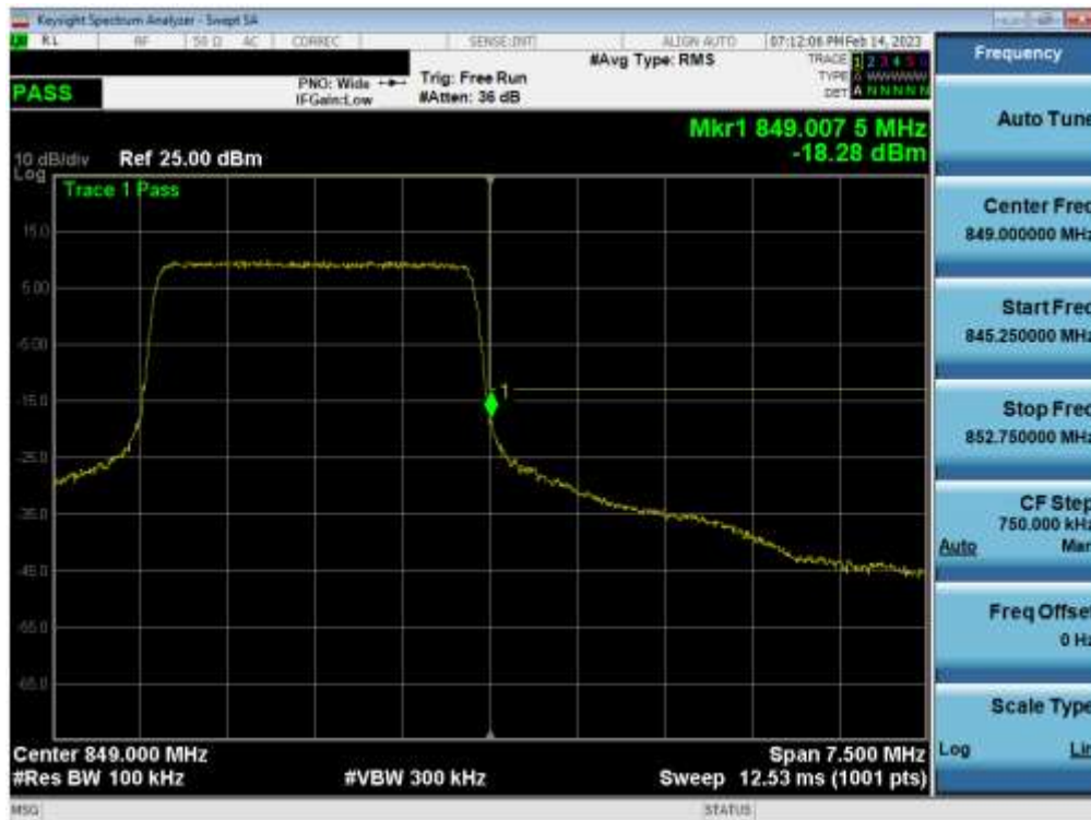
Plot 7-103. Upper Band Edge Plot (LTE Band 5 - 3MHz QPSK – Full RB - Main1)
