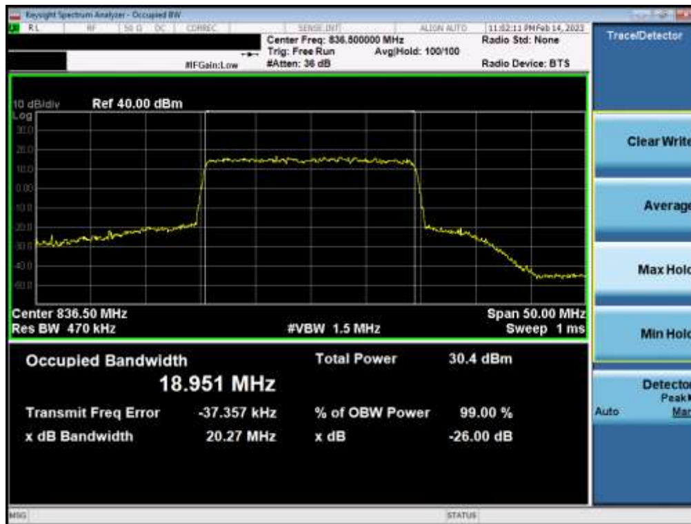
Plot 7-18. Occupied Bandwidth Plot (NR Band n5 - 20MHz QPSK - Full RB - Main1)
