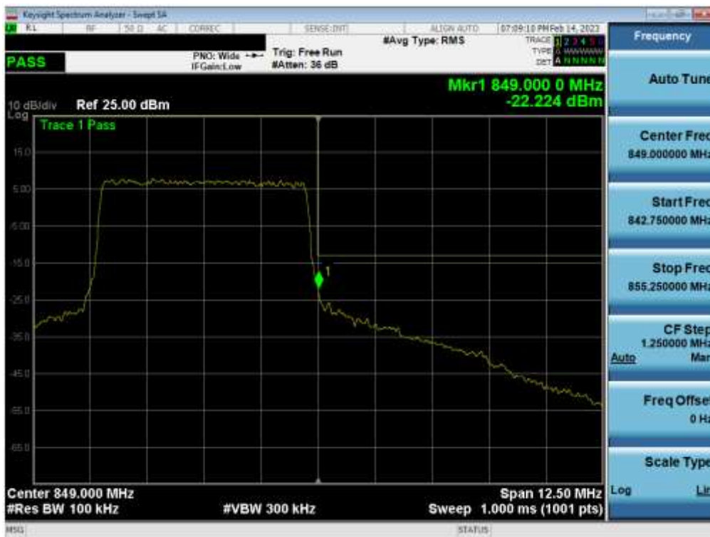
Plot 7-101. Upper Band Edge Plot (LTE Band 5 - 5MHz QPSK – Full RB - Main1)
