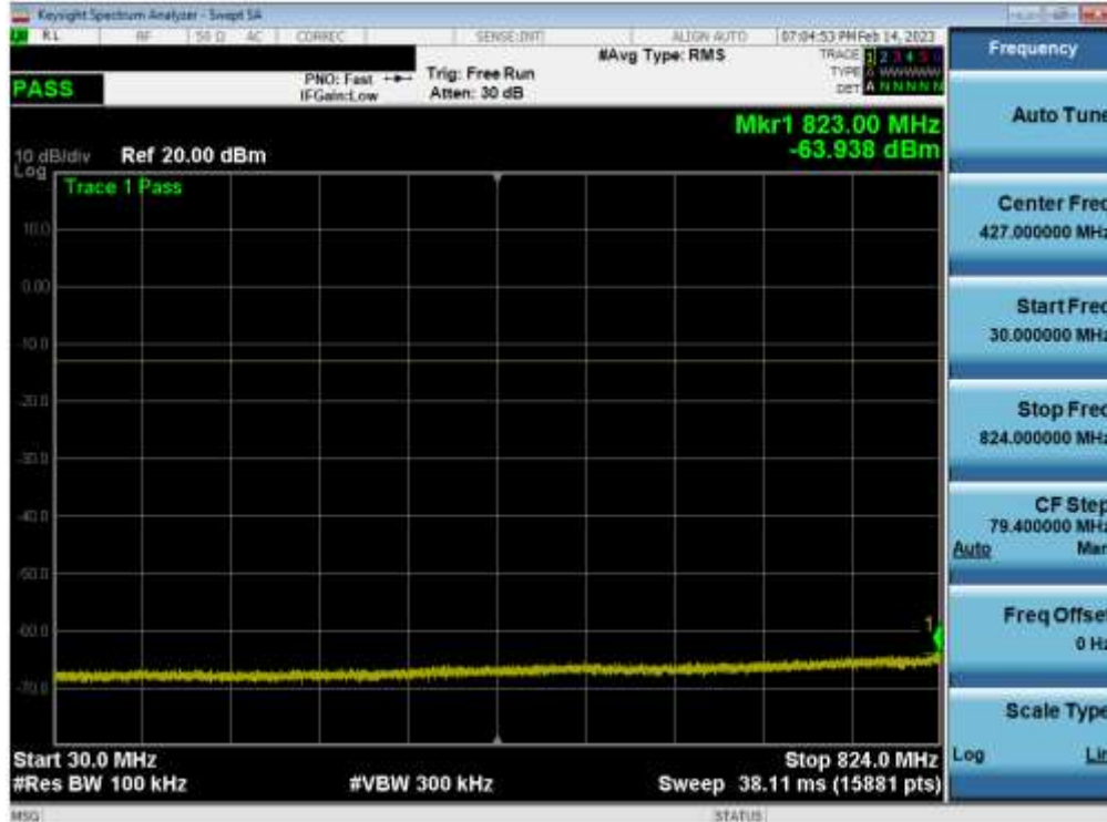
Plot 7-47. Conducted Spurious Plot (LTE Band 5 - 10MHz QPSK - 1 RB - Mid Channel - Main1)
