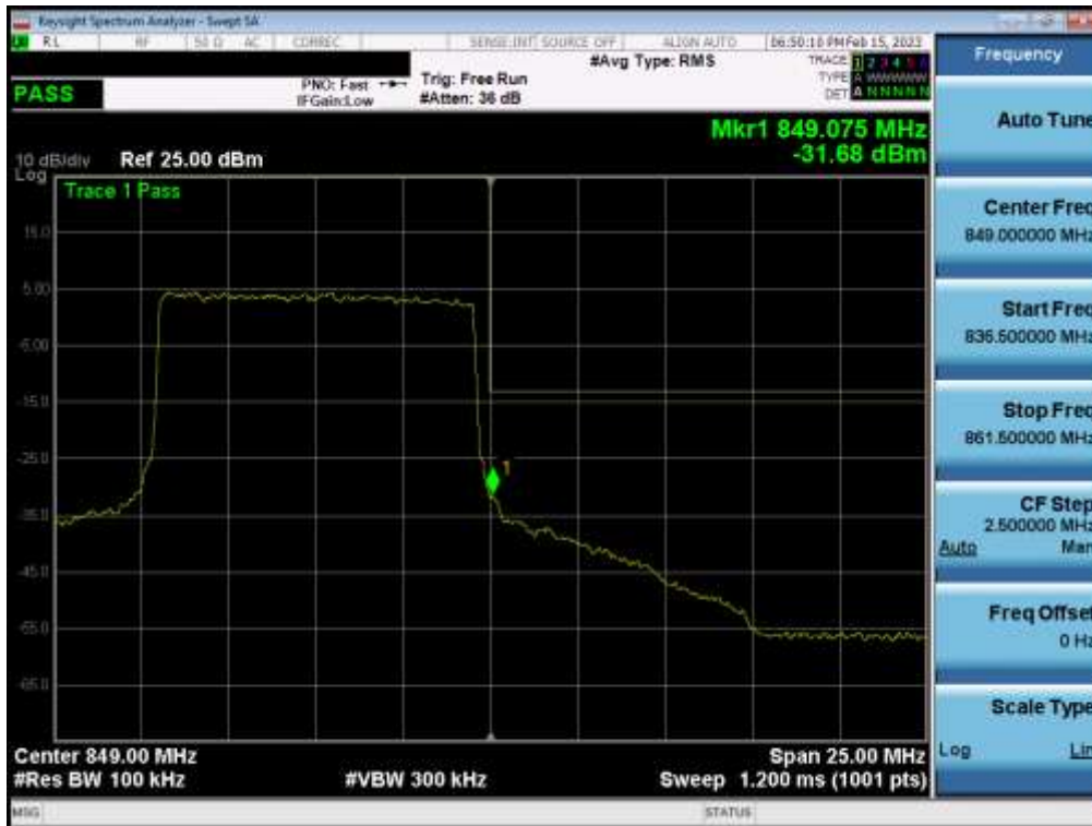
Plot 7-107. Upper Band Edge Plot (LTE Band 5 - 10MHz QPSK – Full RB - Sub)
