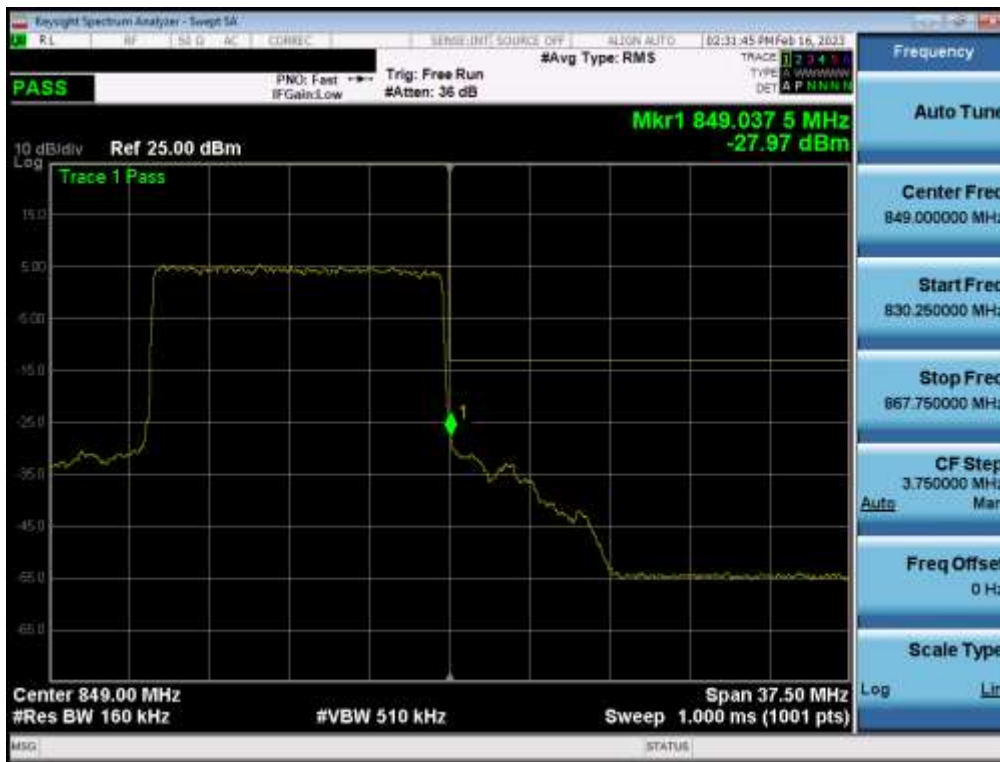
Plot 7-125. Upper Band Edge Plot (NR Band n5 – 15.0MHz - Full RB - Sub)
