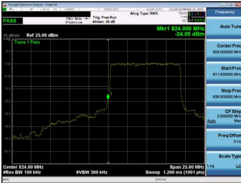
Plot 7-118. Lower Band Edge Plot (NR Band n5 – 10.0MHz - Full RB - Main1)
