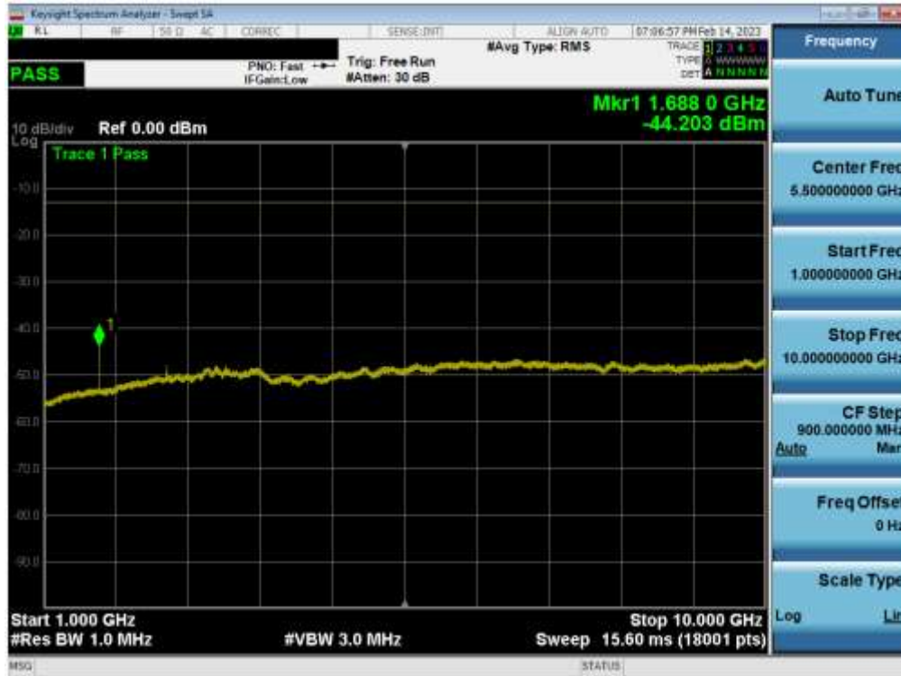
Plot 7-52. Conducted Spurious Plot (LTE Band 5 - 10MHz QPSK - 1 RB - High Channel - Main1)
