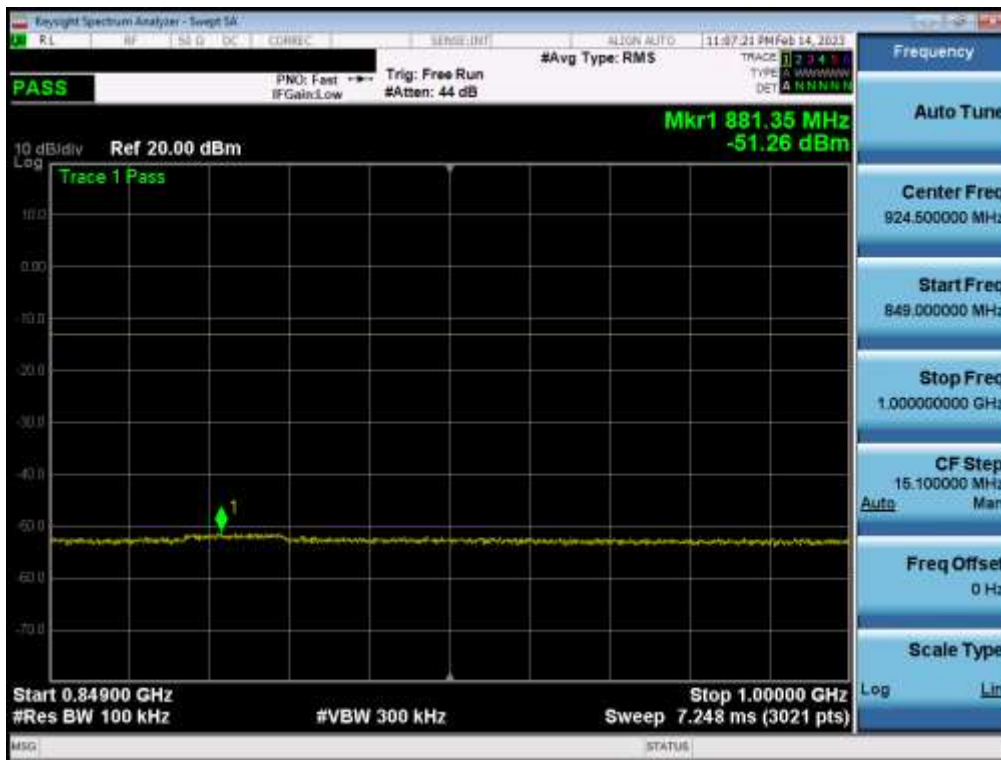
Plot 7-69. Conducted Spurious Plot (NR Band n5 - 20.0MHz - 1 RB - High Channel - Main1)
