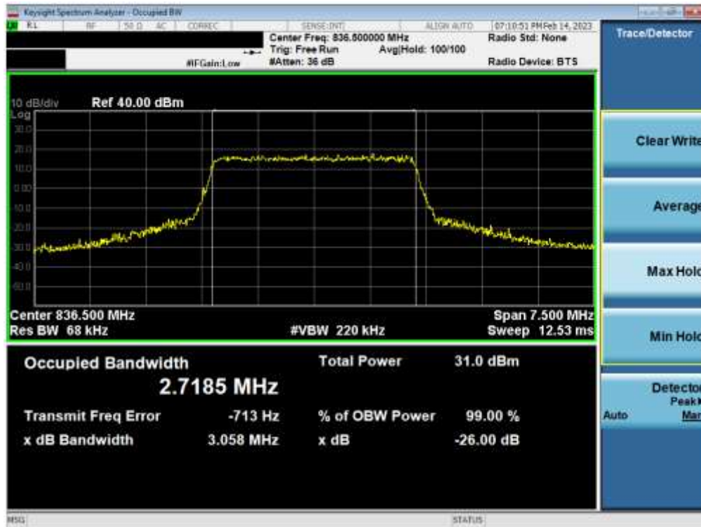
Plot 7-6. Occupied Bandwidth Plot (LTE Band 5 - 3MHz 16-QAM - Full RB - Main1)
