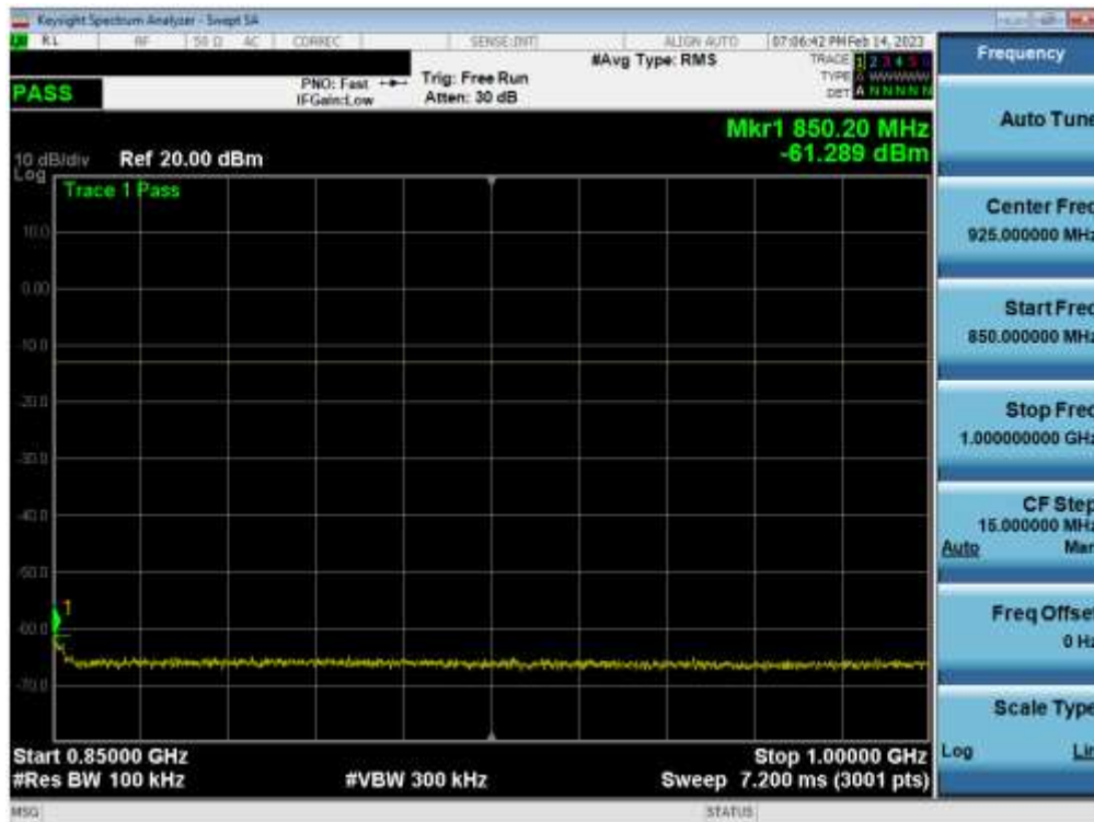
Plot 7-51. Conducted Spurious Plot (LTE Band 5 - 10MHz QPSK - 1 RB - High Channel - Main1)
