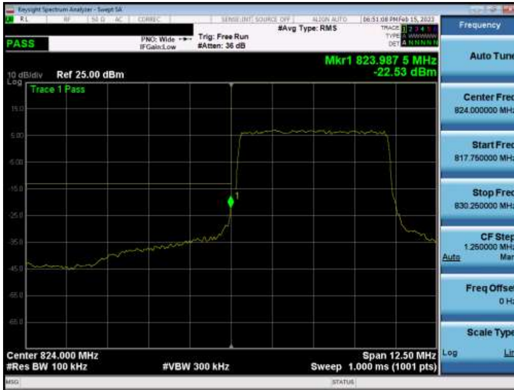
Plot 7-108. Lower Band Edge Plot (LTE Band 5 - 5MHz QPSK – Full RB - Sub)
