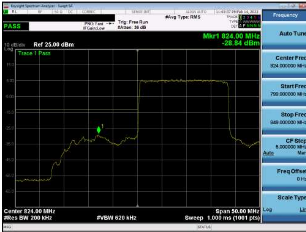
Plot 7-114. Lower Band Edge Plot (NR Band n5 – 20.0MHz - Full RB - Main1)
