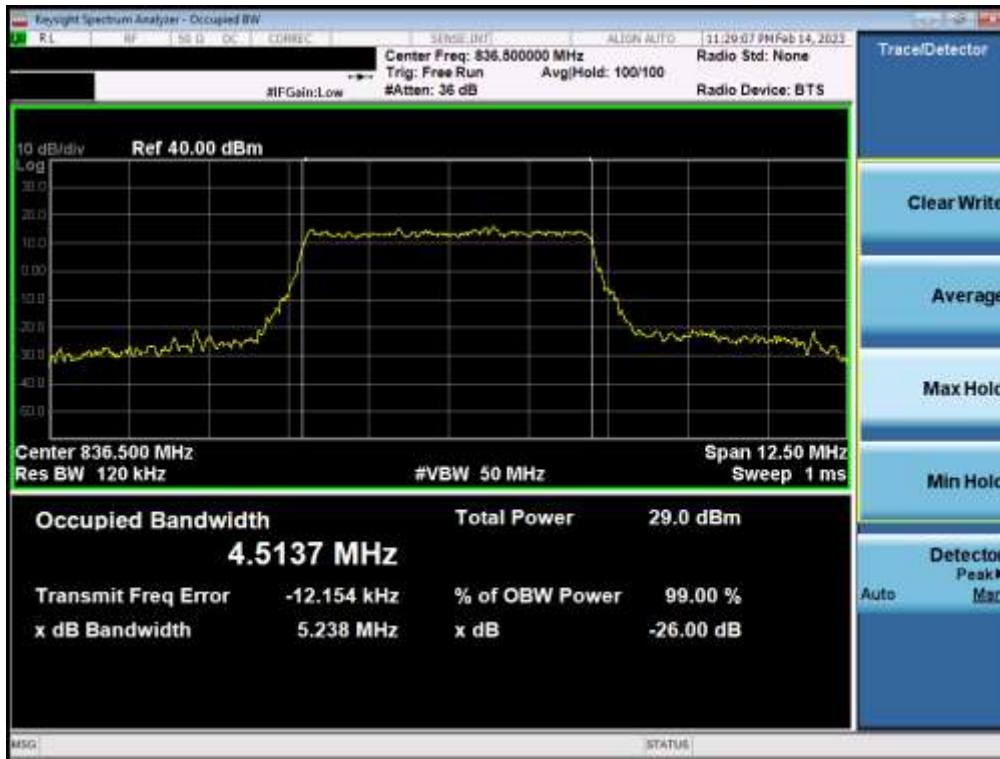
Plot 7-27. Occupied Bandwidth Plot (NR Band n5 - 5MHz QPSK - Full RB - Main1)
