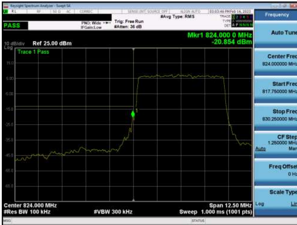
Plot 7-128. Lower Band Edge Plot (NR Band n5 – 5.0MHz - Full RB - Sub)
