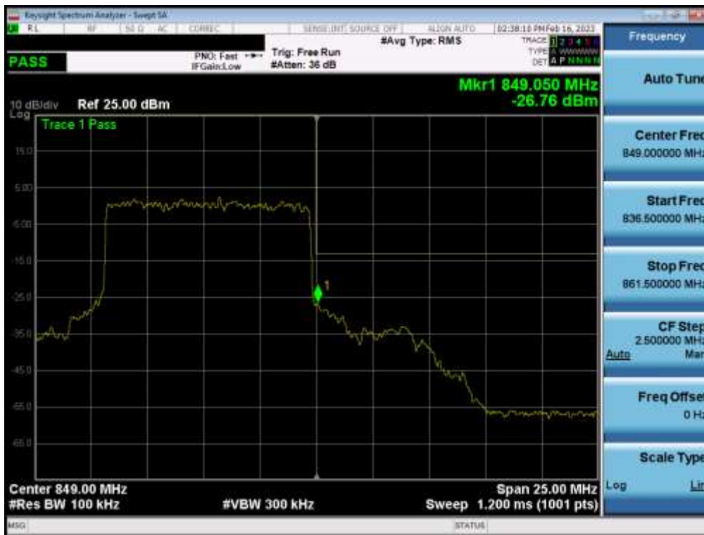
Plot 7-127. Upper Band Edge Plot (NR Band n5 – 10.0MHz - Full RB - Sub)
