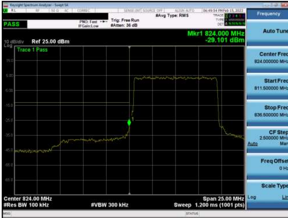
Plot 7-106. Lower Band Edge Plot (LTE Band 5 - 10MHz QPSK – Full RB - Sub)
