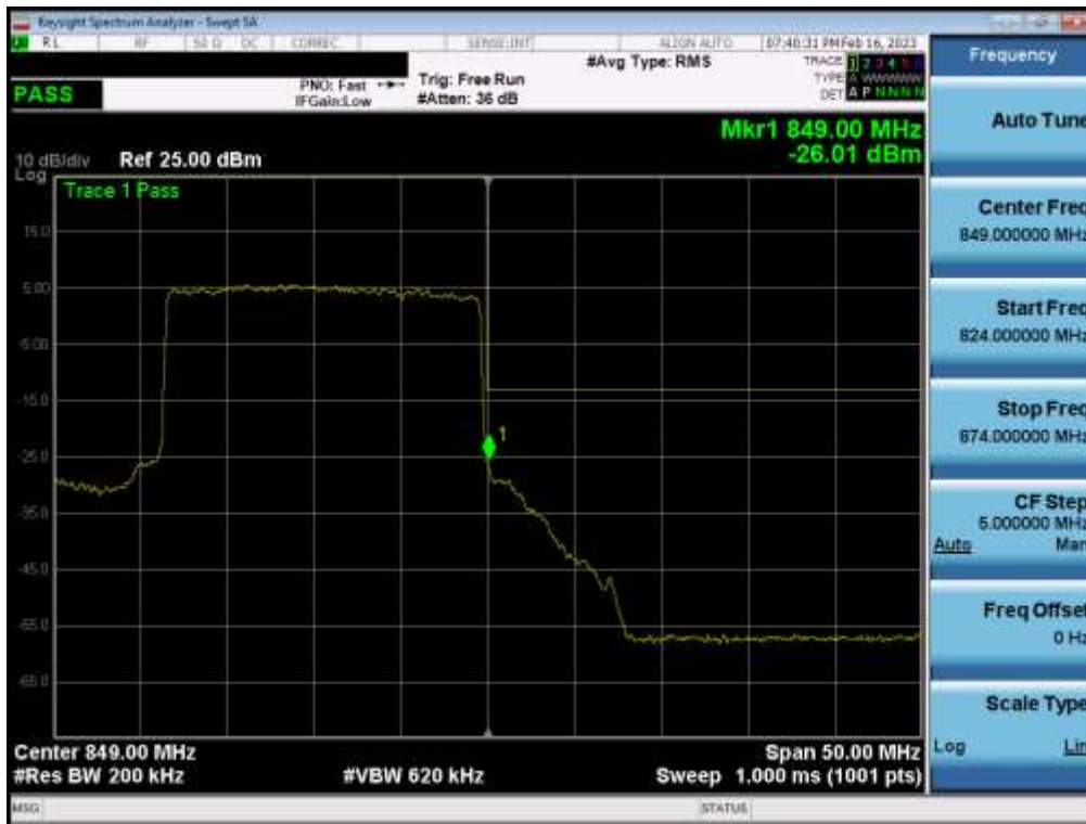
Plot 7-115. Upper Band Edge Plot (NR Band n5 – 20.0MHz - Full RB - Main1)
