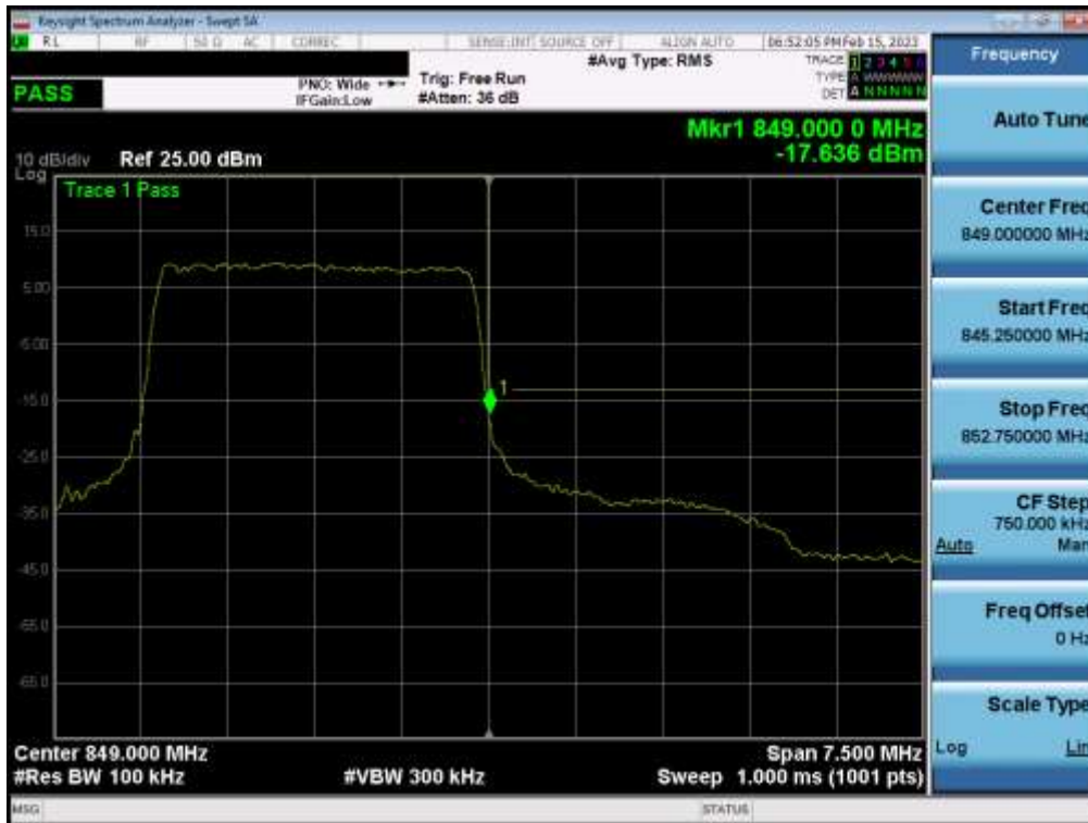
Plot 7-111. Upper Band Edge Plot (LTE Band 5 - 3MHz QPSK – Full RB - Sub)
