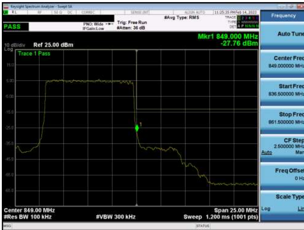
Plot 7-119. Upper Band Edge Plot (NR Band n5 – 10.0MHz - Full RB - Main1)
