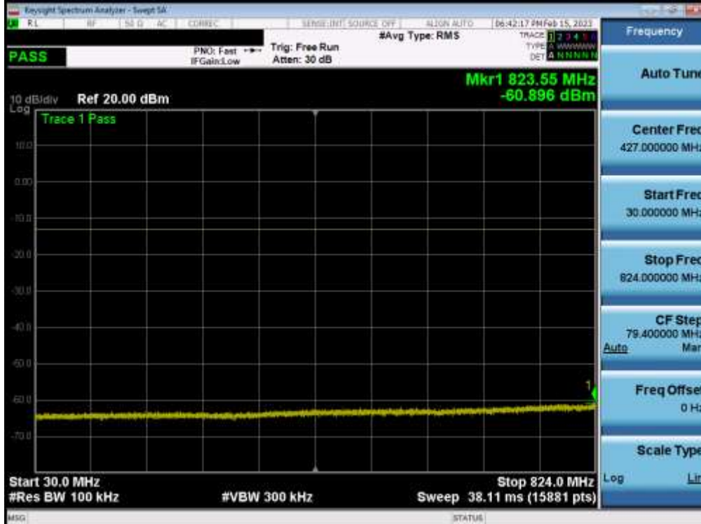
Plot 7-56. Conducted Spurious Plot (LTE Band 5 - 10MHz QPSK - 1 RB - Mid Channel - Sub)
