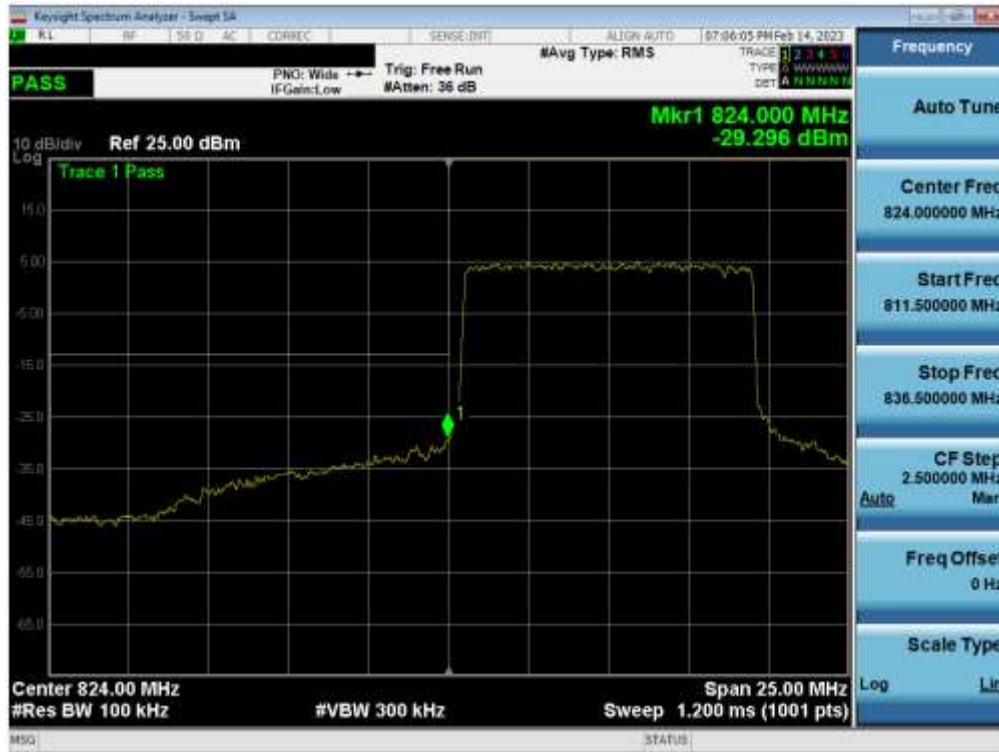
Plot 7-98. Lower Band Edge Plot (LTE Band 5 - 10MHz QPSK – Full RB - Main1)
