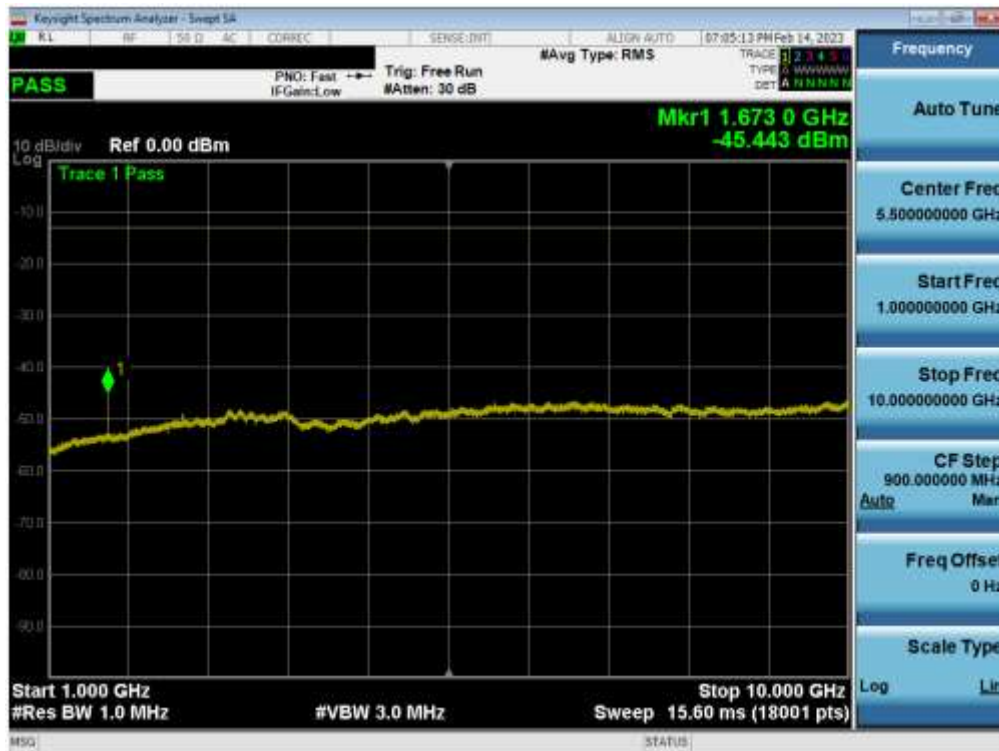
Plot 7-49. Conducted Spurious Plot (LTE Band 5 - 10MHz QPSK - 1 RB - Mid Channel - Main1)
