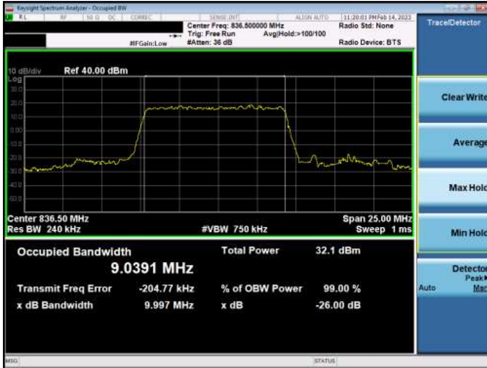
Plot 7-23. Occupied Bandwidth Plot (NR Band n5 - 10MHz \pi/2 BPSK - Full RB - Main1)
