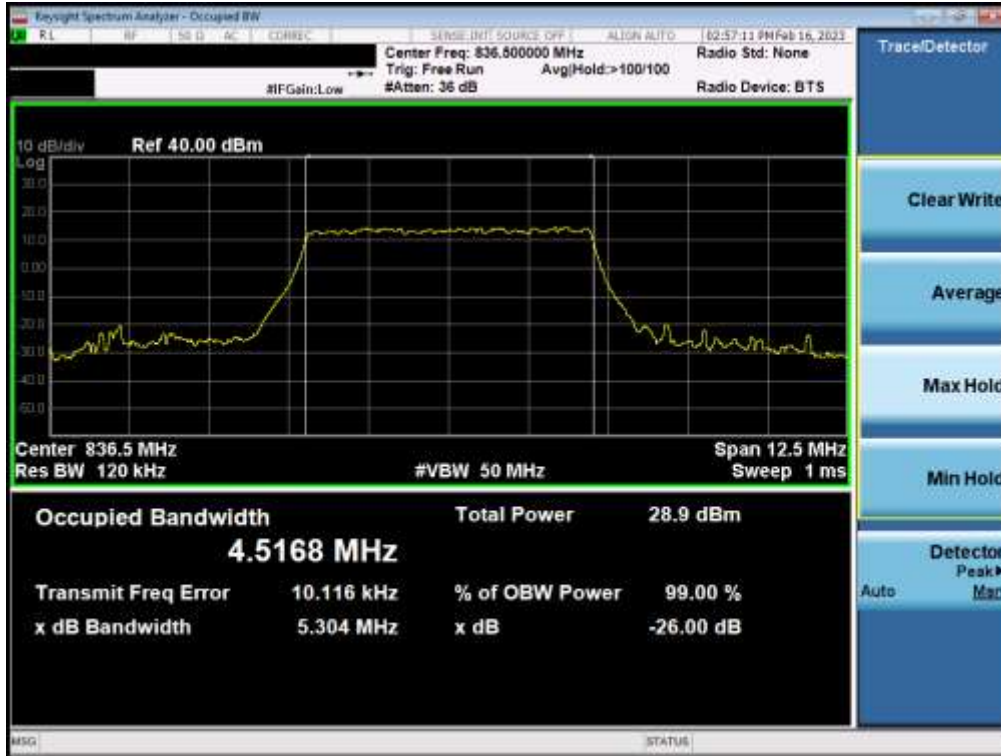
Plot 7-39. Occupied Bandwidth Plot (NR Band n5 - 5MHz QPSK - Full RB - Sub)
