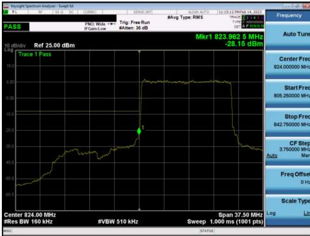
Plot 7-116. Lower Band Edge Plot (NR Band n5 – 15.0MHz - Full RB - Main1)
