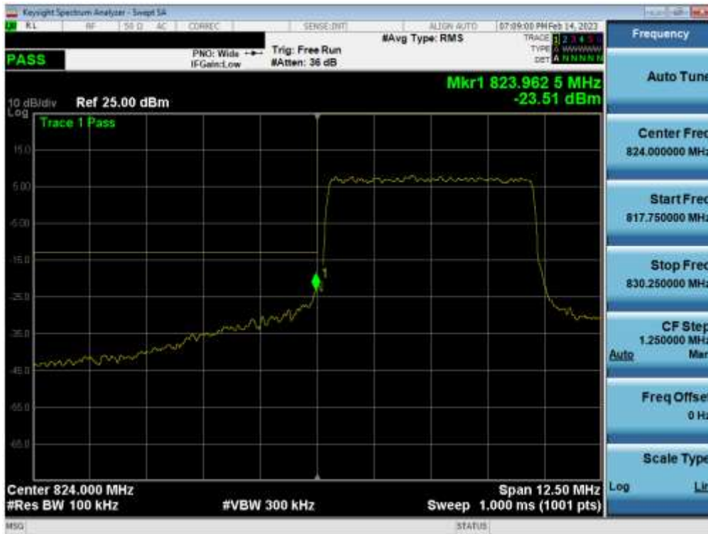
Plot 7-100. Lower Band Edge Plot (LTE Band 5 - 5MHz QPSK – Full RB - Main1)
