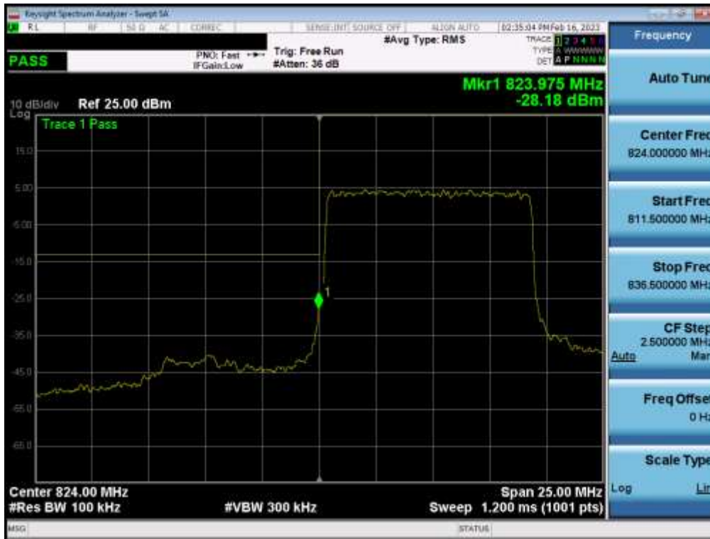
Plot 7-126. Lower Band Edge Plot (NR Band n5 – 10.0MHz - Full RB - Sub)
