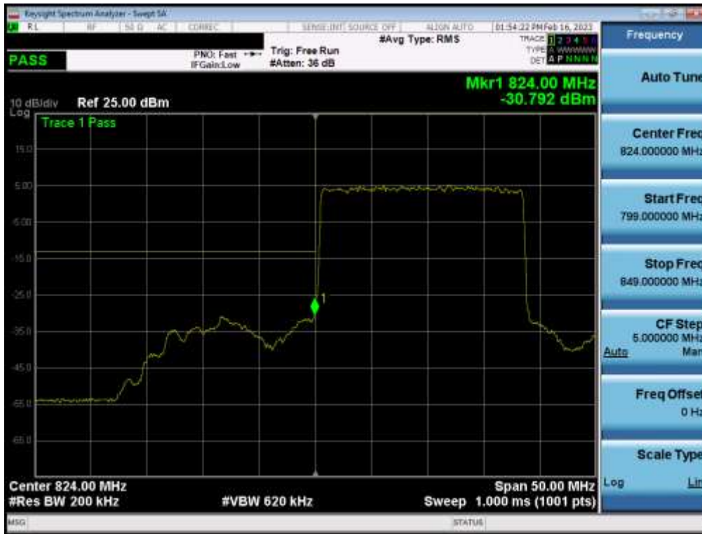
Plot 7-122. Lower Band Edge Plot (NR Band n5 – 20.0MHz - Full RB - Sub)
