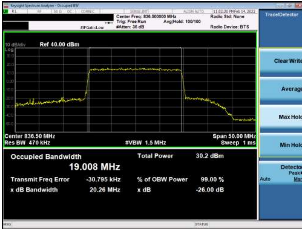
Plot 7-19. Occupied Bandwidth Plot (NR Band n5 - 20MHz 16-QAM - Full RB - Main1)
