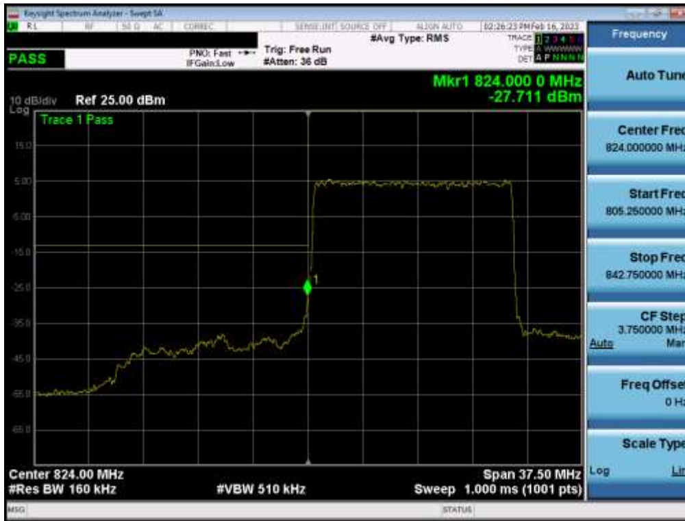
Plot 7-124. Lower Band Edge Plot (NR Band n5 – 15.0MHz - Full RB - Sub)
