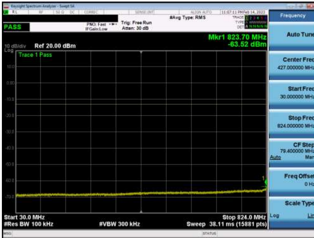
Plot 7-68. Conducted Spurious Plot (NR Band n5 - 20.0MHz - 1 RB - High Channel - Main1)
