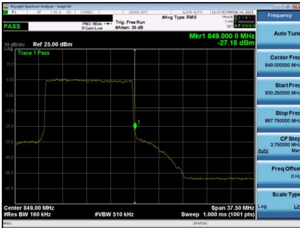
Plot 7-117. Upper Band Edge Plot (NR Band n5 – 15.0MHz - Full RB - Main1)
