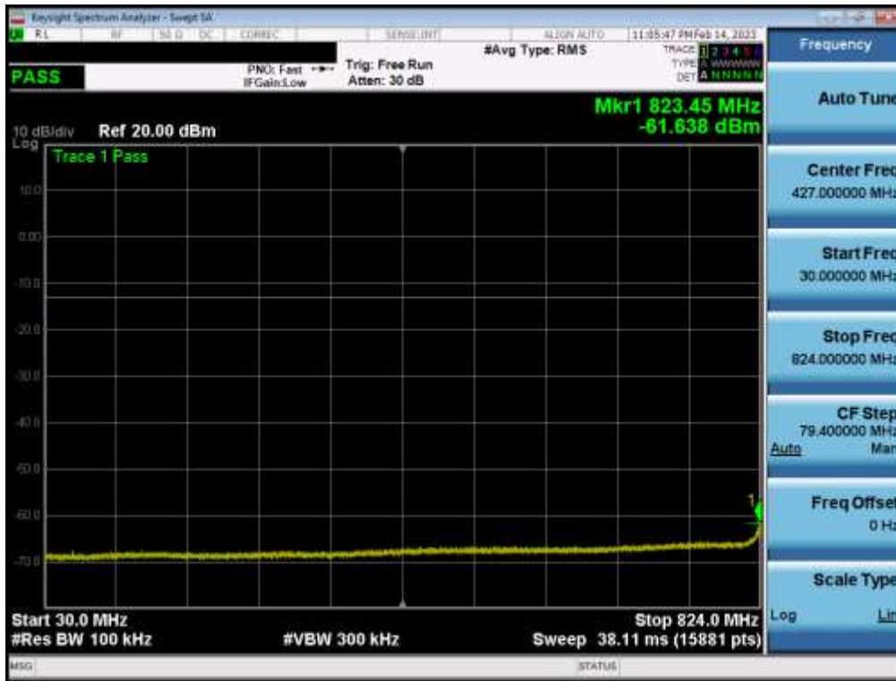
Plot 7-62. Conducted Spurious Plot (NR Band n5 - 20.0MHz - 1 RB - Low Channel - Main1)
