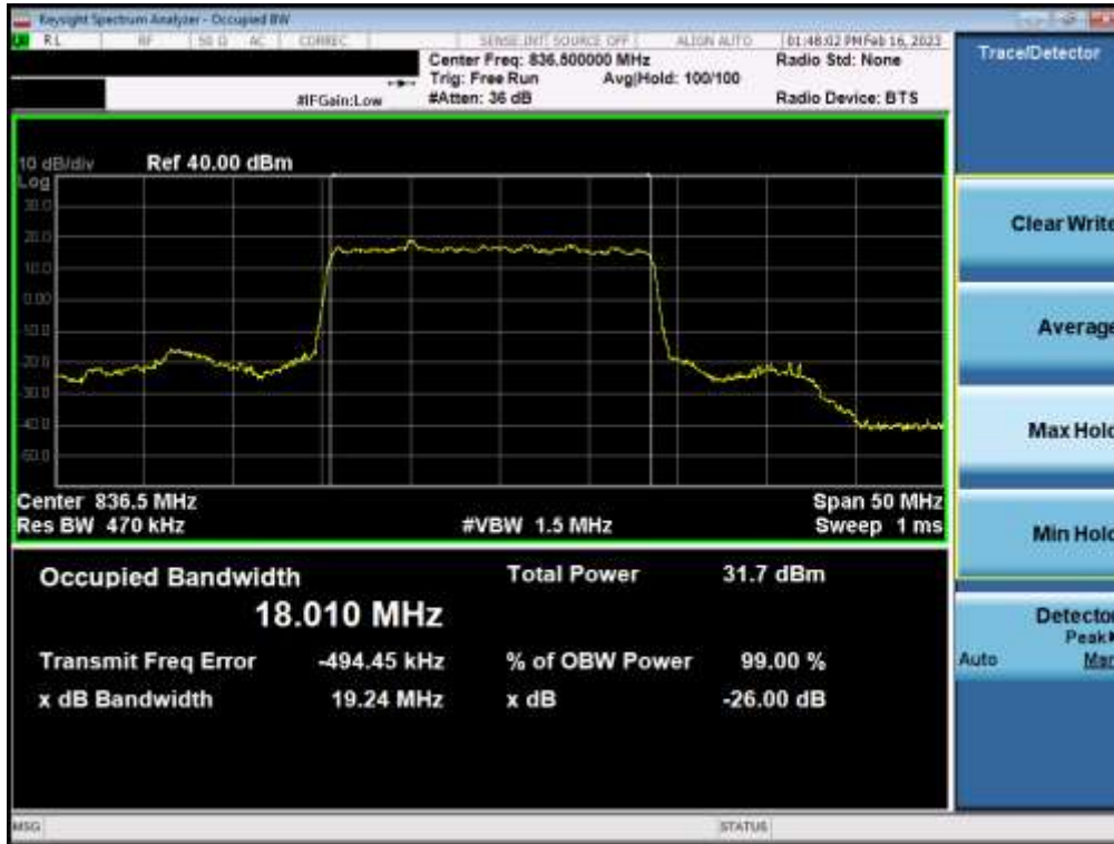
Plot 7-29. Occupied Bandwidth Plot (NR Band n5 - 20MHz \pi/2 BPSK - Full RB - Sub)
