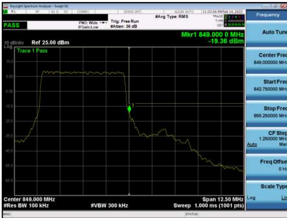
Plot 7-121. Upper Band Edge Plot (NR Band n5 – 5.0MHz - Full RB - Main1)
