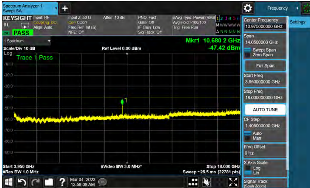
Plot 7-19. Conducted Spurious Plot (LTE Band 48 - 20MHz QPSK - Low Channel - Main Ant)
