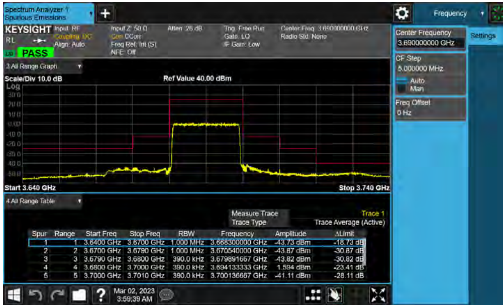
Plot 7-55. Channel - Sub Ant Edge Plot (LTE Band 48 - 20MHz QPSK - High Channel - Sub Ant)
