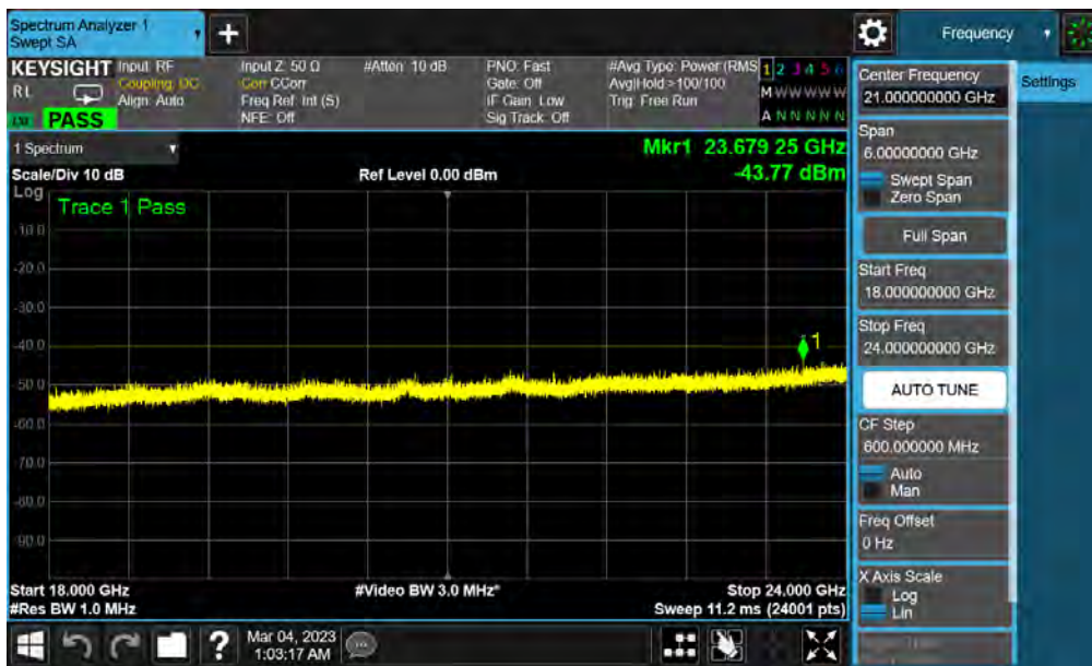
Plot 7-24. Conducted Spurious Plot (LTE Band 48 - 20MHz QPSK - Mid Channel - Main Ant)
