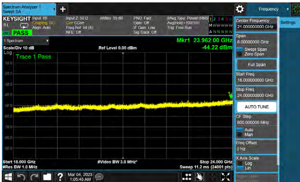
Plot 7-20. Conducted Spurious Plot (LTE Band 48 - 20MHz QPSK - Low Channel - Main Ant)
