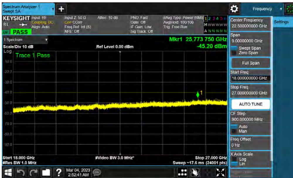
Plot 7-40. Conducted Spurious Plot (LTE Band 48 - 20MHz QPSK - High Channel - Sub Ant)
