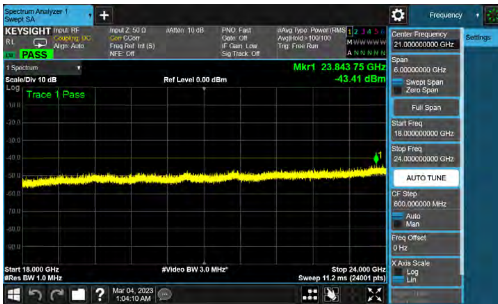
Plot 7-28. Conducted Spurious Plot (LTE Band 48 - 20MHz QPSK - High Channel - Main Ant)
