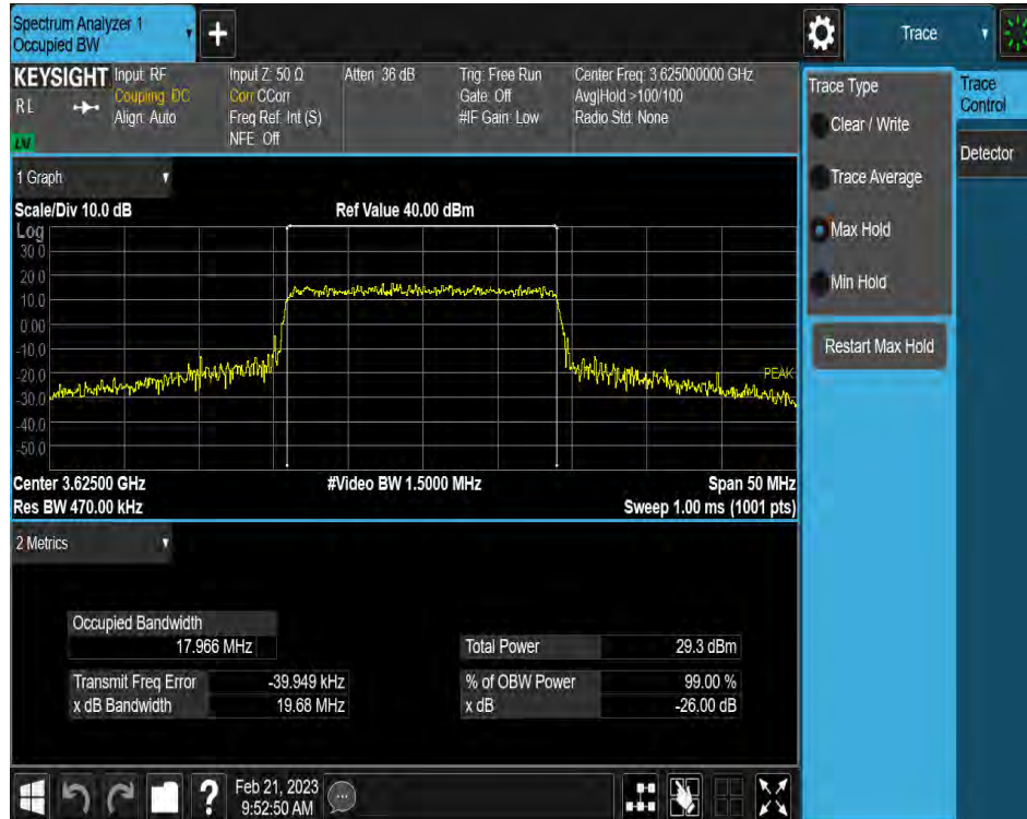
Plot 7-2. Occupied Bandwidth Plot (LTE Band 48 - 20MHz 16-QAM - Full RB Configuration - Main Ant)
