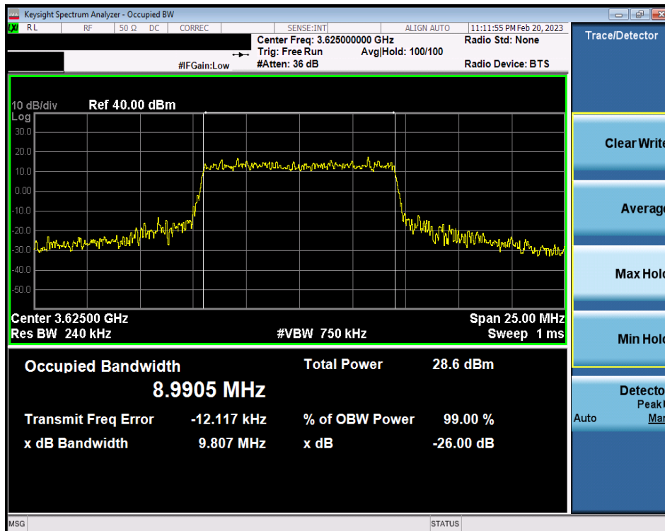
Plot 7-6. Occupied Bandwidth Plot (LTE Band 48 - 10MHz 16-QAM - Full RB Configuration - Main Ant)
