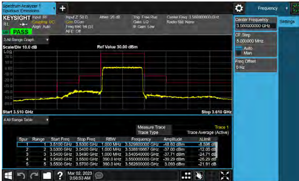
Plot 7-53. Channel - Sub Ant Edge Plot (LTE Band 48 - 20MHz QPSK - Low Channel - Sub Ant)
