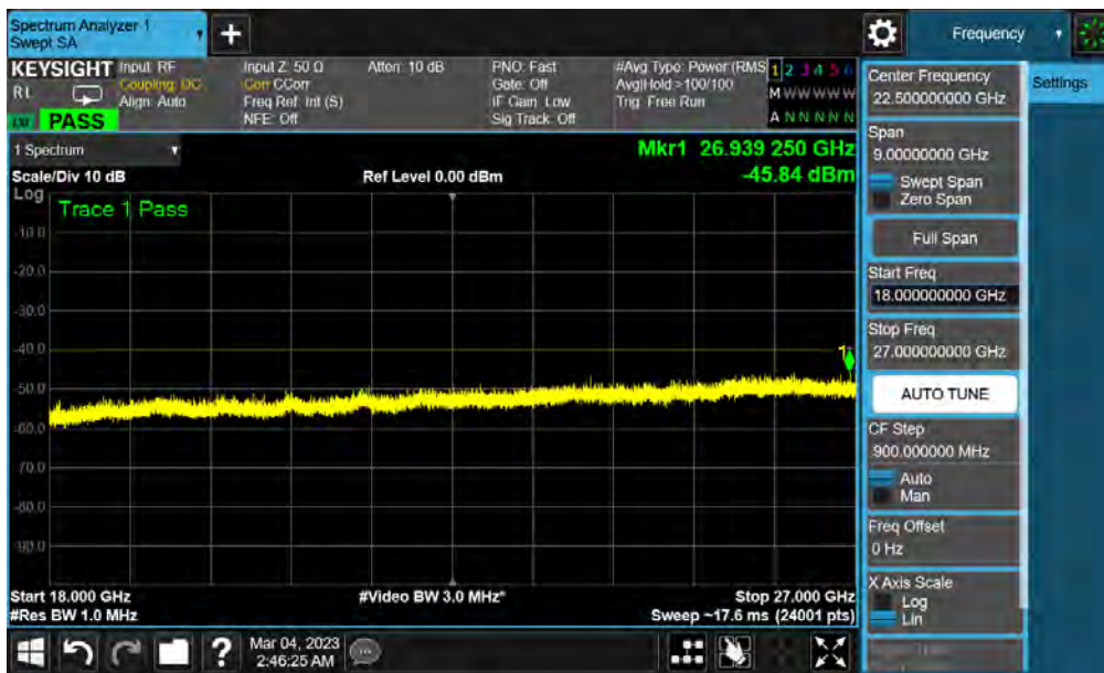
Plot 7-36. Conducted Spurious Plot (LTE Band 48 - 20MHz QPSK - Mid Channel - Sub Ant)
