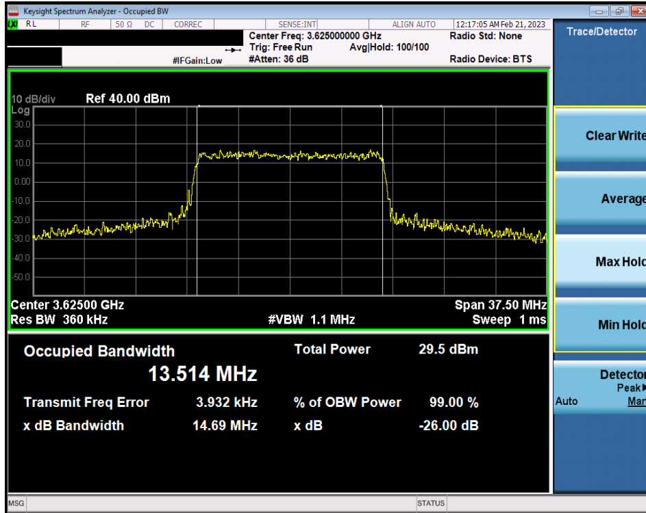
Plot 7-11. Occupied Bandwidth Plot (LTE Band 48 - 15MHz QPSK - Full RB Configuration - Sub Ant)
