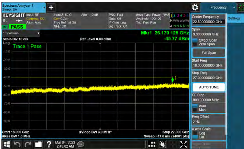
Plot 7-32. Conducted Spurious Plot (LTE Band 48 - 20MHz QPSK - Low Channel - Sub Ant)
