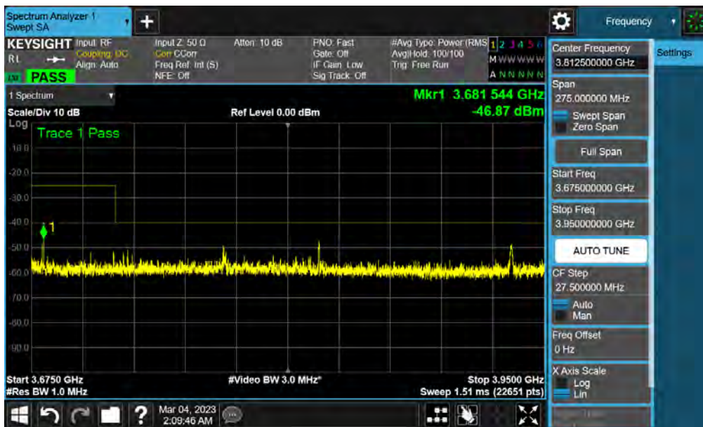
Plot 7-22. Conducted Spurious Plot (LTE Band 48 - 20MHz QPSK - Mid Channel - Main Ant)
