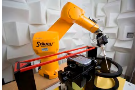
Figure 4-3 SPEAG Robotic System
