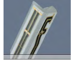
Figure 4-1 E-field Free-space Probe
