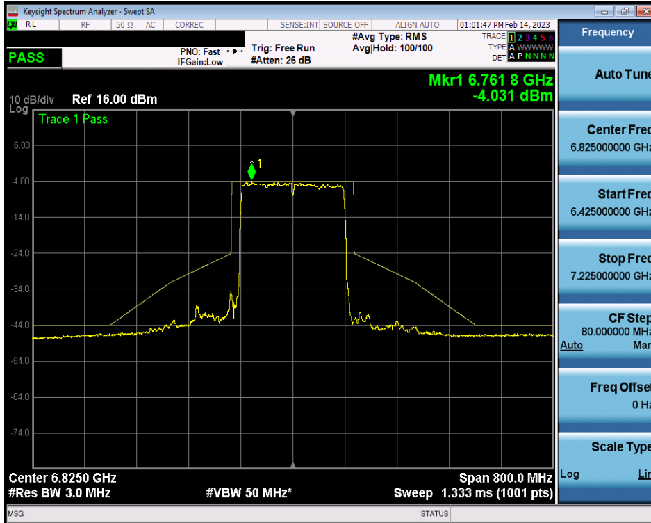
Plot 7-471. In-Band Emission Plot MIMO ANT2 (160MHz BW 802.11ax (Full Tone) (UNII Band 7) – Ch. 175)
