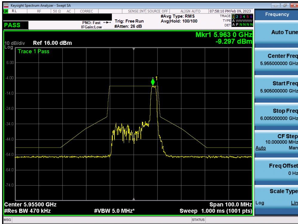
Plot 7-401. In-Band Emission Plot MIMO ANT2 (20MHz BW 802.11ax (26 Tones) UNII Band 5) – Ch. 1
