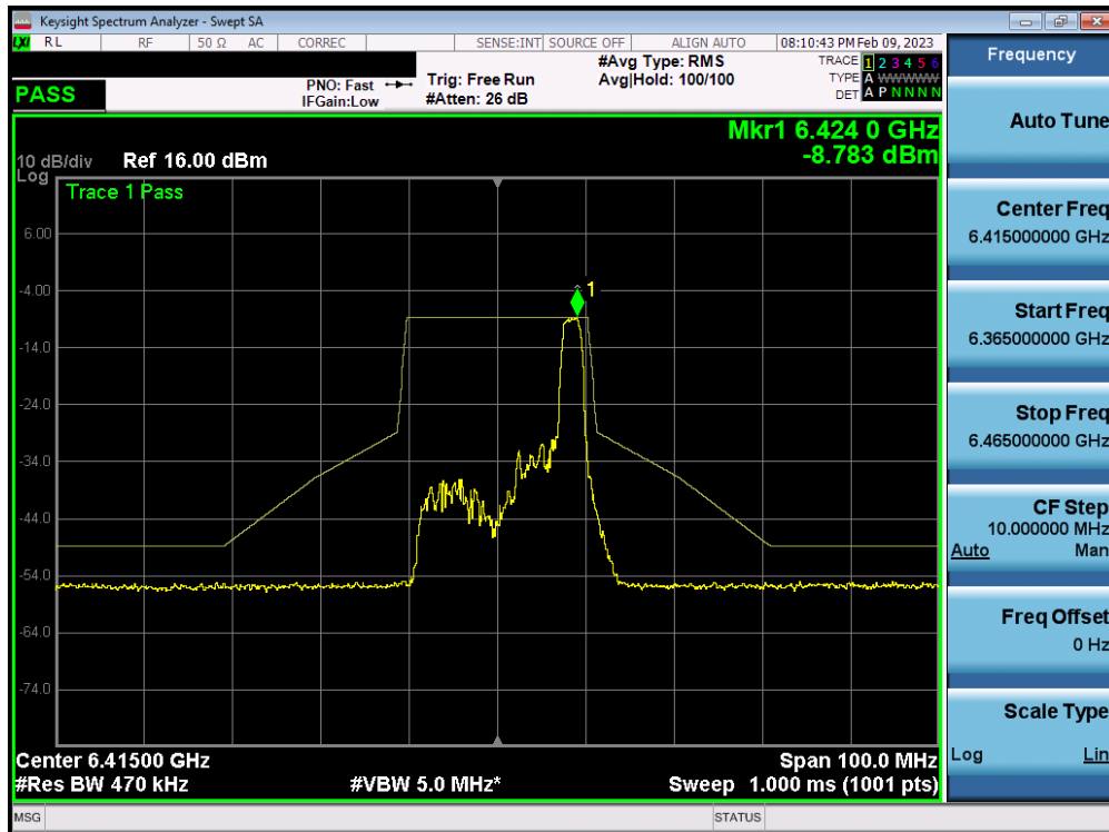
Plot 7-403. In-Band Emission Plot MIMO ANT2 (20MHz BW 802.11ax (26 Tones) UNII Band 5) – Ch. 93)
