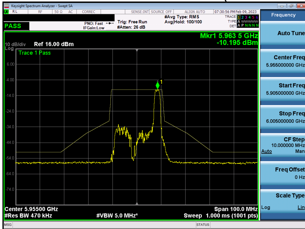
Plot 7-321. In-Band Emission Plot MIMO ANT1 (20MHz BW 802.11ax (26 Tones) UNII Band 5) – Ch. 1
