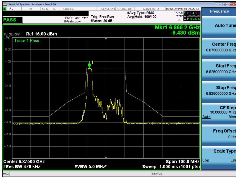
Plot 7-423. In-Band Emission Plot MIMO ANT2 (20MHz BW 802.11ax (26 Tones) (UNII Band 7) – Ch. 185)
