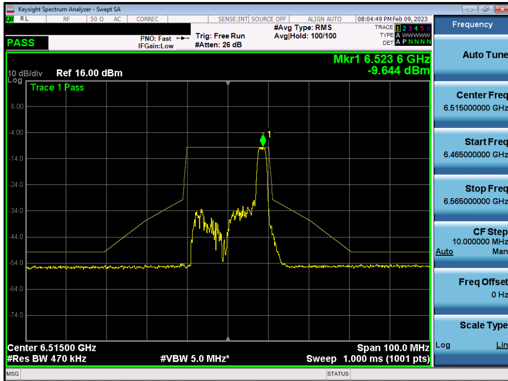
Plot 7-415. In-Band Emission Plot MIMO ANT2 (20MHz BW 802.11ax (26 Tones) (UNII Band 6) – Ch. 113)
