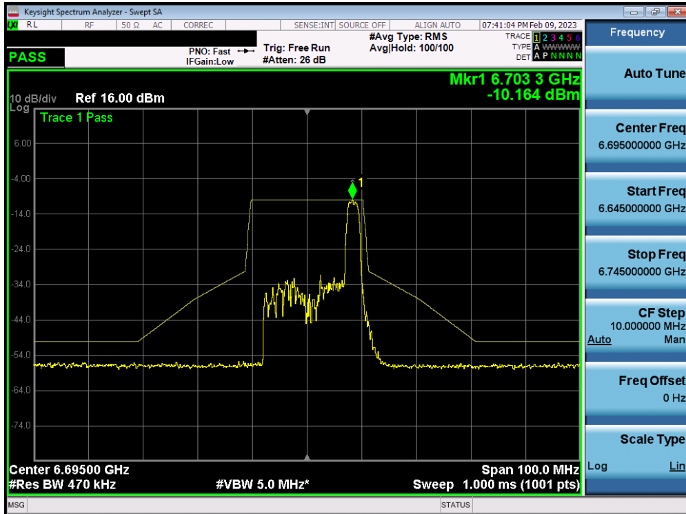
Plot 7-342. In-Band Emission Plot MIMO ANT1 (20MHz BW 802.11ax (26 Tones) (UNII Band 7) – Ch. 149)
