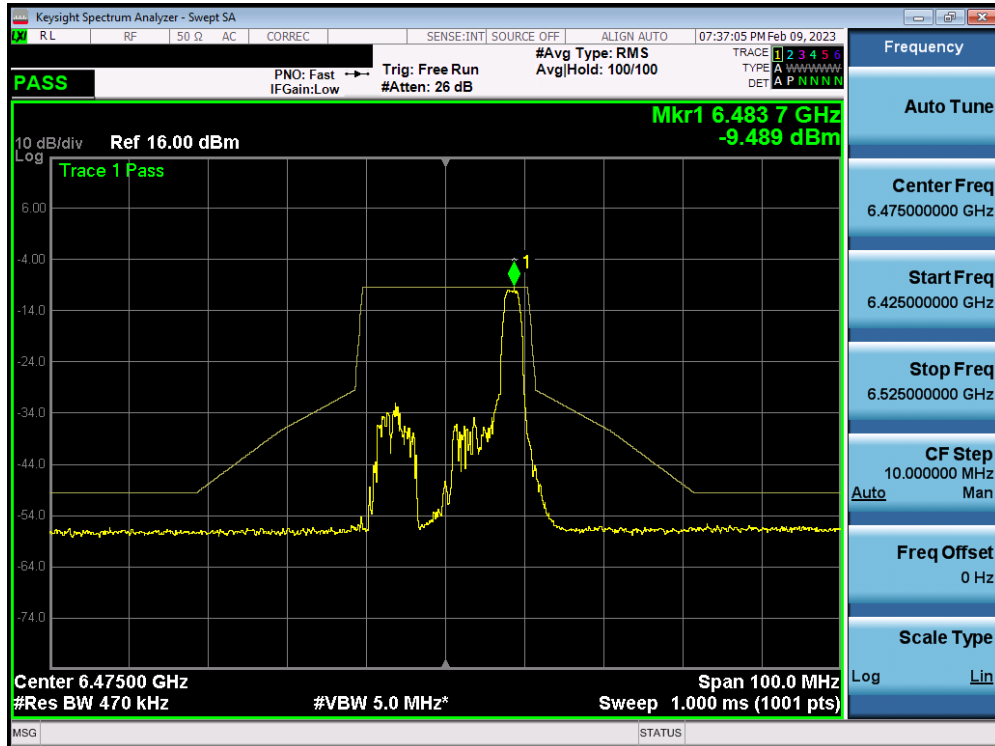
Plot 7-334. In-Band Emission Plot MIMO ANT1 (20MHz BW 802.11ax (26 Tones) (UNII Band 6) – Ch. 105)
