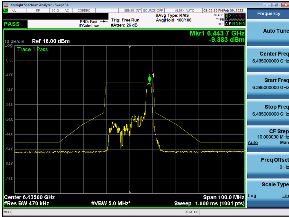
Plot 7-413. In-Band Emission Plot MIMO ANT2 (20MHz BW 802.11ax (26 Tones) (UNII Band 6) – Ch. 97)
