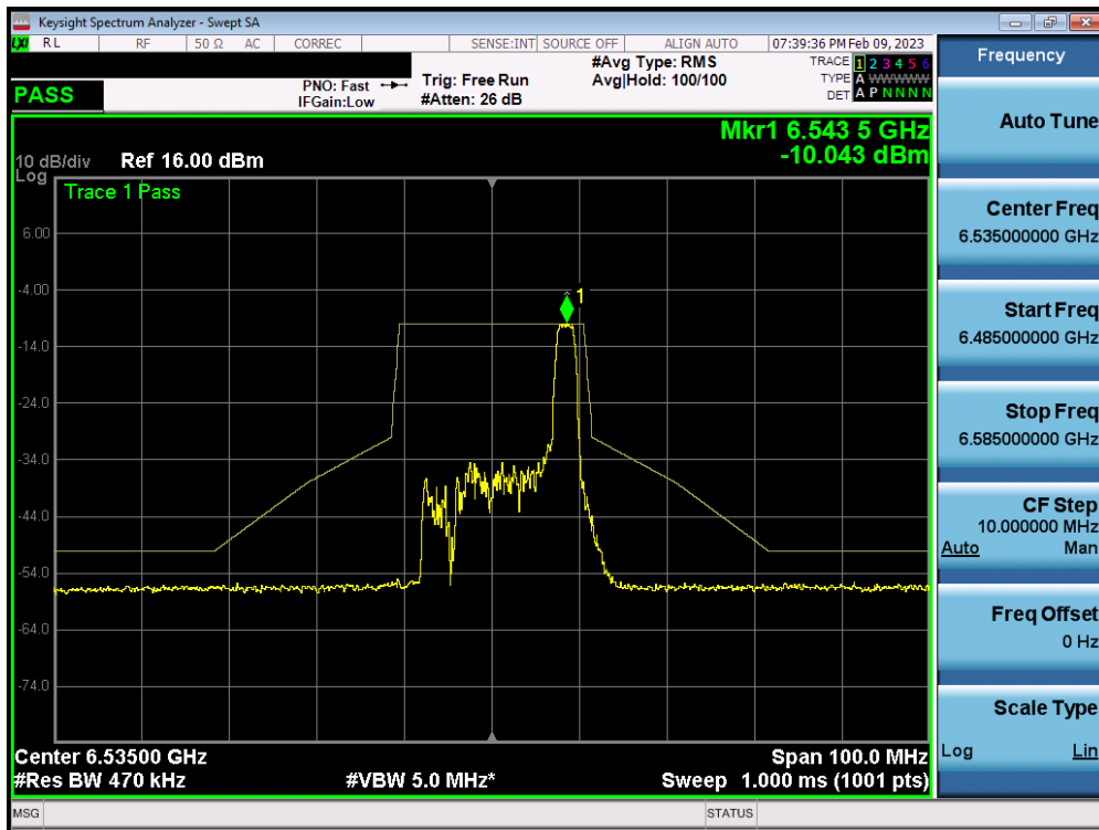
Plot 7-341. In-Band Emission Plot MIMO ANT1 (20MHz BW 802.11ax (26 Tones) (UNII Band 7) – Ch. 117)
