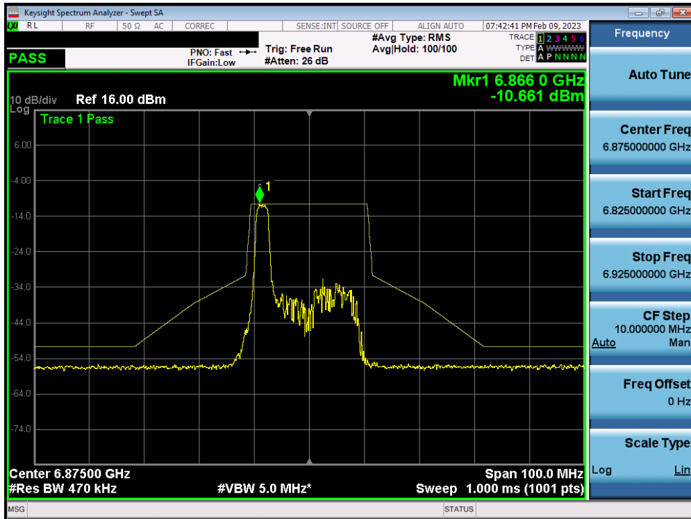
Plot 7-343. In-Band Emission Plot MIMO ANT1 (20MHz BW 802.11ax (26 Tones) (UNII Band 7) – Ch. 185)
