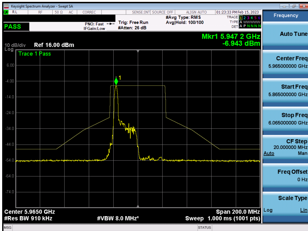
Plot 7-324. In-Band Emission Plot MIMO ANT1 (40MHz BW 802.11ax (26 Tones) (UNII Band 5) – Ch. 3)
