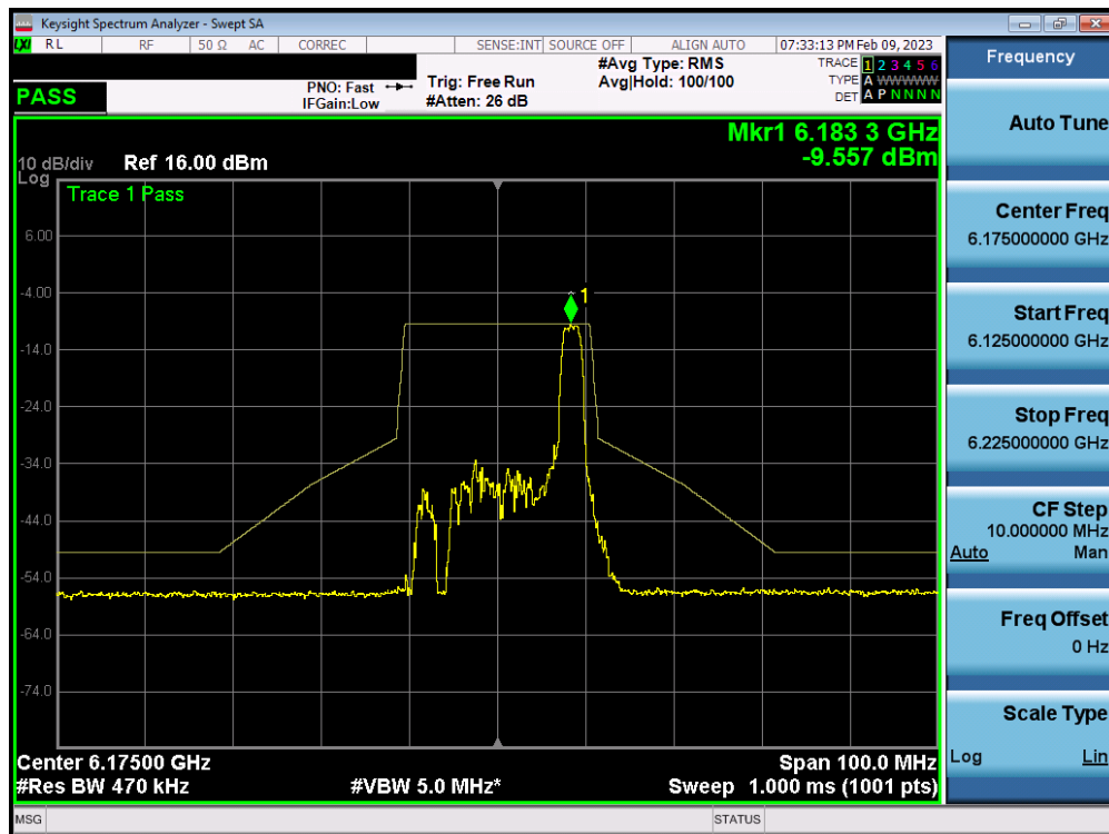
Plot 7-322. In-Band Emission Plot MIMO ANT1 (20MHz BW 802.11ax (26 Tones) (UNII Band 5) – Ch. 45)
