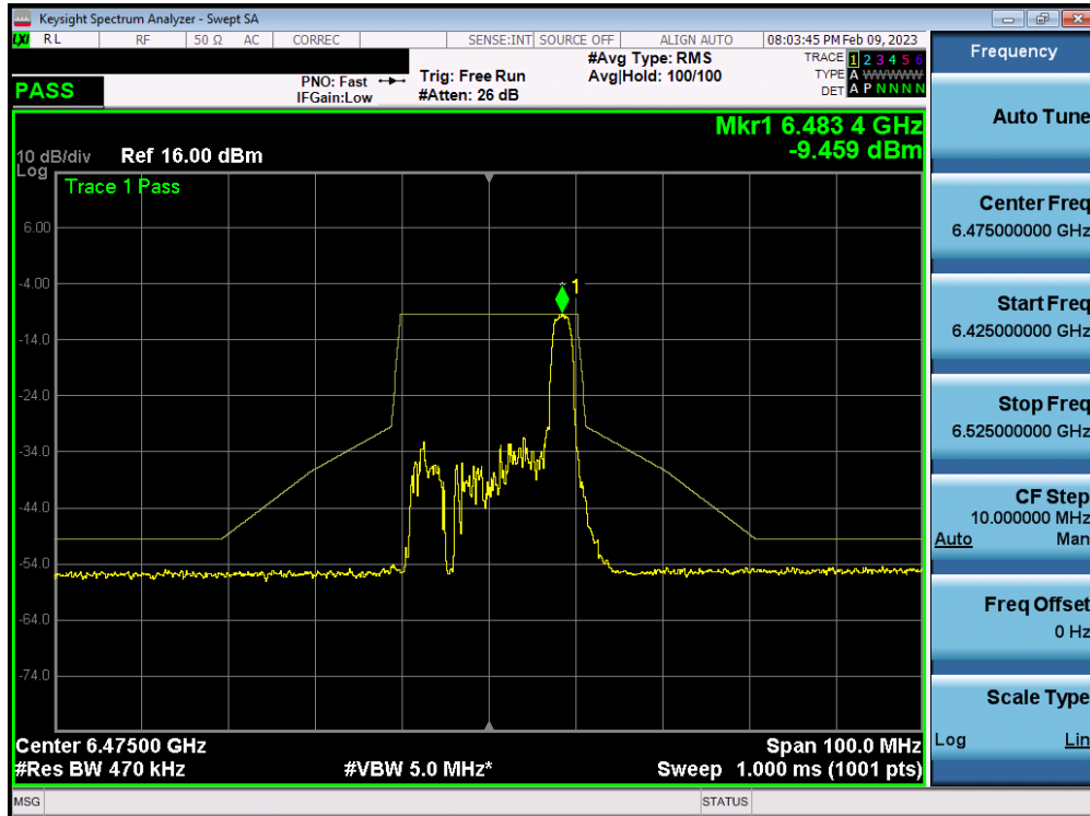
Plot 7-414. In-Band Emission Plot MIMO ANT2 (20MHz BW 802.11ax (26 Tones) (UNII Band 6) – Ch. 105)
