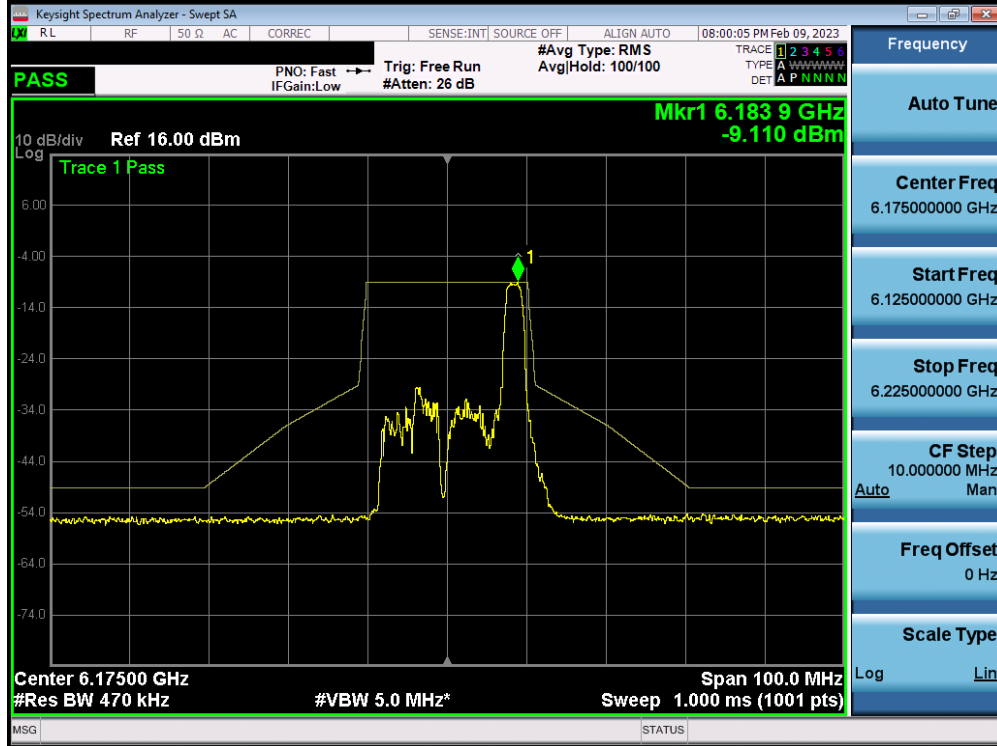
Plot 7-402. In-Band Emission Plot MIMO ANT2 (20MHz BW 802.11ax (26 Tones) (UNII Band 5) – Ch. 45)
