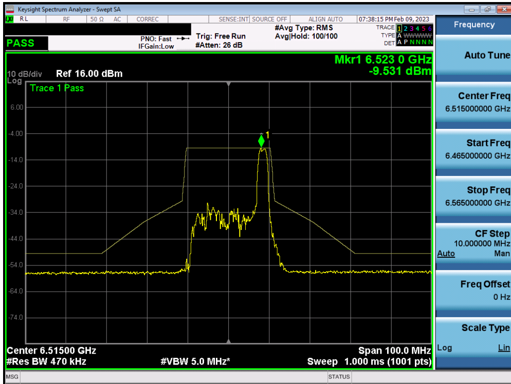
Plot 7-335. In-Band Emission Plot MIMO ANT1 (20MHz BW 802.11ax (26 Tones) (UNII Band 6) – Ch. 113)
