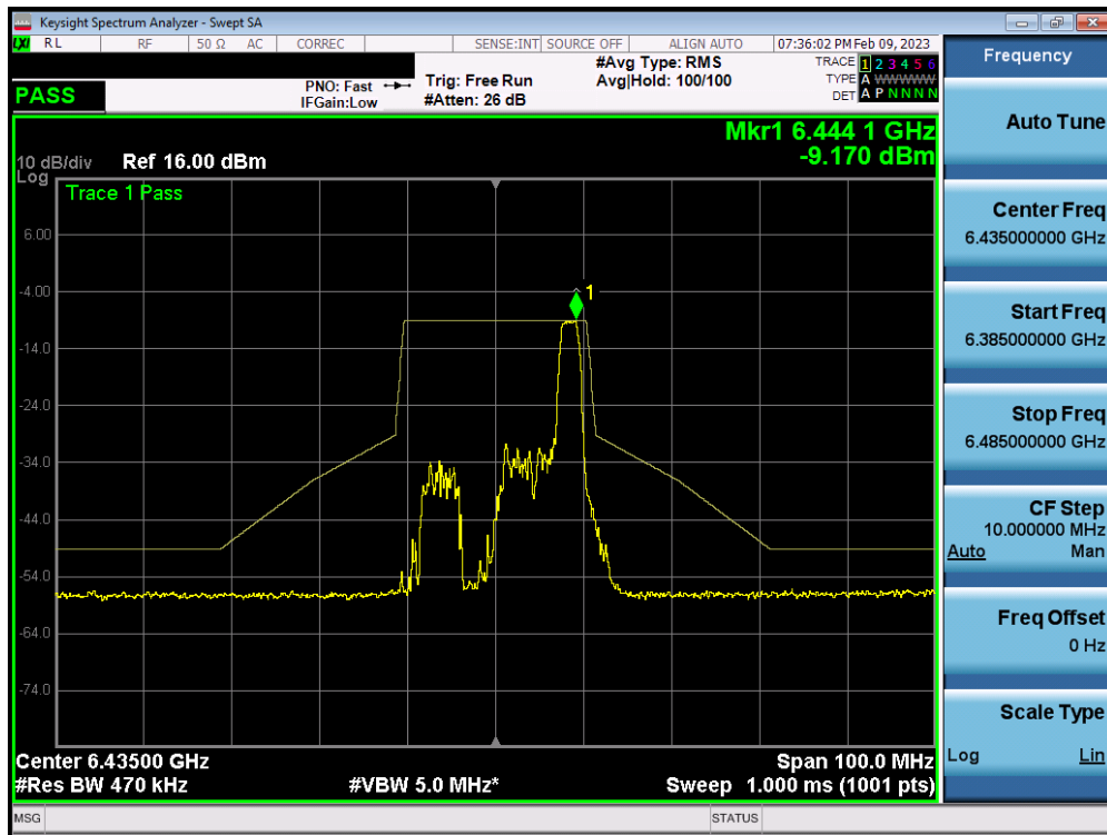
Plot 7-333. In-Band Emission Plot MIMO ANT1 (20MHz BW 802.11ax (26 Tones) (UNII Band 6) – Ch. 97)
