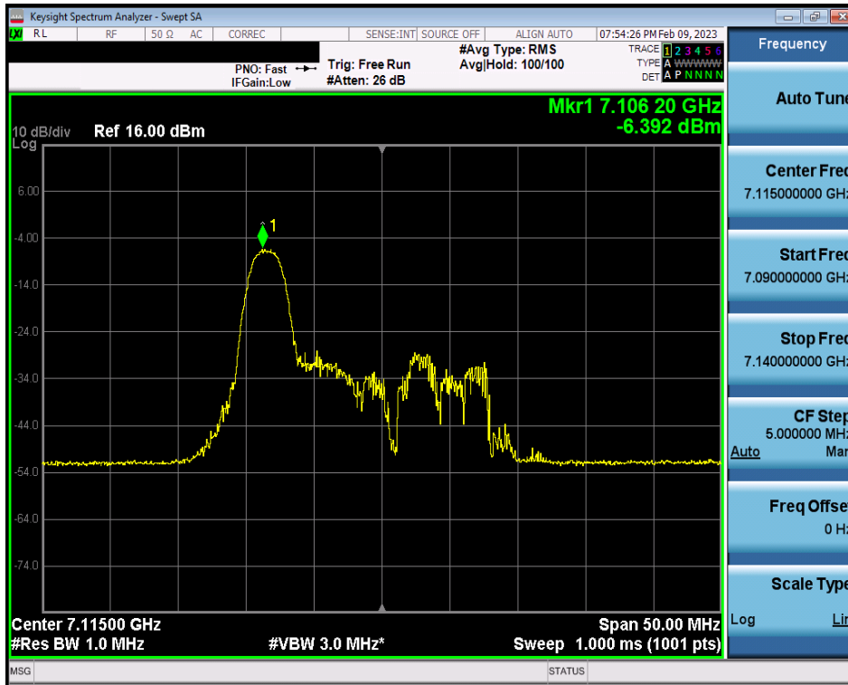
Plot 7-274. Power Spectral Density Plot MIMO ANT2 (20MHz BW 802.11ax (26 Tones) (UNII Band 8) – Ch. 233)
