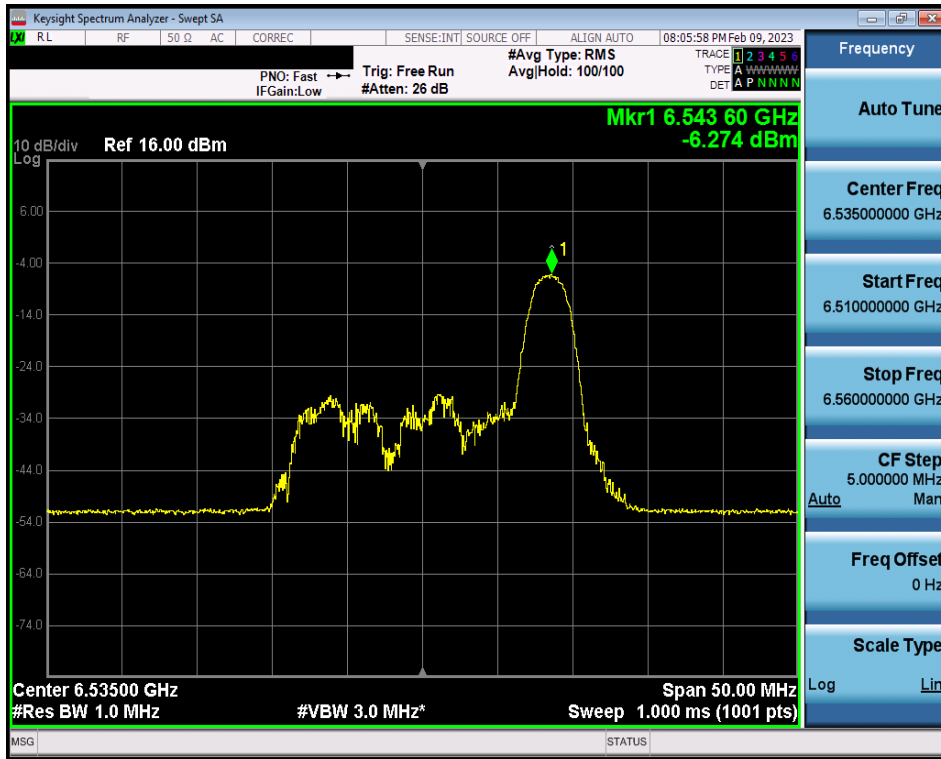
Plot 7-261. Power Spectral Density Plot MIMO ANT2 (20MHz BW 802.11ax (26 Tones) (UNII Band 7) – Ch. 117)
