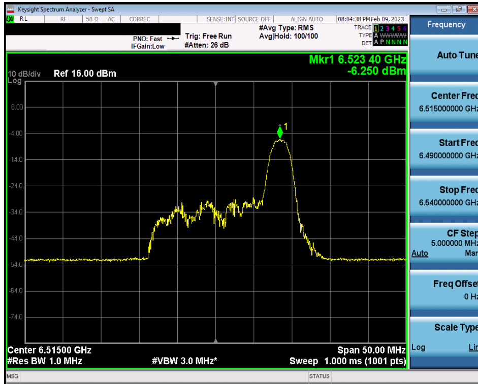
Plot 7-255. Power Spectral Density Plot MIMO ANT2 (20MHz BW 802.11ax (26 Tones) (UNII Band 6) – Ch. 113)
