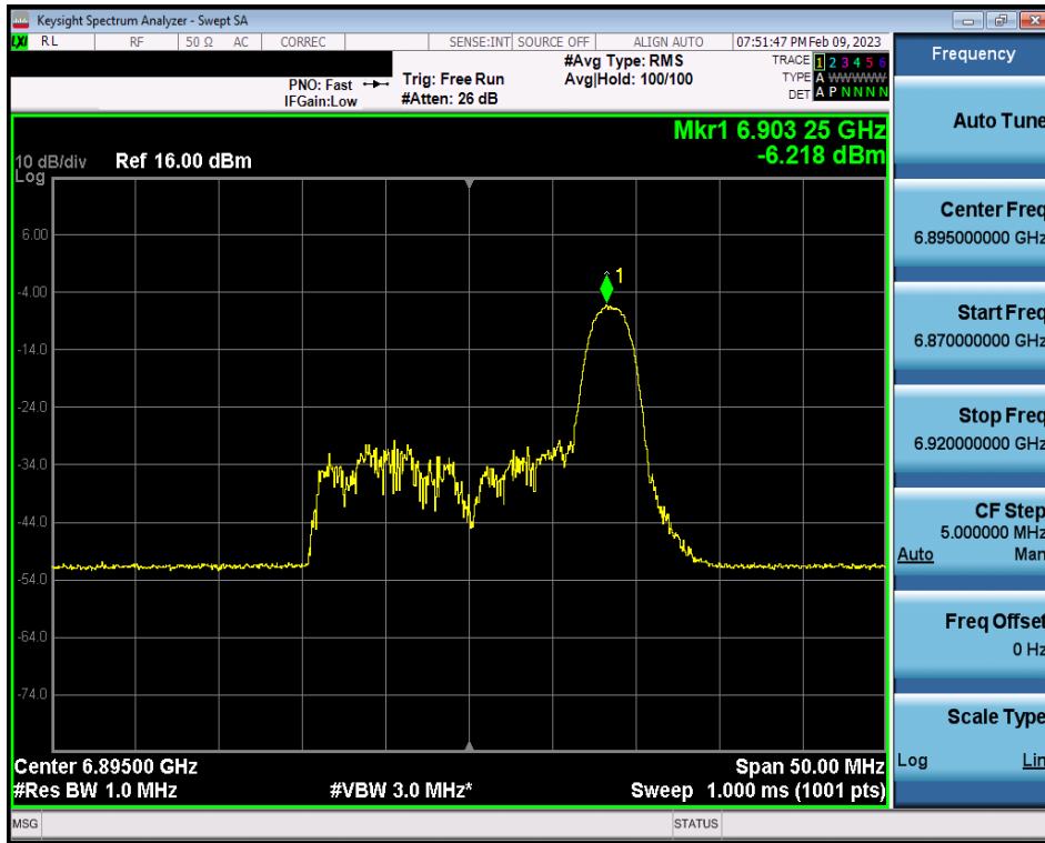
Plot 7-272. Power Spectral Density Plot MIMO ANT2 (20MHz BW 802.11ax (26 Tones) (UNII Band 8) – Ch. 189)
