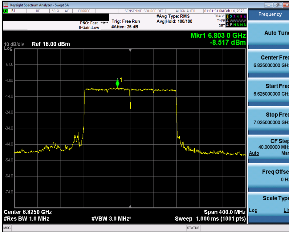
Plot 7-311. Power Spectral Density Plot MIMO ANT2 (160MHz BW 802.11ax (Full Tone) (UNII Band 7) – Ch. 175)
