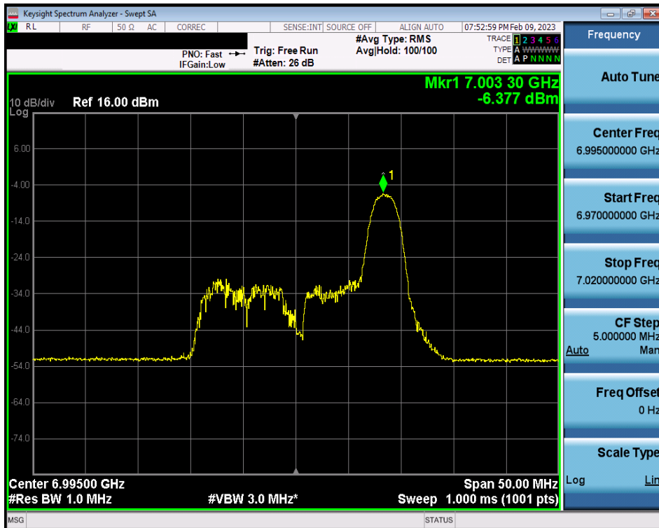
Plot 7-273. Power Spectral Density Plot MIMO ANT2 (20MHz BW 802.11ax (26 Tones) (UNII Band 8) – Ch. 209)
