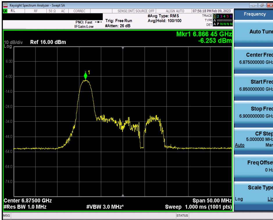
Plot 7-263. Power Spectral Density Plot MIMO ANT2 (20MHz BW 802.11ax (26 Tones) (UNII Band 7) – Ch. 185)
