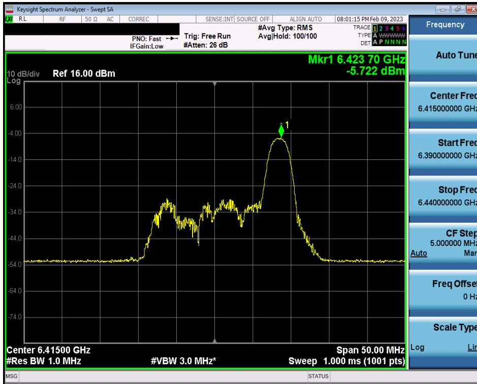
Plot 7-243. Power Spectral Density Plot MIMO ANT2 (20MHz BW 802.11ax (26 Tones) UNII Band 5) – Ch. 93)
