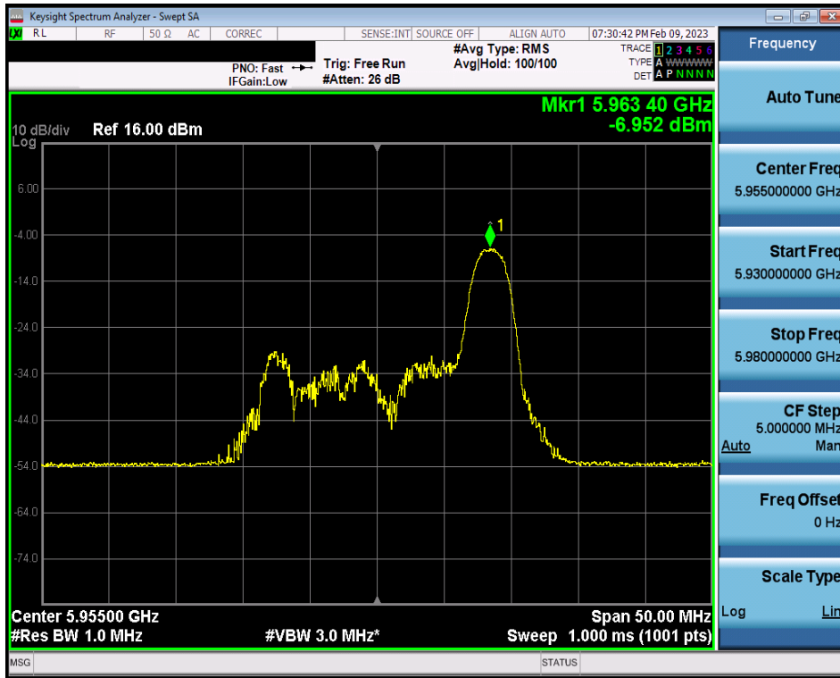
Plot 7-161. Power Spectral Density Plot MIMO ANT1 (20MHz BW 802.11ax (26 Tones) UNII Band 5) – Ch. 1
