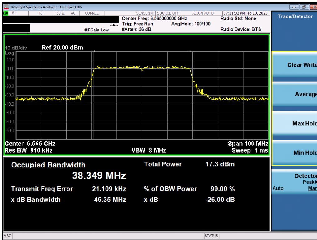
Plot 7-144. Occupied Bandwidth Plot MIMO ANT2 (40MHz BW 802.11ax (Full Tone) (UNII Band 7) – Ch. 123)
