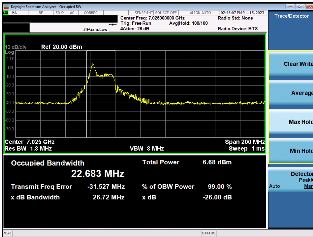
Plot 7-119. Occupied Bandwidth Plot MIMO ANT2 (80MHz BW 802.11ax (26 Tones) (UNII Band 8) – Ch. 215)
