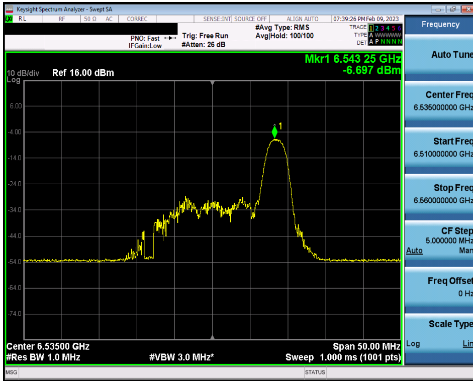
Plot 7-181. Power Spectral Density Plot MIMO ANT1 (20MHz BW 802.11ax (26 Tones) (UNII Band 7) – Ch. 117)
