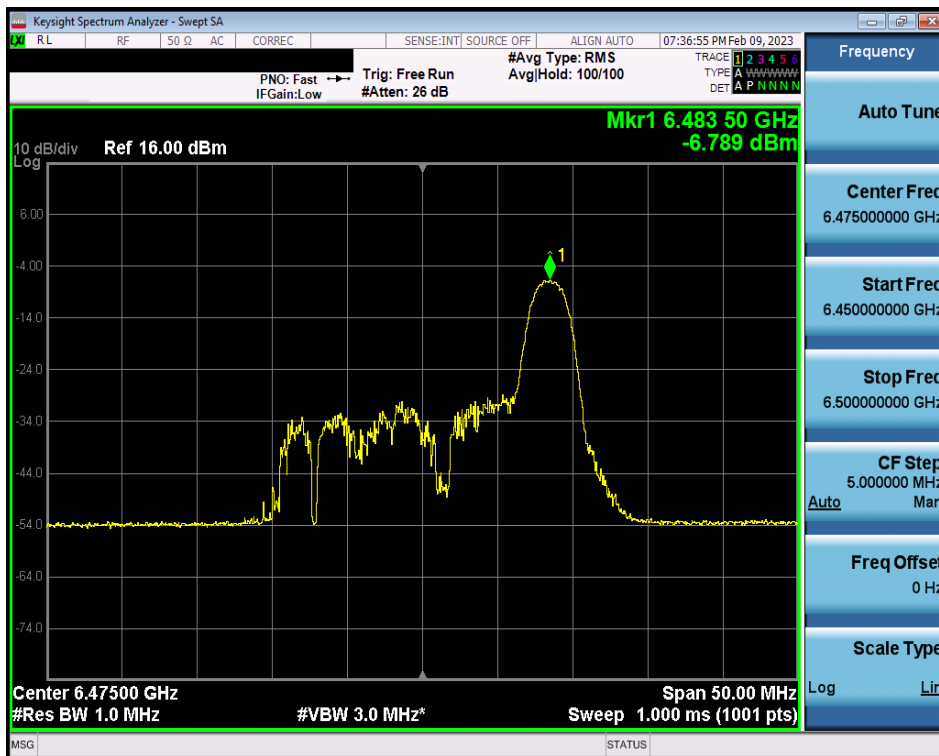
Plot 7-174. Power Spectral Density Plot MIMO ANT1 (20MHz BW 802.11ax (26 Tones) (UNII Band 6) – Ch. 105)
