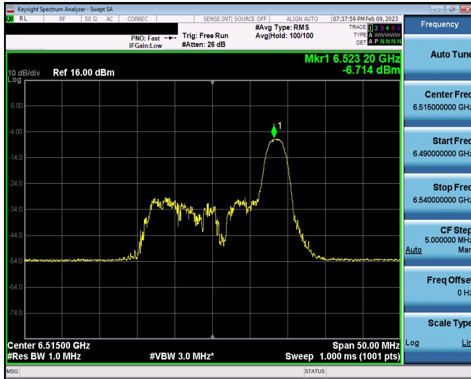
Plot 7-175. Power Spectral Density Plot MIMO ANT1 (20MHz BW 802.11ax (26 Tones) (UNII Band 6) – Ch. 113)
