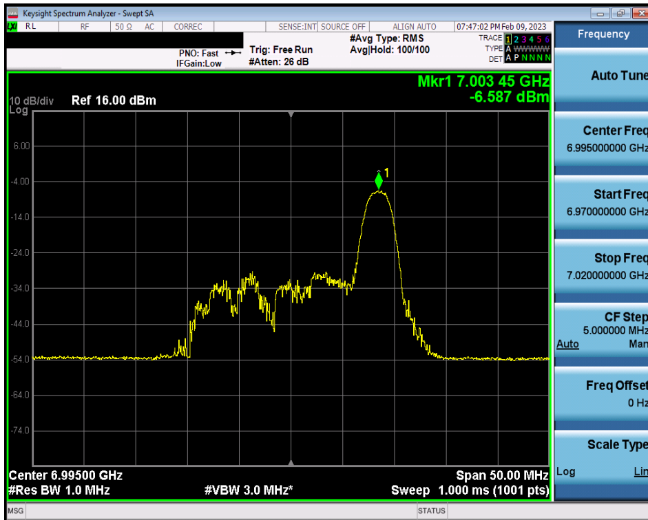
Plot 7-193. Power Spectral Density Plot MIMO ANT1 (20MHz BW 802.11ax (26 Tones) (UNII Band 8) – Ch. 209)
