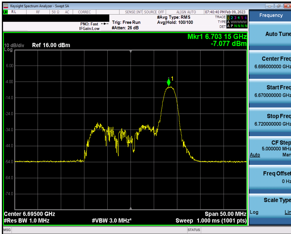
Plot 7-182. Power Spectral Density Plot MIMO ANT1 (20MHz BW 802.11ax (26 Tones) (UNII Band 7) – Ch. 149)
