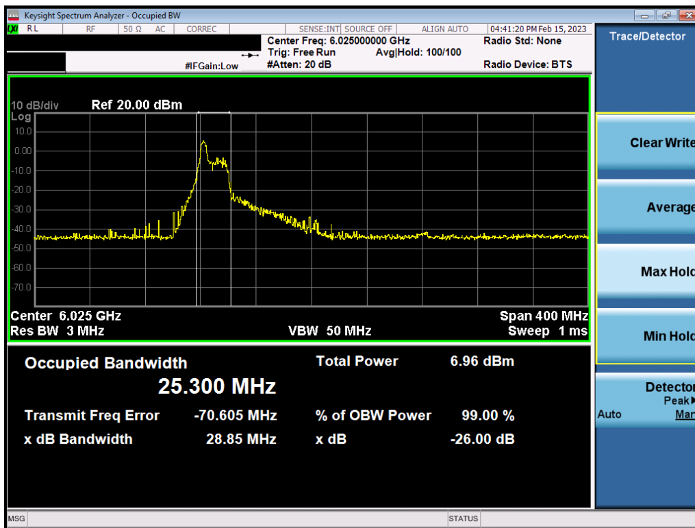
Plot 7-90. Occupied Bandwidth Plot MIMO ANT2 (160MHz BW 802.11ax (26 Tones) (UNII Band 5) – Ch. 15)
