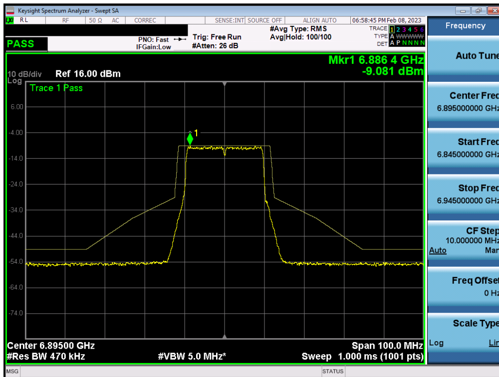
Plot 7-304. In-Band Emission Plot Measurement MIMO ANT2 (20MHz 802.11ax (UNII Band 8) – Ch. 189)
