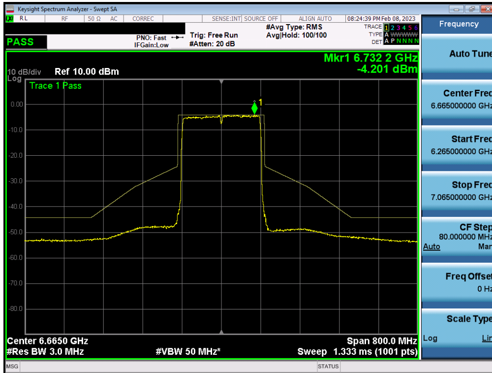
Plot 7-247. In-Band Emission Plot Measurement MIMO ANT1 (160MHz 802.11ax (UNII Band 7) – Ch. 143)
