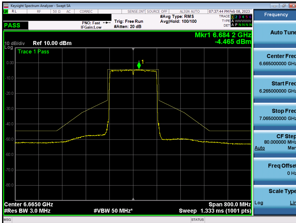
Plot 7-299. In-Band Emission Plot Measurement MIMO ANT2 (160MHz 802.11ax (UNII Band 7) – Ch. 143)
