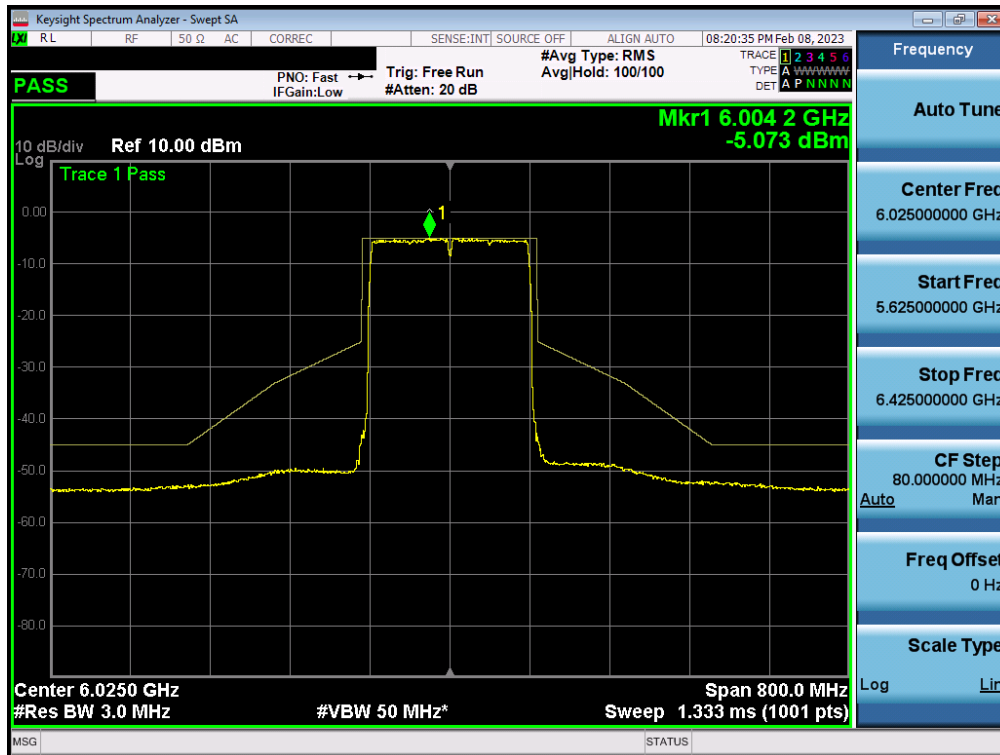
Plot 7-221. In-Band Emission Plot Measurement MIMO ANT1 (160MHz 802.11ax (UNII Band 5) – Ch. 15)
