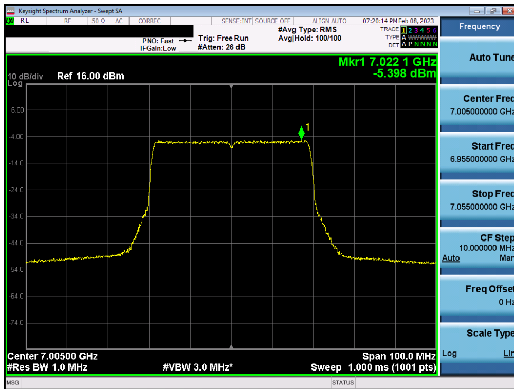
Plot 7-204. Power Spectral Density Measurement MIMO ANT2 (40MHz 802.11ax (UNII Band 8) – Ch. 211)
