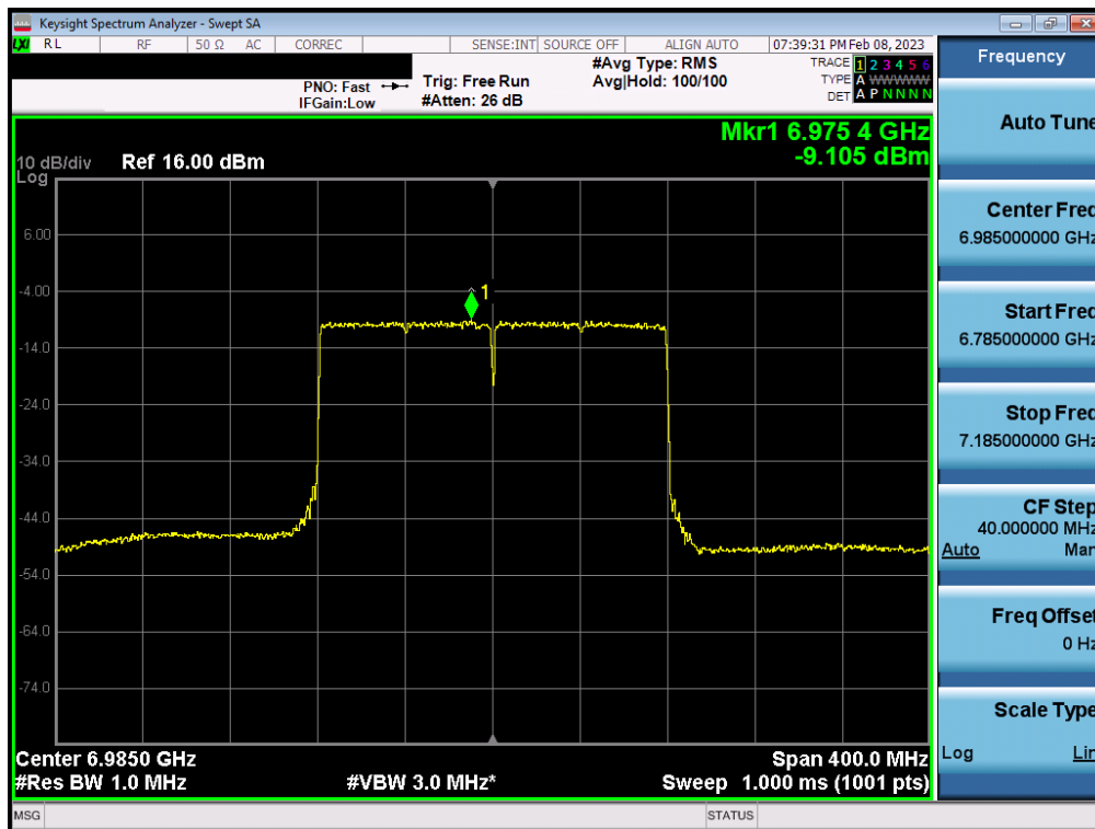
Plot 7-208. Power Spectral Density Measurement MIMO ANT2 (160MHz 802.11ax (UNII Band 8) – Ch. 207)
