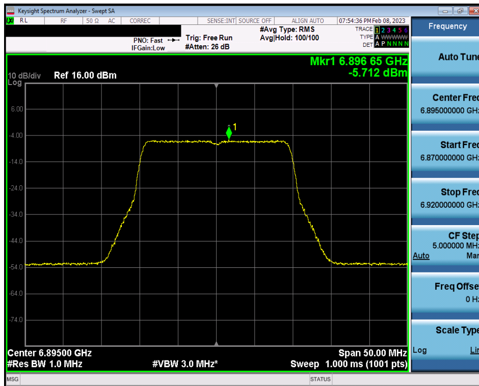
Plot 7-148. Power Spectral Density Measurement MIMO ANT1 (20MHz 802.11ax (UNII Band 8) – Ch. 189)
