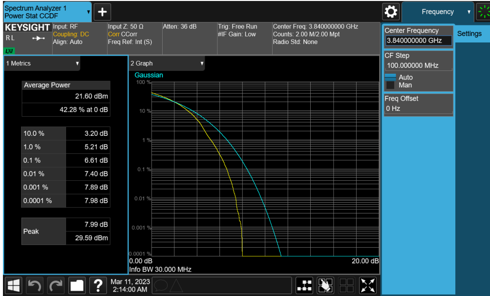
Plot 7-333. PAR Plot (NR Band n77 PC2 (C-band) - 30MHz CP-OFDM 256-QAM - Full RB - Sub-UHB)
