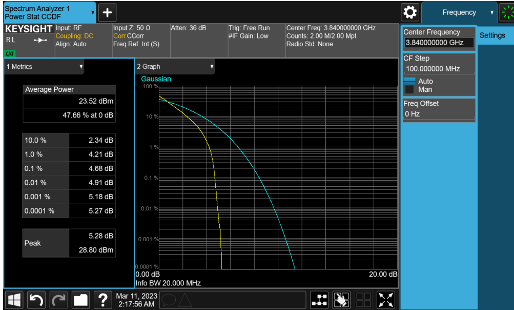
Plot 7-335. PAR Plot (NR Band n77 PC2 (C-band) - 20MHz CP-OFDM QPSK - Full RB - Sub-UHB)
