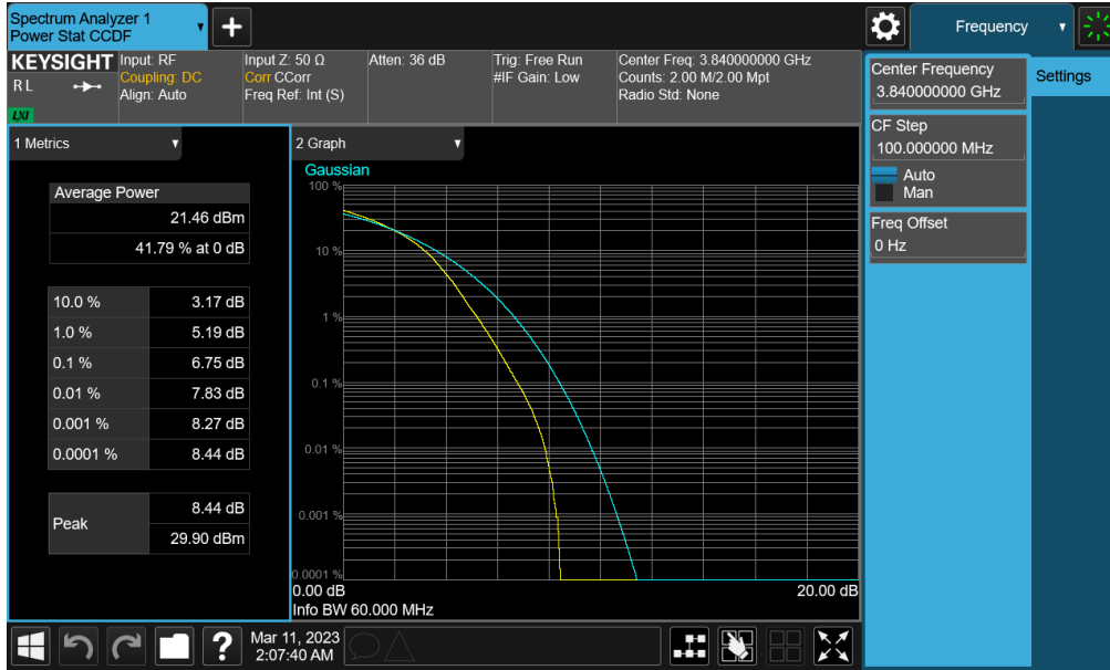
Plot 7-327. PAR Plot (NR Band n77 PC2 (C-band) - 60MHz CP-OFDM 256-QAM - Full RB - Sub-UHB)
