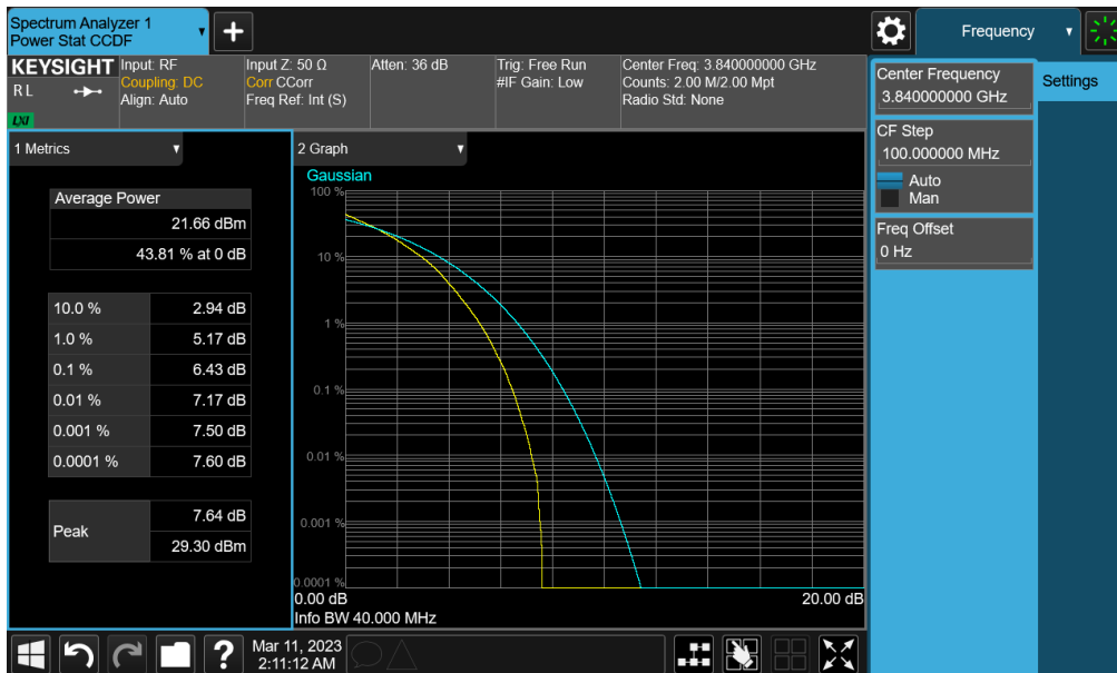
Plot 7-330. PAR Plot (NR Band n77 PC2 (C-band) - 40MHz CP-OFDM 256-QAM - Full RB - Sub-UHB)
