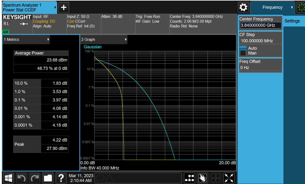
Plot 7-329. PAR Plot (NR Band n77 PC2 (C-band) - 40MHz CP-OFDM QPSK - Full RB - Sub-UHB)
