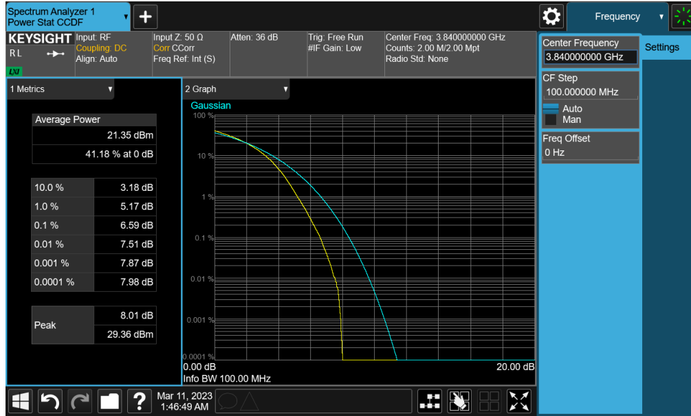
Plot 7-321. PAR Plot (NR Band n77 PC2 (C-band) - 100MHz CP-OFDM 256-QAM - Full RB - Sub-UHB)
