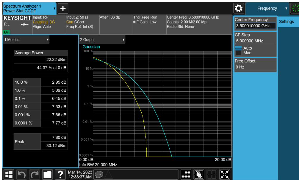
Plot 7-300. PAR Plot (NR Band n77 PC2 (DoD) - 20MHz CP-OFDM 256-QAM - Full RB - Sub-UHB)
