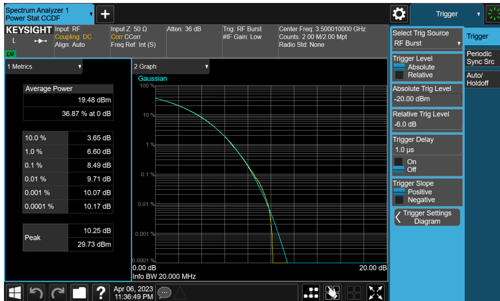
Plot 7-282. PAR Plot (NR Band n77 PC2 (DoD) - 20MHz CP-OFDM 256-QAM - Full RB - Main1)
