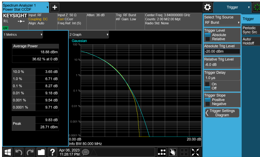
Plot 7-306. PAR Plot (NR Band n77 PC2 (C-band) - 80MHz CP-OFDM 256-QAM - Full RB - Main1)
