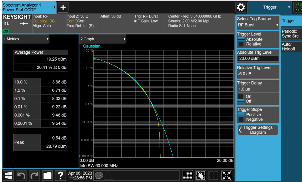
Plot 7-309. PAR Plot (NR Band n77 PC2 (C-band) - 60MHz CP-OFDM 256-QAM - Full RB - Main1)
