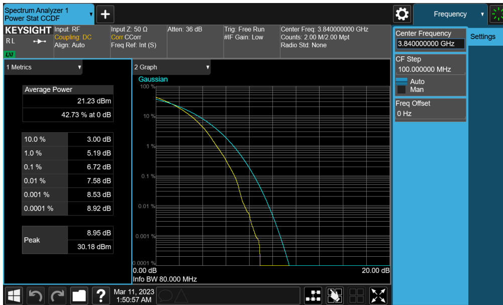
Plot 7-324. PAR Plot (NR Band n77 PC2 (C-band) - 80MHz CP-OFDM 256-QAM - Full RB - Sub-UHB)
