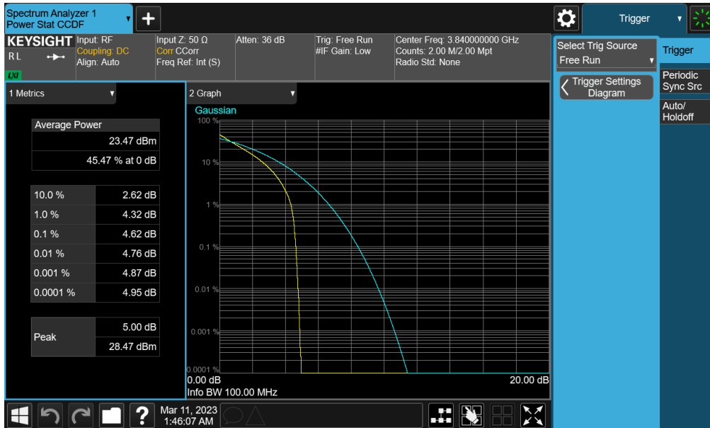
Plot 7-320. PAR Plot (NR Band n77 PC2 (C-band) - 100MHz CP-OFDM QPSK - Full RB - Sub-UHB)
