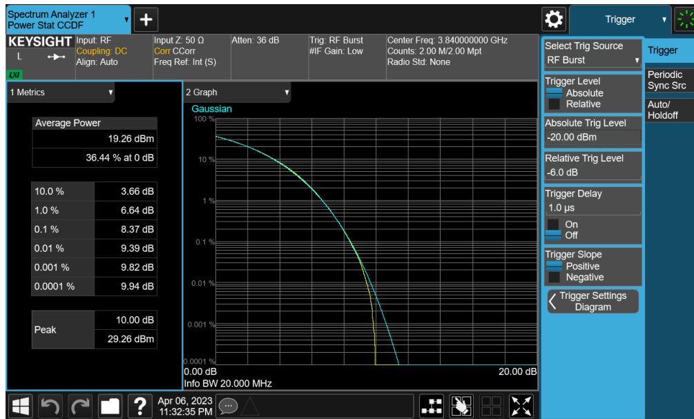
Plot 7-318. PAR Plot (NR Band n77 PC2 (C-band) - 20MHz CP-OFDM 256-QAM - Full RB - Main1)
