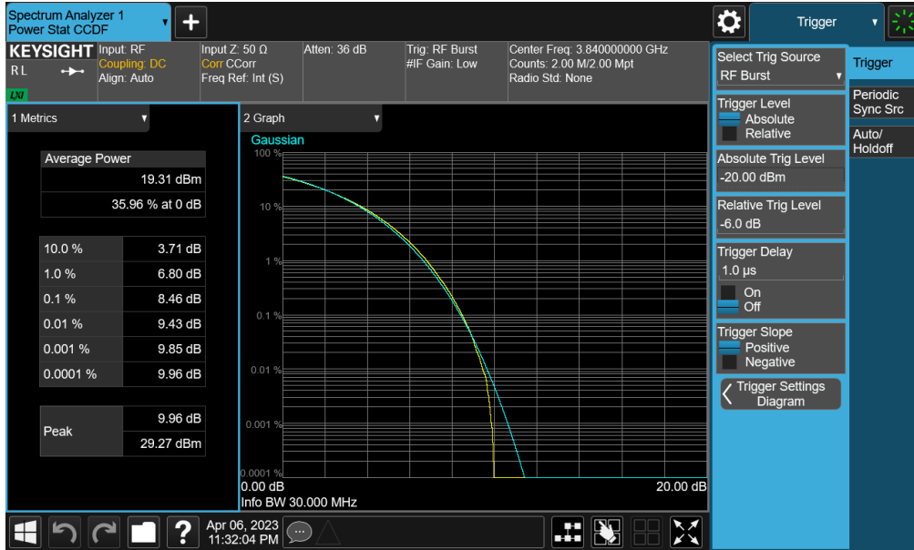
Plot 7-315. PAR Plot (NR Band n77 PC2 (C-band) - 30MHz CP-OFDM 256-QAM - Full RB - Main1)
