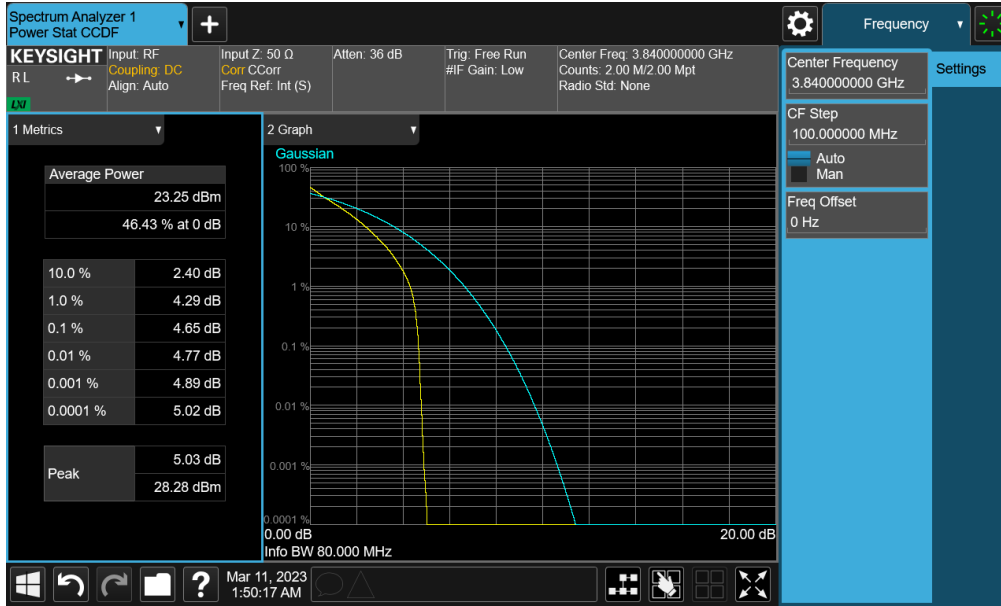
Plot 7-323. PAR Plot (NR Band n77 PC2 (C-band) - 80MHz CP-OFDM QPSK - Full RB - Sub-UHB)
