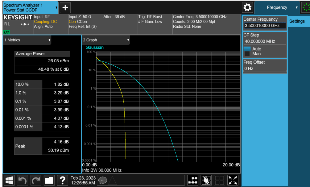
Plot 7-277. PAR Plot (NR Band n77 PC2 (DoD) - 30MHz DFT-s-OFDM BPSK - Full RB - Main1)
