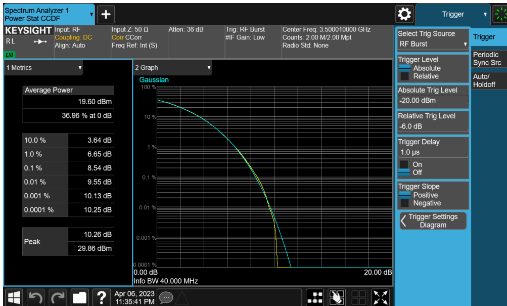
Plot 7-276. PAR Plot (NR Band n77 PC2 (DoD) - 40MHz CP-OFDM 256-QAM - Full RB - Main1)
