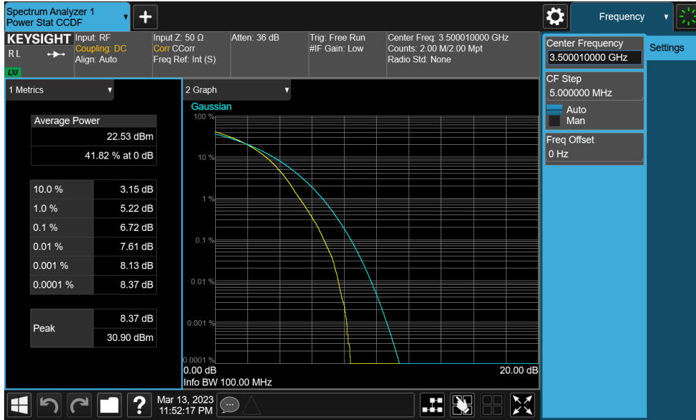
Plot 7-285. PAR Plot (NR Band n77 PC2 (DoD) - 100MHz CP-OFDM 256-QAM - Full RB - Sub-UHB)
