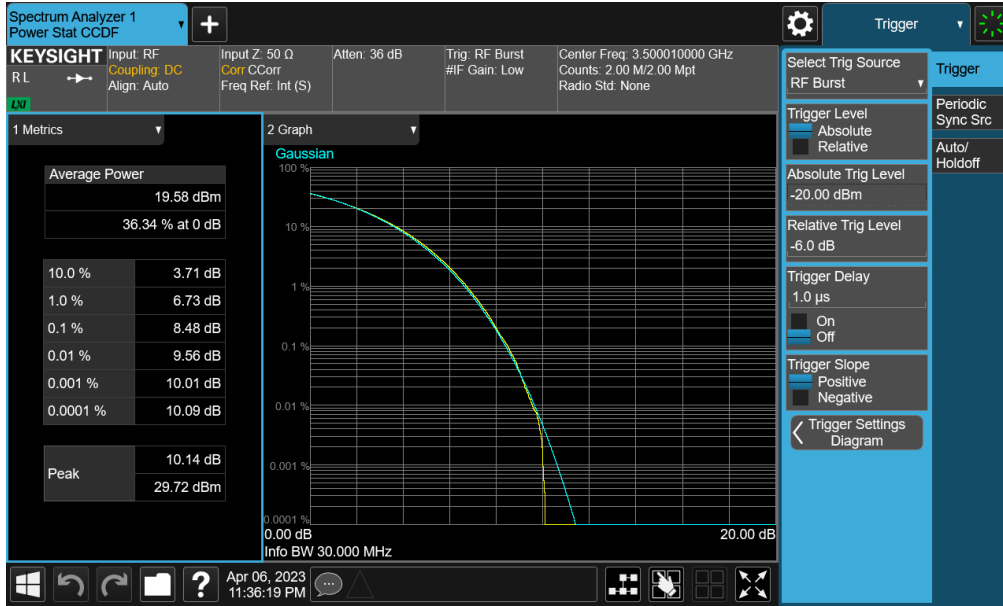
Plot 7-279. PAR Plot (NR Band n77 PC2 (DoD) - 30MHz CP-OFDM 256-QAM - Full RB - Main1)
