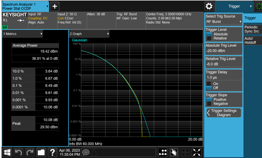
Plot 7-273. PAR Plot (NR Band n77 PC2 (DoD) - 60MHz CP-OFDM 256-QAM - Full RB - Main1)
