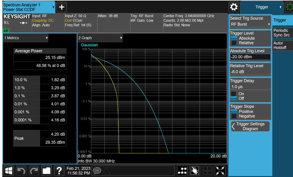
Plot 7-313. PAR Plot (NR Band n77 PC2 (C-band) - 30MHz DFT-s-OFDM BPSK - Full RB - Main1)
