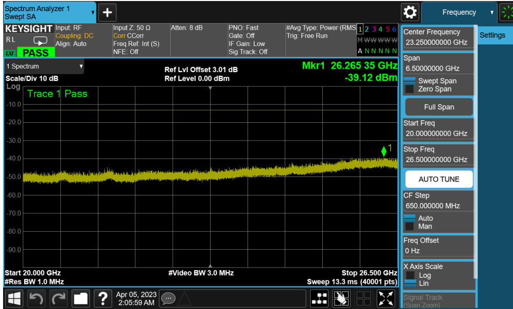
Plot 7-111. Conducted Spurious Plot (NR Band n77 PC3 (C-band) - 100MHz QPSK - 1RB - Low Channel - Main1 (UL-MIMO))
