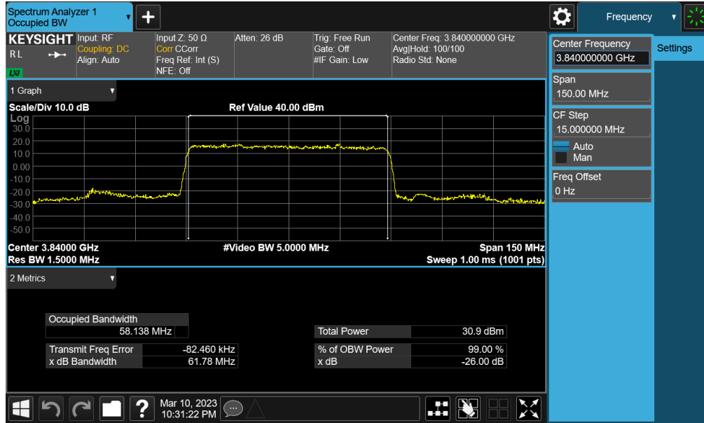
Plot 7-77. Occupied Bandwidth Plot (NR Band n77 PC2 (C-band) - 60MHz \pi/2 BPSK - Full RB - Sub-UHB)
