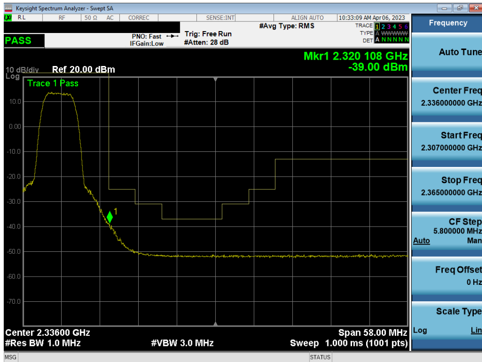
Plot 7-201. Extended Upper Band Edge Plot (NR Band n30 - 5MHz CP-OFDM-QPSK – Full RB - Main2)
