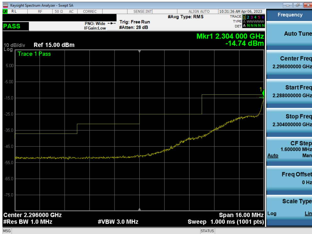
Plot 7-199. Extended Lower Band Edge Plot (NR Band n30 - 5MHz CP-OFDM-QPSK – Full RB - Main2)
