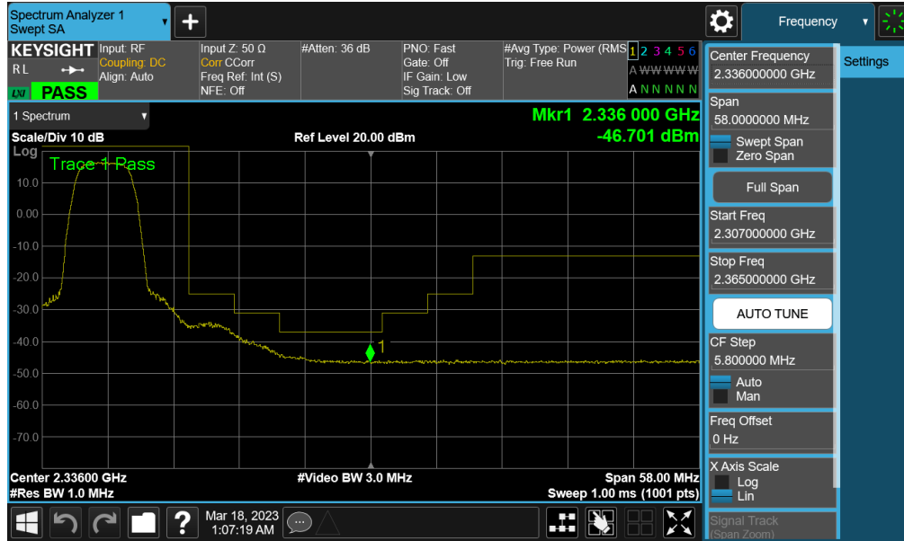
Plot 7-145. Extended Upper Band Edge Plot (LTE Band 30 - 5MHz QPSK – Full RB - Main2)
