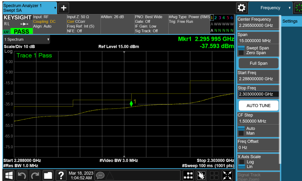
Plot 7-143. Extended Lower Band Edge Plot Integration Below 2303MHz (LTE Band 30 - 5MHz QPSK – Full RB - Main2)
