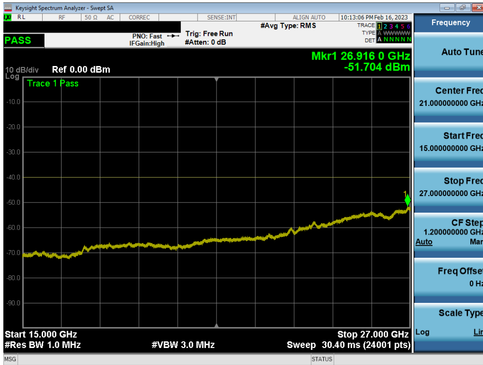
Plot 7-49. Conducted Spurious Plot (LTE Band 30 - 10MHz QPSK - 1RB - Main2)
