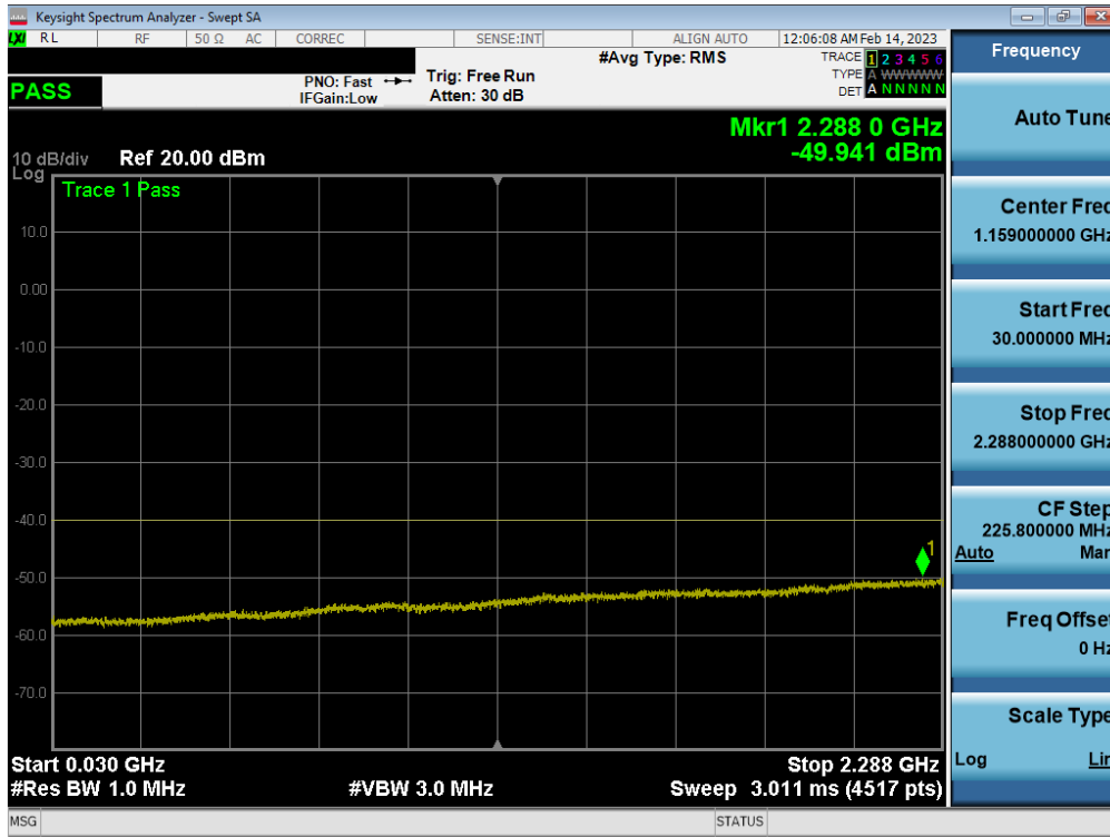
Plot 7-47. Conducted Spurious Plot (LTE Band 30 - 10MHz QPSK - 1RB - Main2)
