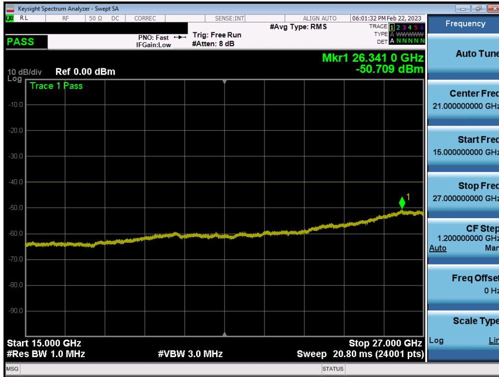
Plot 7-61. Conducted Spurious Plot (NR Band n30 - 10MHz QPSK - RB Size 1 – Main2)
