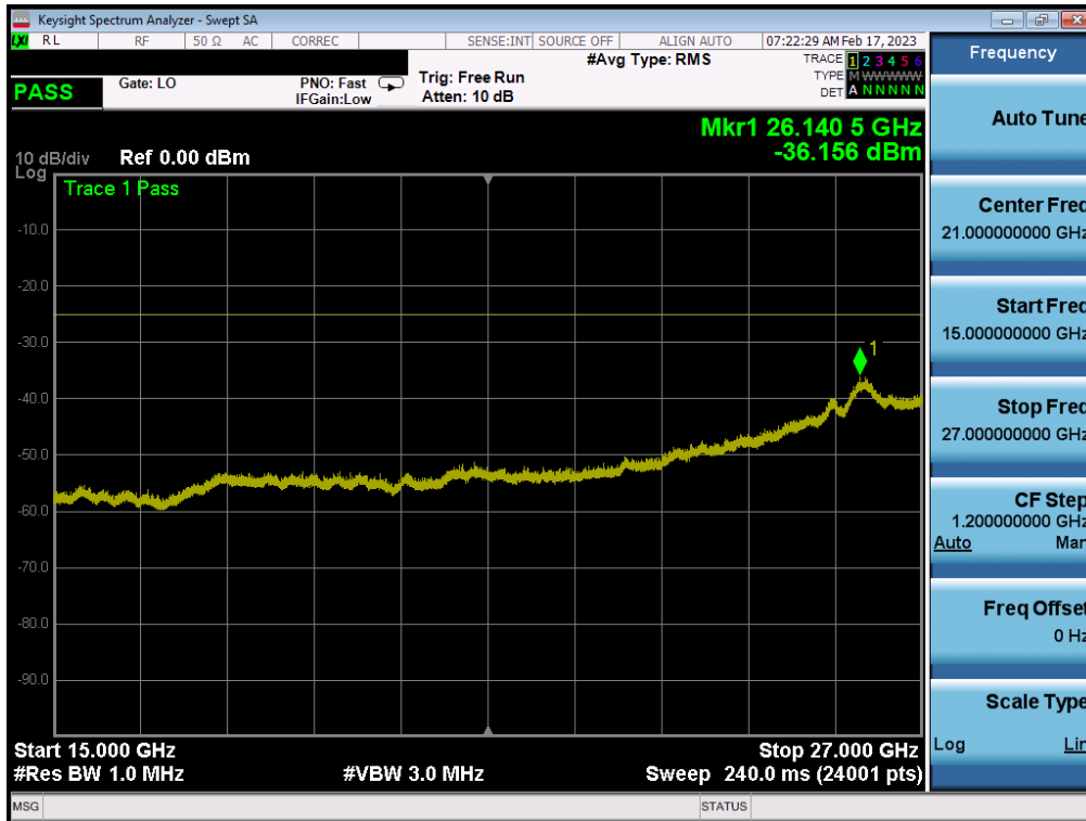
Plot 7-55. Conducted Spurious Plot (LTE Band 41(PC3) - 20MHz QPSK - 1RB - Mid Channel - Main2)
