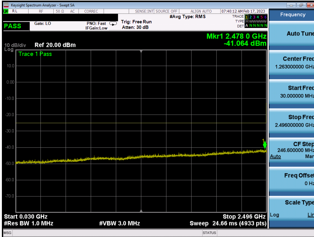
Plot 7-56. Conducted Spurious Plot (LTE Band 41(PC3) - 20MHz QPSK - 1RB - High Channel - Main2)
