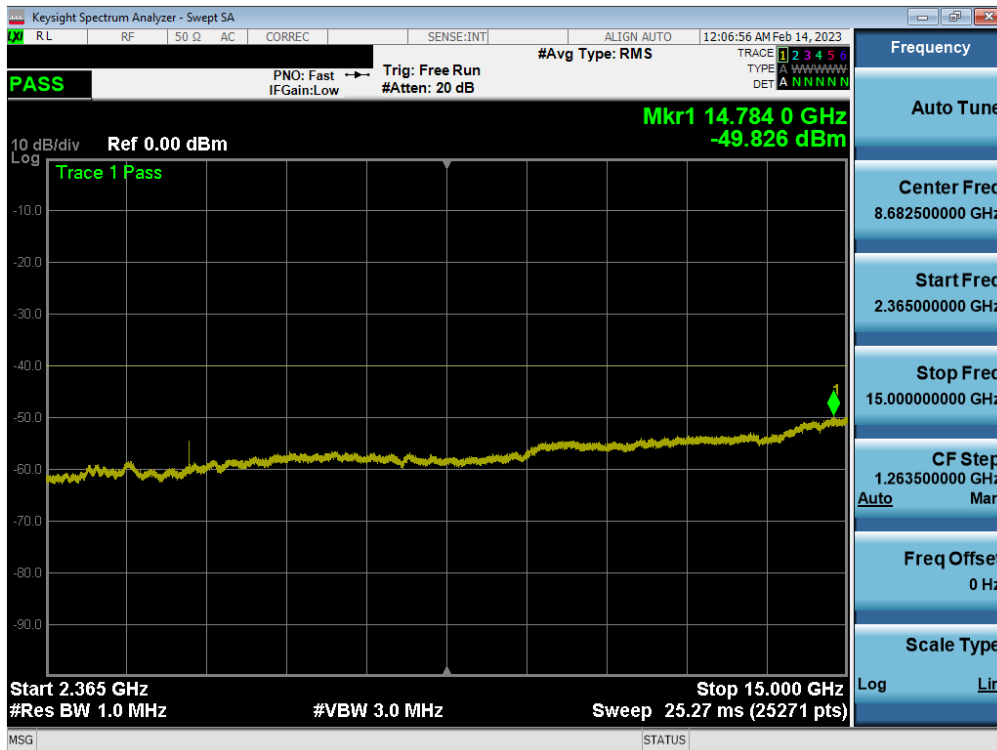
Plot 7-48. Conducted Spurious Plot (LTE Band 30 - 10MHz QPSK - 1RB - Main2)
