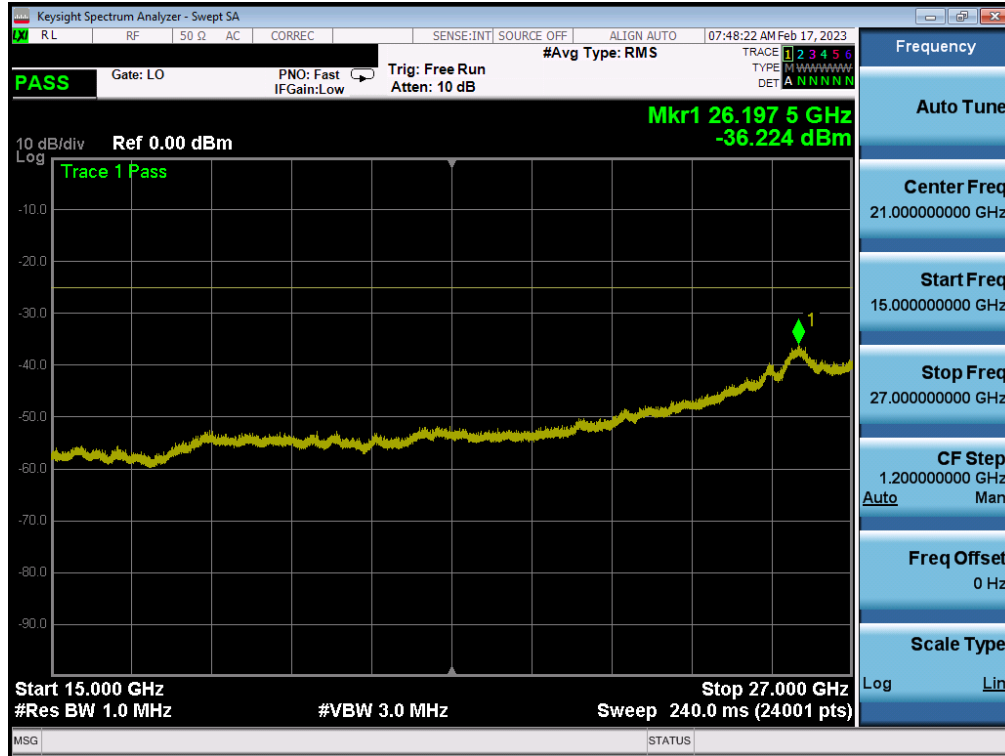
Plot 7-58. Conducted Spurious Plot (LTE Band 41(PC3) - 20MHz QPSK - 1RB - High Channel - Main2)
