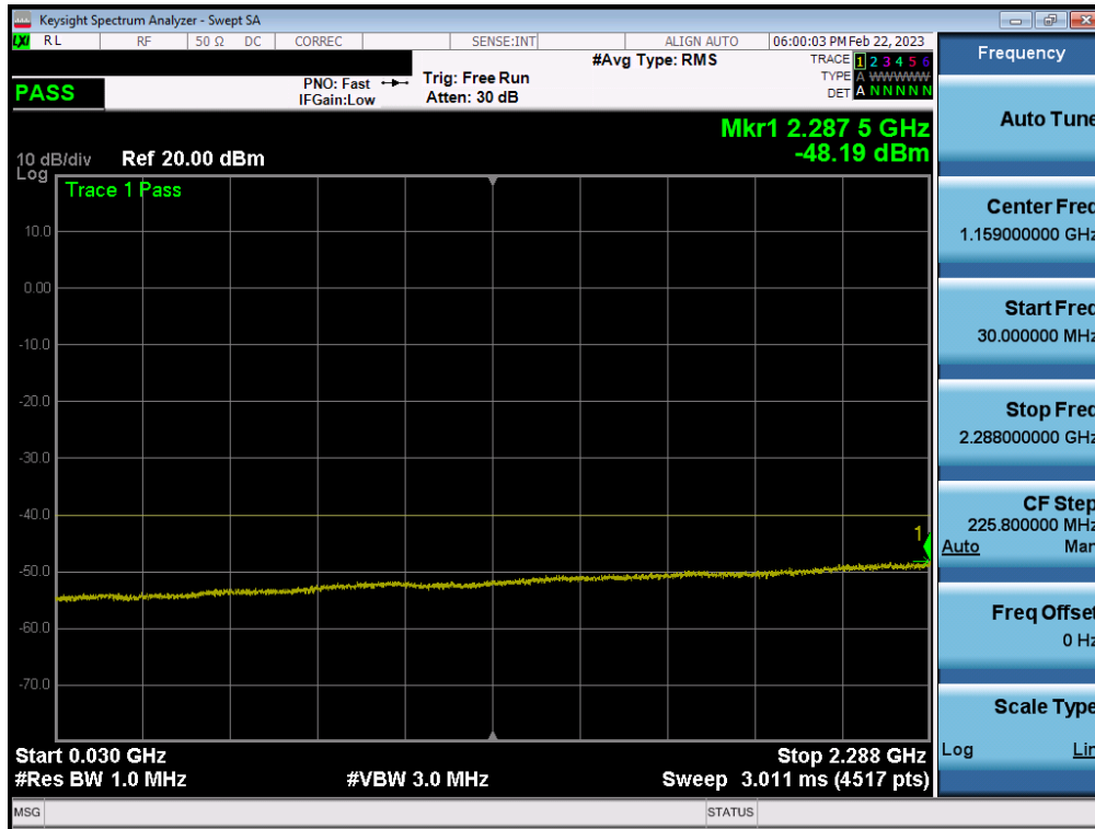
Plot 7-59. Conducted Spurious Plot (NR Band n30 - 10MHz QPSK - 1RB – Main2)
