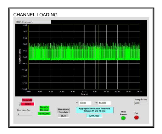
The level of traffic loading on the channel by the EUT is 22.1%
