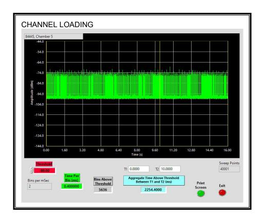
The level of traffic loading on the channel by the EUT is 22.5%
