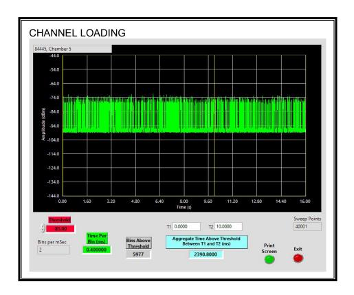
The level of traffic loading on the channel by the EUT is 23.9%
