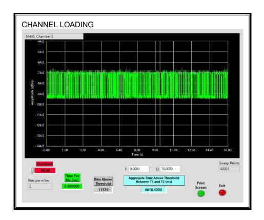
The level of traffic loading on the channel by the EUT is 46.1%
