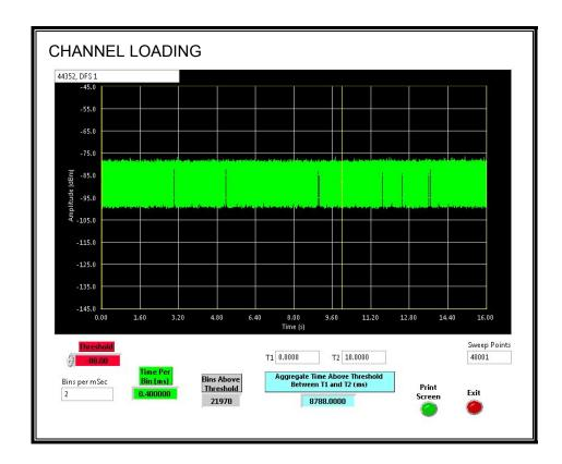
The level of traffic loading on the channel by the EUT is 87.88%.
