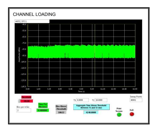
The level of traffic loading on the channel by the EUT is 42.488%.
