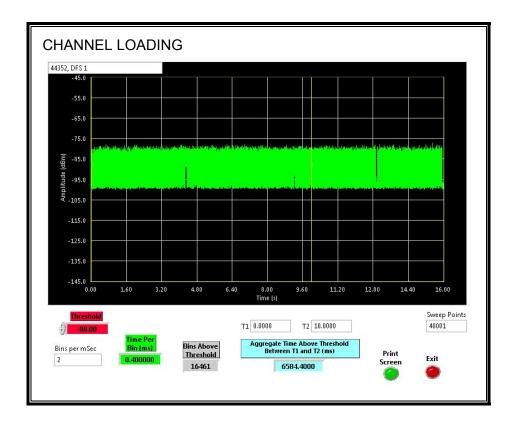
The level of traffic loading on the channel by the EUT is 65.844%
