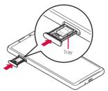
Push the tray into the end, firmly press each point indicated with O, and then make sure that there are no gaps between the terminal and the cover.
