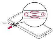
You are recommended to replace the parts for maintaining waterproof/dustproof property once every two years regardless of whether any abnormality is present or not. For replacement of the parts, DOCOMO keeps the terminal at DOCOMO-specified repair office and accept for a fee.
