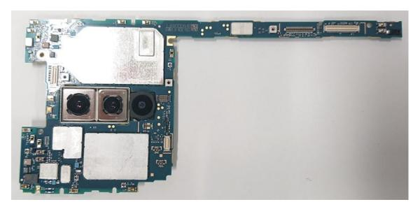
Internal PWB without Shield cases (Rear-side)
