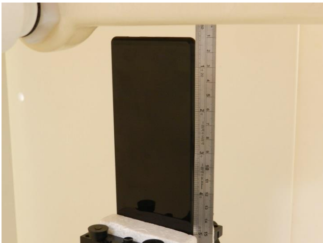
Top Side, Test Separation 10 mm
