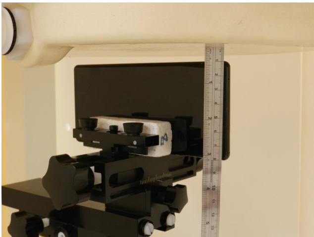
Left Side, Test Separation 10 mm
